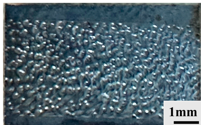
Figure 9. Surface view of 22CrMoH steel after SEBP.
