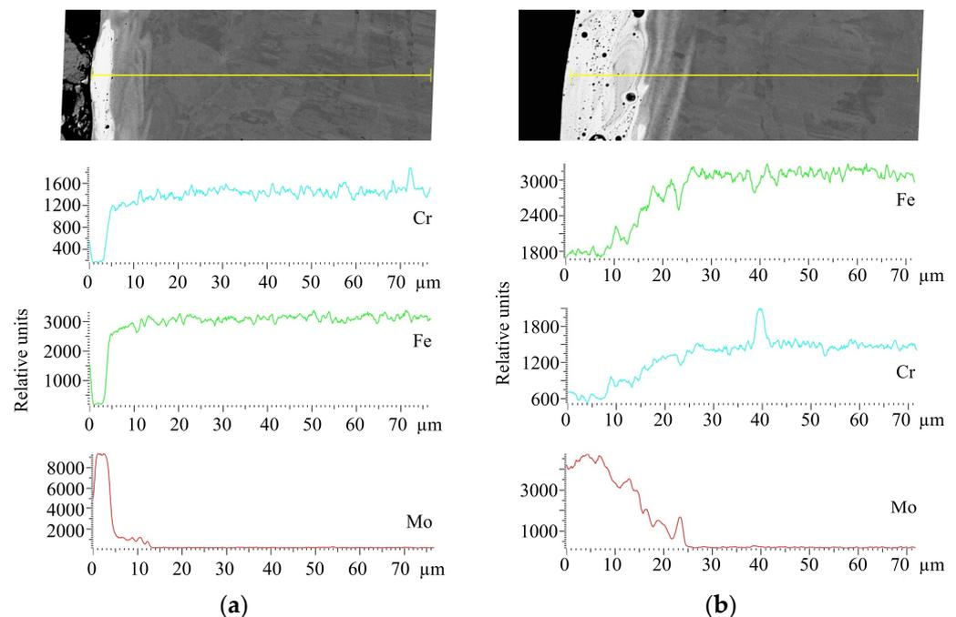
**Figure 6.** Distribution of elements in coatings obtained by ESA technology, which is performed by a Mo-electrode with preliminary application of MoS<sub>2</sub> powder on the surface of AISI 321 steel. The ESA process was performed at discharge energies (Wp): (a)—0.55 J; (b)—3.4 J.
