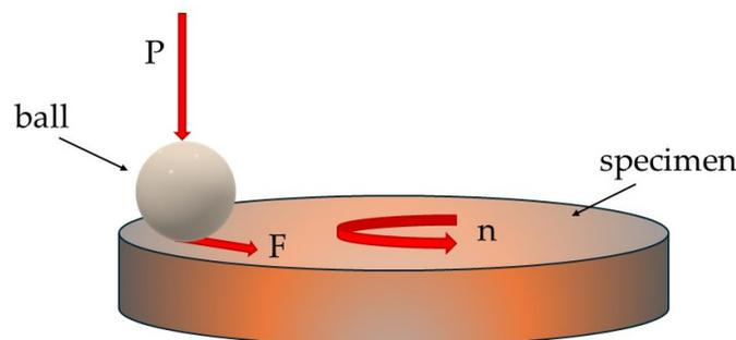
**Figure 3.** Test scheme on the T-21 tribo-tester.
