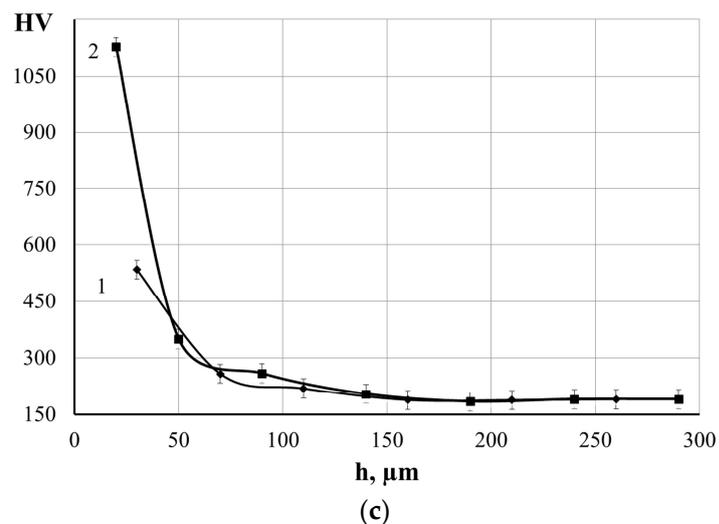
**Figure 4.** Microstructures (a,b) and microhardness distribution (c) in the AISI 321 steel surface layer obtained by ESA technology, which is performed by a Mo-electrode with the preliminary application of MoS<sub>2</sub> powder. The ESA process was performed at discharge energies ( $W_p$ ): (a)—0.55 J; (b)—3.4 J; (c)—on the graph: 1— $W_p = 0.55 \text{ J}$ , 2— $W_p = 3.4 \text{ J}$ .
