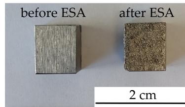
**Figure 1.** Samples before and after electrospark alloying.
