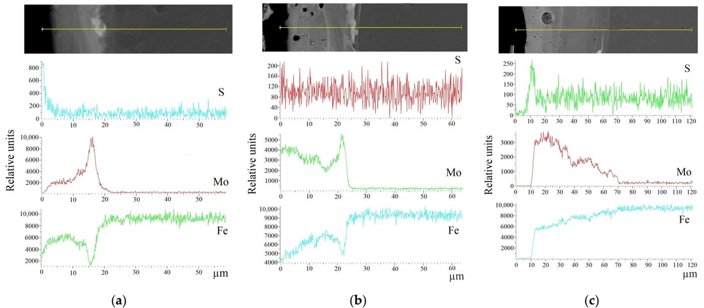
**Figure 9.** Distribution of elements in coatings obtained by ESA technology, which is performed by a Mo-electrode with the use of a sulfur-containing paste, on C40 steel at the ESA discharge energies: (a)—0.13 J; (b)—0.55 J; and (c)—3.4 J.
