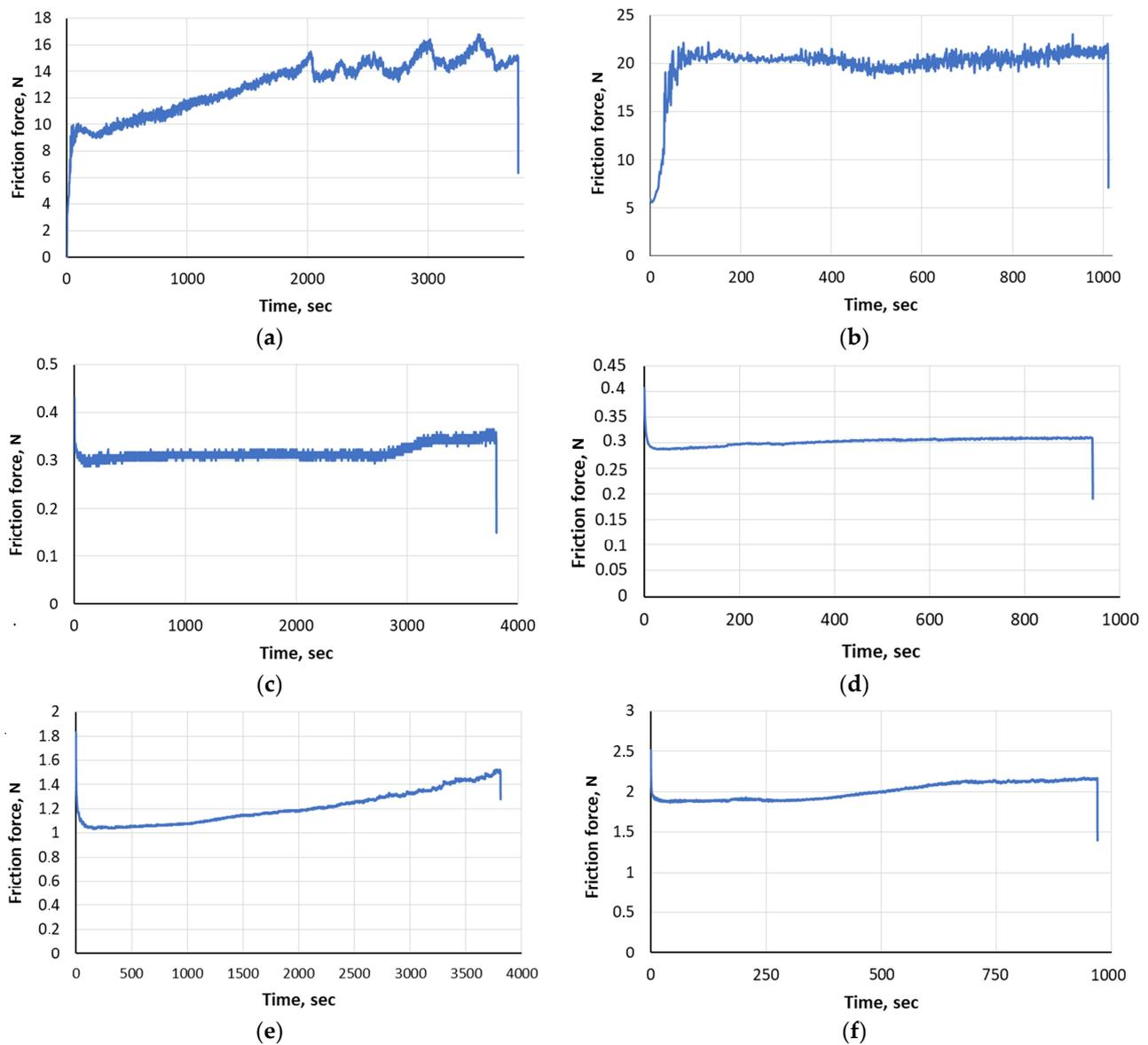
**Figure 10.** The nature of the change in the friction force T (N) of the steel ball over the surface of the test specimen: (a)—Mo coating, P = 20 N, (b)—Mo coating, P = 40 N, (c)—Mo + S coating, P = 20 N, (d)—Mo + S coating, P = 40 N, (e)—Mo+ MoS<sub>2</sub> coating, P = 20 N, (f)—Mo+ MoS<sub>2</sub> coating, P = 40 N.
