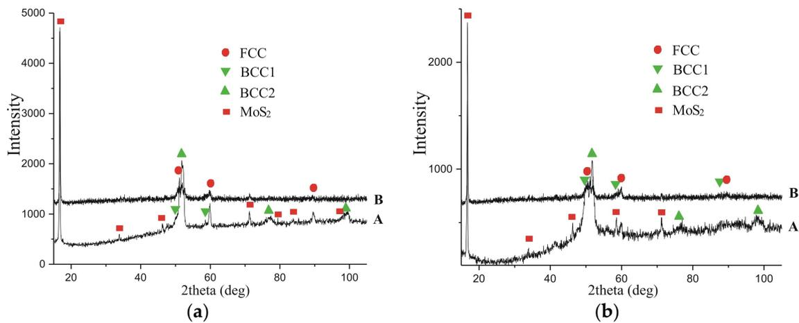
**Figure 7.** Diffractograms of the coatings obtained by the ESA technology, which is performed by a Mo-electrode with preliminary application of MoS<sub>2</sub> powder on the surface of AISI 321 steel: A—surface, B—after polishing 15  $\mu$ m. The ESA process was performed at discharge energies (Wp): (a)—0.55 J; (b)—3.4 J.
