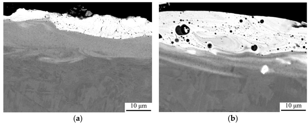
**Figure 5.** Results of electron-microscopic studies of coatings obtained by ESA technology, which is performed by a Mo-electrode with preliminary application of MoS<sub>2</sub> powder on the surface of AISI 321 steel. The ESA process was performed at discharge energies (Wp): (a)—0.55 J; (b)—3.4 J.
