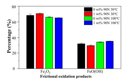
Figure 13. Proportion of Fe<sub>2</sub>O<sub>3</sub> and FeO(OH) in friction oxidation products.
