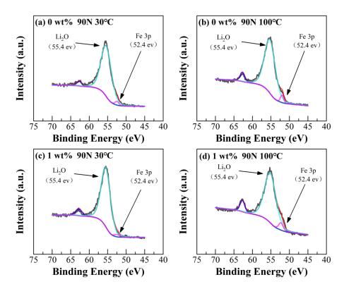
Figure 12. XPS analysis results of Li1s on the worn surfaces of steel plates.
