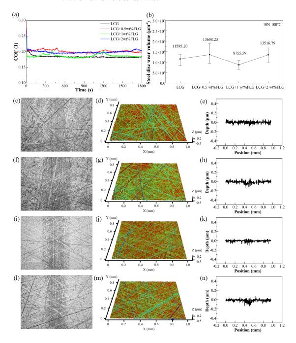
**Figure 6.** (a) COF curves of LCG; (b) abrasion volume of worn surfaces; (c,f,i,l) surface appearance of steel plate abrasion scars; (d,g,j,m) three-dimensional appearance of steel plate abrasion scars and; (e,h,k,n) sectional view of steel plate abrasion scars under 10 N, 100 °C.
