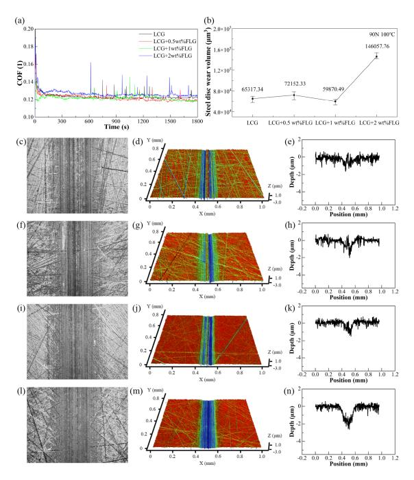
**Figure 8.** (a) COF curves of LCG; (b) abrasion volume of worn surfaces; ( $\mathbf{c}, \mathbf{f}, \mathbf{i}, \mathbf{l}$ ) surface appearance of steel plate abrasion scars; ( $\mathbf{d}, \mathbf{g}, \mathbf{j}, \mathbf{m}$ ) three-dimensional appearance of steel plate abrasion scars and; ( $\mathbf{e}, \mathbf{h}, \mathbf{k}, \mathbf{n}$ ) sectional view of steel plate abrasion scars under 90 N, 100 °C.
