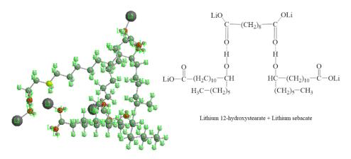
Figure 1. Chemical configuration of thickener for lithium compound grease.
