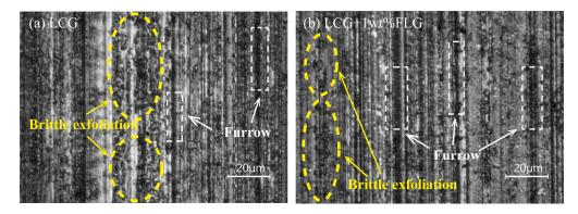
**Figure 15.** The enlarged perspective of the abrasion scar lubricated with LCG and LCG + 1 wt% FLG under 90 N and 100  $^{\circ}$ C.
