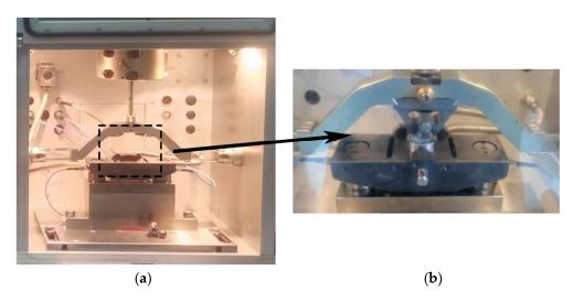
Figure 2. Wear testing equipment and sketch diagram of tribology principle: (a) SRV-5; (b) Test platform.
