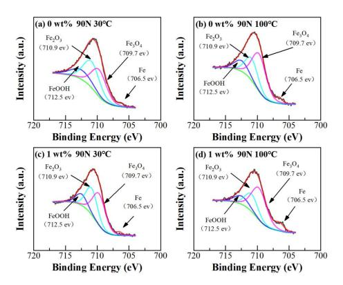
Figure 11. XPS analysis results of Fe2p on the worn surfaces of steel plates.
