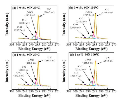
Figure 9. XPS analysis results of C1s on the worn surface of steel plates.
