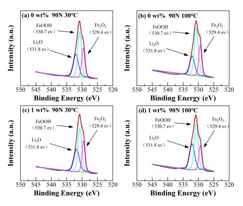
Figure 10. XPS analysis results of O1s on the worn surfaces of steel plates.
