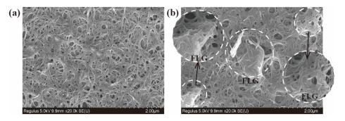
Figure 4. SEM images: (a) pure LCG; (b) LCG with 1 wt% FLG.
