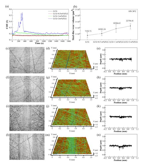
Figure 5. (a) COF curves of LCG; (b) abrasion volume of worn surfaces; ( $\mathbf{c},\mathbf{f},\mathbf{i},\mathbf{l}$ ) surface appearance of steel plate abrasion scars; ( $\mathbf{d},\mathbf{g},\mathbf{j},\mathbf{m}$ ) three-dimensional appearance of steel plate abrasion scars and; ( $\mathbf{e},\mathbf{h},\mathbf{k},\mathbf{n}$ ) sectional view of steel plate abrasion scars under 10 N, 30 °C.
