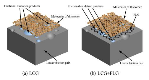
Figure 14. Schematic drawing of frictional mechanism model: (a) LCG; (b) LCG + FLG.
