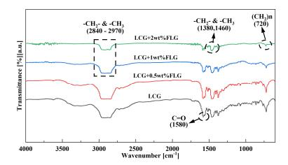
Figure 3. Fourier infrared spectra of four kinds of lithium compound greases.
