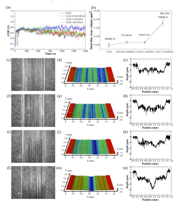
**Figure 7.** (a) COF curves of LCG; (b) abrasion volume of worn surfaces; ( $\mathbf{c}$ , $\mathbf{f}$ , $\mathbf{i}$ , $\mathbf{l}$ ) surface appearance of steel plate abrasion scars; ( $\mathbf{d}$ , $\mathbf{g}$ , $\mathbf{j}$ , $\mathbf{m}$ ) three-dimensional appearance of steel plate abrasion scars and; ( $\mathbf{e}$ , $\mathbf{h}$ , $\mathbf{k}$ , $\mathbf{n}$ ) sectional view of steel plate abrasion scars under 90 N, 30 °C.
