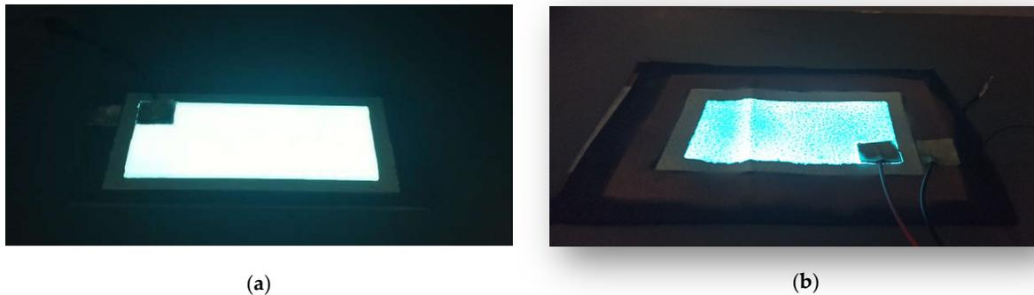
**Figure 6.** ACPEL devices: (a) sample S1, functionalized on the PC/ABS substrate; (b) sample S2, functionalized on the polyester substrate.
