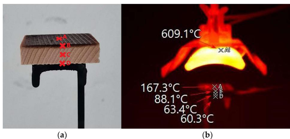
**Figure 1.** Locations of points for thermal camera measurement (a) and infrared snapshot (b).
