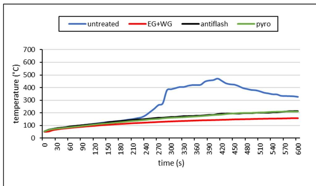
**Figure 8.** Temperature course of the samples at point D (untreated = reference samples, EG + WG = expandable graphite in combination with water glass, antifiash = Bochemit Antifiash, pyro = Bochemit Pyro).
