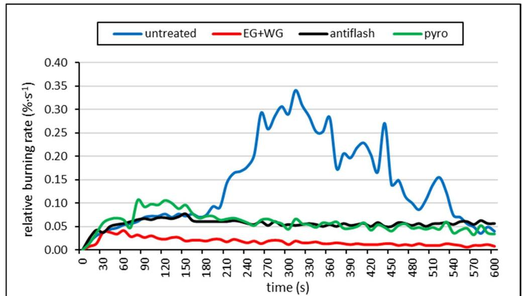
**Figure 4.** Relative burning rate of the samples during the test with a radiant heat source (untreated = reference samples, EG + WG = expandable graphite in combination with water glass, antiflash = Bochemit Antiflash, pyro = Bochemit Pyro).
