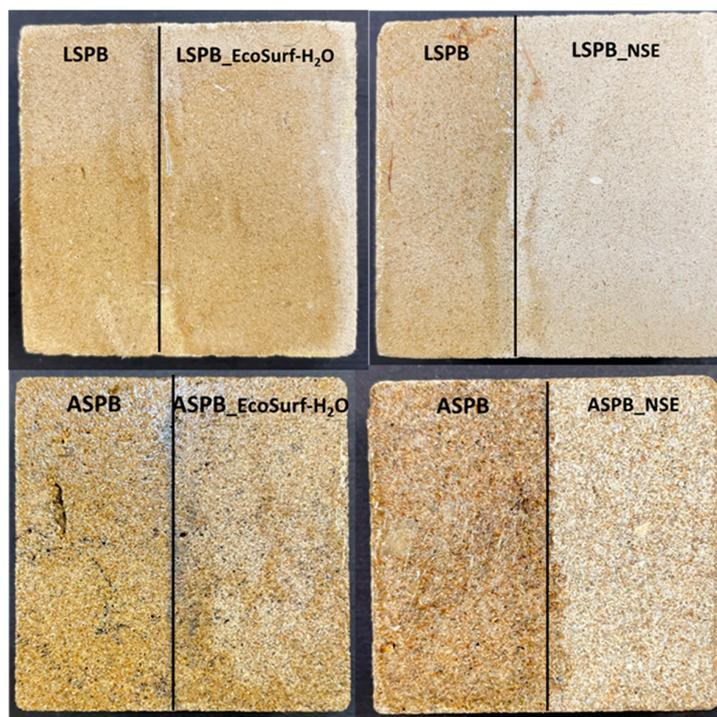
**Figure 4.** Coated LS and AS before and after exposure to the cleaning process using two different emulsions (EcoSurf/H<sub>2</sub>O and NSE). For each specimen, the vertical bar demarcates the coated area (**left**) and the area treated with the emulsion-coated hydrogel (**right**).
