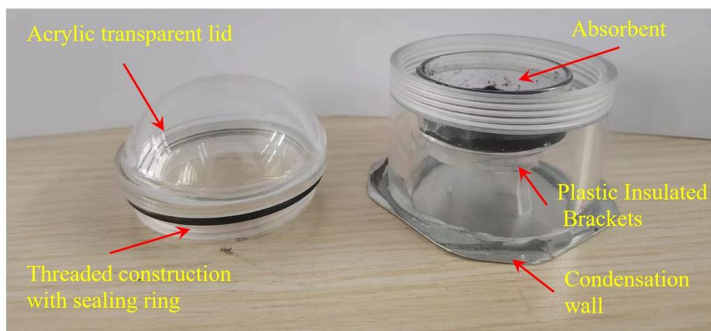
**Figure 7.** Structure of the desorption vessel.
