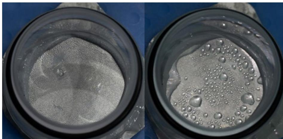
**Figure 8.** Condensation on desorption vessel cooling walls.
