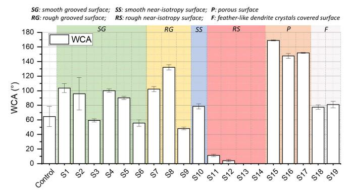
Figure 22. WCA of samples with their classifications, plus the control sample (untreated surface).
