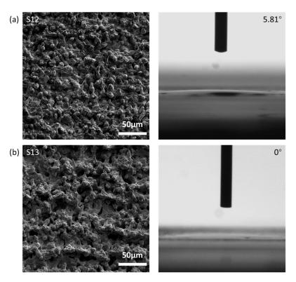
**Figure 27.** SEM images of (**a**) hydrophilic RS samples, (**b**) superhydrophilic RS samples, with their WCA results.
