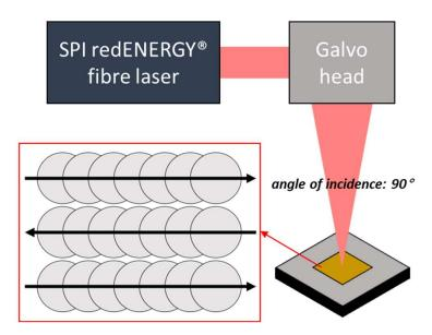
Figure 1. Laser setup and scanning patterns.
