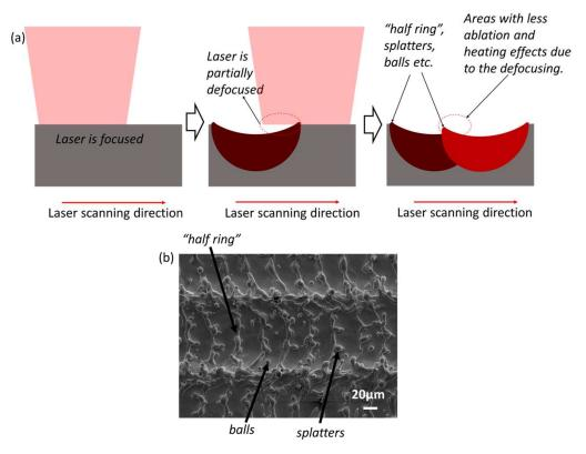
**Figure 14.** Laser texturing mechanism of a single line scanning using a nanosecond infrared laser on metals. (a) The ablation of two adjacent pulse; (b) The morphology of "half ring", balls and splatters.
