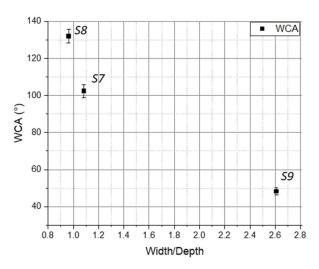
Figure 25. WCA change with groove width/depth ratio for RG samples.
