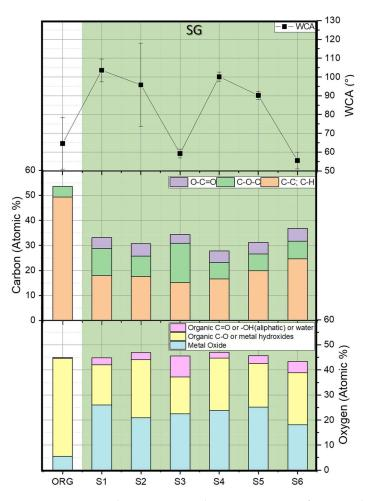
Figure 24. WCA, carbon contents and oxygen contents of SG samples.
