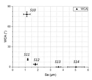
Figure 26. WCA change with surface roughness for SS and RS samples.
