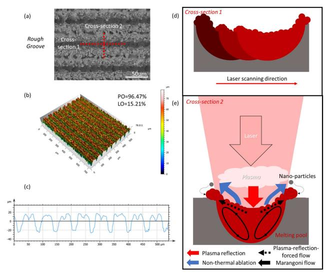
**Figure 16.** Rough groove surface texture: (a) SEM image of sample S7; (b) surface 3D structure of sample S7; (c) average cross-section view of sample S7; (d,e) two cross-section view of laser ablation mechanism.
