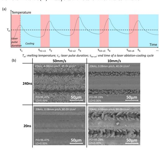
**Figure 21.** Surface textures at low feed speed: (a) temperature–time curve at extremely low feed speed; (b) SEM images of samples with various feed speeds and pulse widths, frequency 20 kHz, pitch 0.08, fluence 40.04 J/cm<sup>2</sup> for 240 ns samples, fluence 80.09 J/cm<sup>2</sup> for 240 ns samples.
