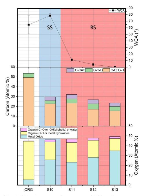
Figure 28. WCA, carbon contents and oxygen contents of SS, RS samples.
