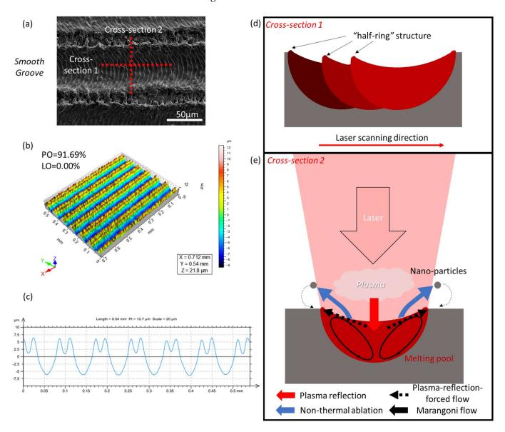
**Figure 15.** Smooth groove surface texture: (a) SEM image of sample S5; (b) surface 3D structure of sample S5; (c) average cross-section view of sample S5; (d,e) two cross-section view of laser ablation mechanism.
