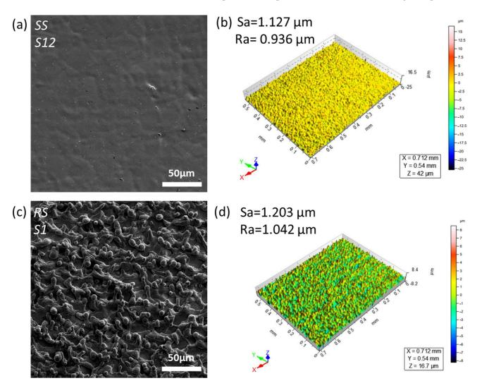
**Figure 9.** (a) SEM image of SS sample (S10). (b) 3D surface structure of S10. (c) SEM image of one of RS sample (S11). (d) 3D surface structure of S11.
