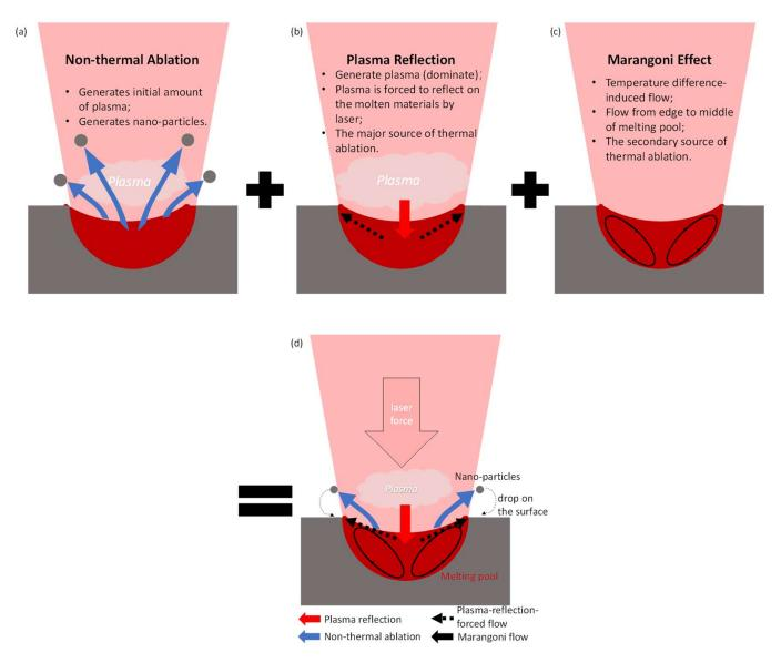
**Figure 13.** Laser texturing mechanism for metals of single spot by nanosecond infrared laser. (a) Nonthermal ablation, (b) plasma reflection, (c) Marangoni effect. Part of the schematic diagram is adopted from Leitz et al. [38], Hamad [39], Lahaye et al. [40], He et al. [41] and Gaudiuso [42].
