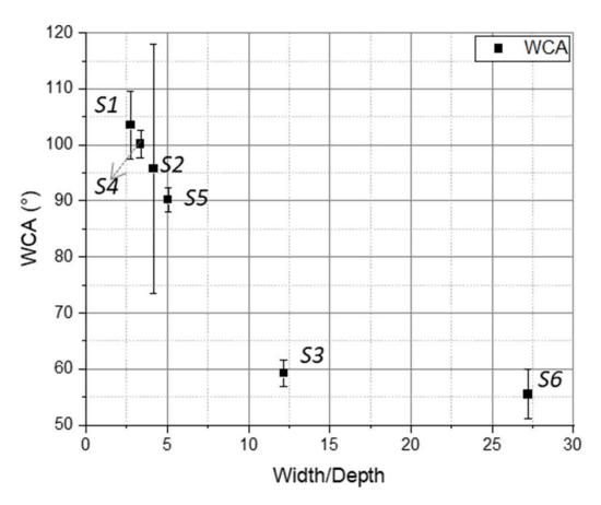
Figure 23. WCA change with groove width/depth ratio for SG samples.
