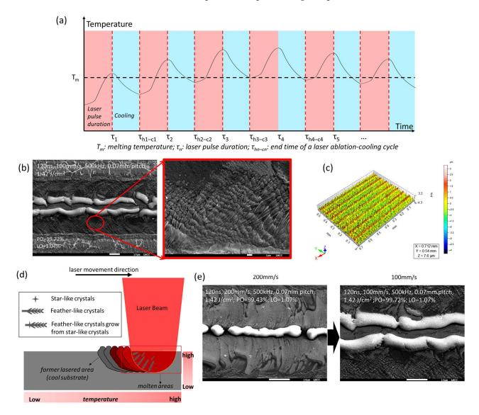
**Figure 20.** Feather-like dendrites texture-covered textures: (a) temperature—time curve at extremely high frequency; (b) SEM images of F sample S19; (c) surface 3D structure of S19; (d) formation of dendrites; (e) morphology change while reducing feed speed from 200 mm/s (S18) to 100 mm/s (S19).
