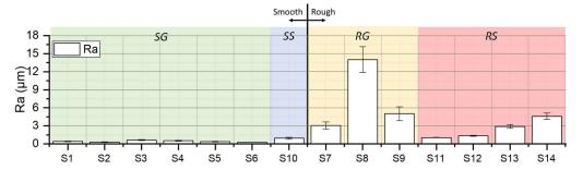
Figure 5. Ra of SG, SS, RG, and RS samples.
