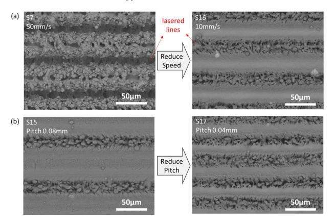
**Figure 10.** (a) Fabrication of P samples through reducing feed speed. Other laser parameters: 240 ns, 20 kHz, 35.58 J/cm<sup>2</sup>, 0.06 mm pitch. (b) Reducing pitch to make porous structures cover the whole surface. Other laser parameters: 240 ns, 20 mm/s, 20 kHz, 35.58 J/cm<sup>2</sup>.
