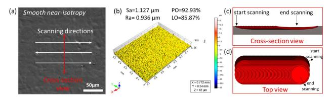
**Figure 17.** Smooth near-isotropic structure: (a) SEM of S10, (b) surface 3D structure of S10, and (c,d) formation mechanism.
