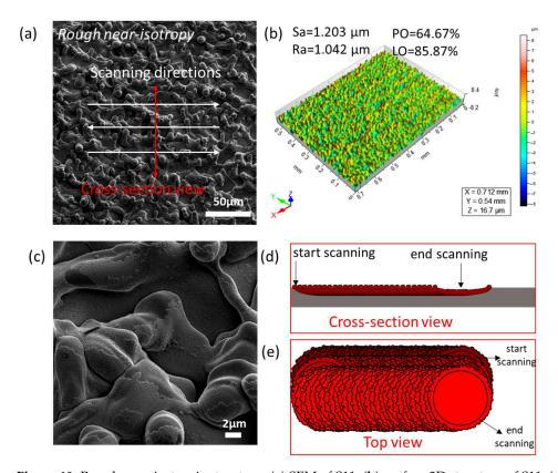
**Figure 18.** Rough near-isotropic structure: (a) SEM of S11, (b) surface 3D structure of S11, (c) nano features covered micro-protrusion (S11), and (d,e) formation mechanism.
