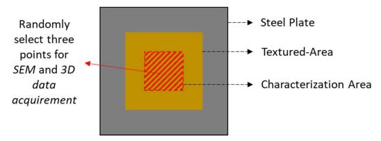
**Figure 2.** Schematic diagram to show the characterisation area.
