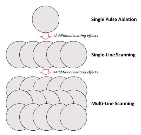
Figure 12. Accumulation effects from spot ablation to surface ablation.
