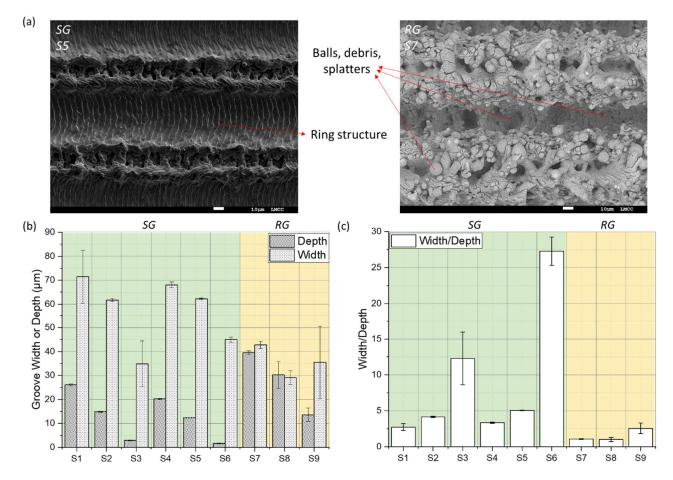
**Figure 8.** (a) Typical topographies of SG and RG samples. (b) Depth and width of SG and RG samples. (c) Aseptic ratio of grooves of SG and RG samples.
