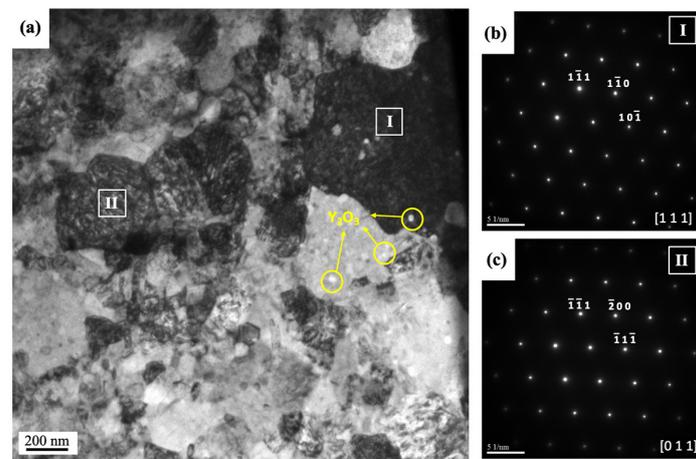
**Figure 8.** TEM investigations of the bulk  $\text{AlCoCrFeNi}_{2.1} + 2 \text{ wt.}\% \text{Y}_2\text{O}_3$ : (a) TEM bright-field image and the SAD patterns corresponding to (b) point “I” and (c) point “II”.
