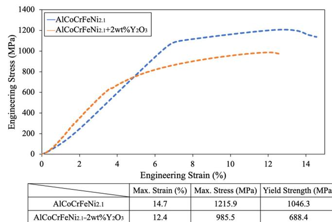
Figure 13. Compressive engineering stress–strain curves of the sintered bulk materials.
