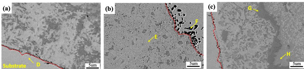
Figure 5. SEM images of the AlCoCrFeNi<sub>2.1</sub> coatings after annealing treatment for (a) 4 h, (b) 8 h, and (c) 16 h of milling.
