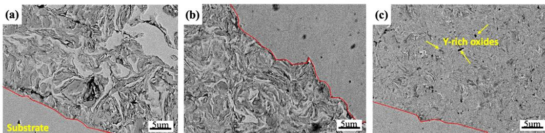
Figure 4. SEM images of the AlCoCrFeNi<sub>2.1</sub> with 2 wt.% of Y<sub>2</sub>O<sub>3</sub> coatings milled for (a) 4 h, (b) 8 h, and (c) 16 h.
