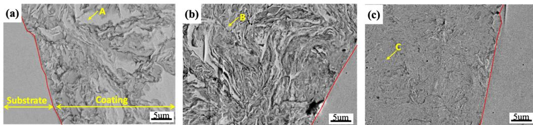
Figure 3. SEM images of the AlCoCrFeNi<sub>2.1</sub> coatings milled for (a) 4 h, (b) 8 h, and (c) 16 h.
