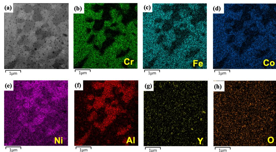
**Figure 10.** TEM-EDS mapping of the bulk  $\text{AlCoCrFeNi}_{2.1} + 2 \text{ wt.}\% \text{Y}_2\text{O}_3$ : (a) SEM image, (b) Cr map, (c) Fe map, (d) Co map, (e) Ni map, (f) Al map, (g) Y map, and (h) O map.
