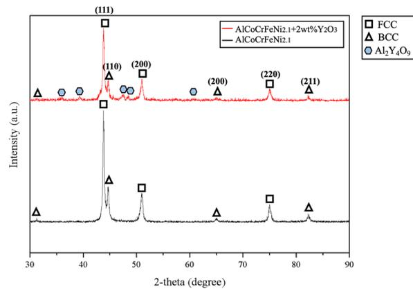
Figure 11. XRD spectra of the sintered bulk EHEAs.
