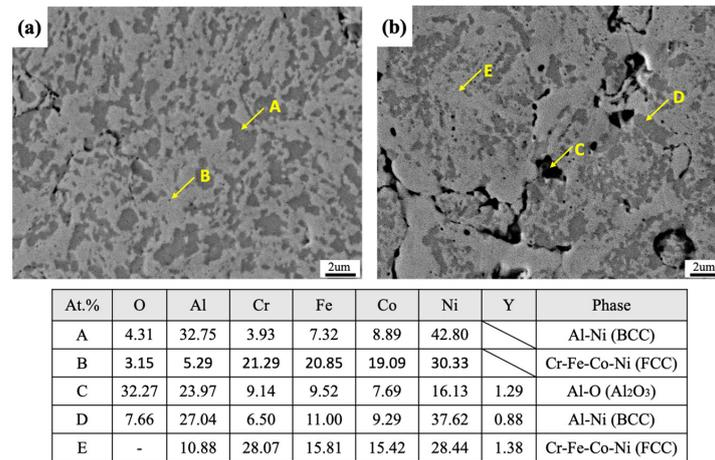
**Figure 7.** SEM images of the sintered bulk materials milled for 16 h: (a) AlCoCrFeNi<sub>2.1</sub> and (b) AlCoCrFeNi<sub>2.1</sub> with 2 wt.% of Y<sub>2</sub>O<sub>3</sub>.
