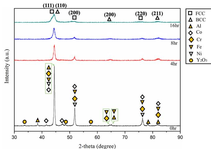
**Figure 2.** XRD spectra of the AlCoCrFeNi<sub>2.1</sub> added with 2 wt.% of Y<sub>2</sub>O<sub>3</sub> powder milled for different milling durations: 0 h, 4 h, 8 h, and 16 h.
