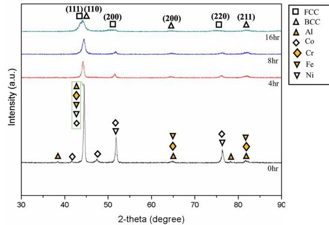
**Figure 1.** XRD spectra of the AlCoCrFeNi<sub>2.1</sub> powders milled for different milling durations: 0 h, 4 h, 8 h, and 16 h.
