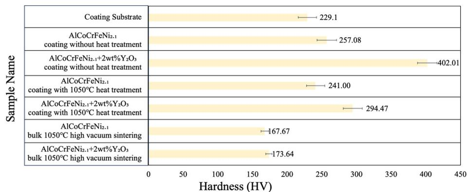
Figure 12. The microhardness of the model coatings and sintered bulk materials.
