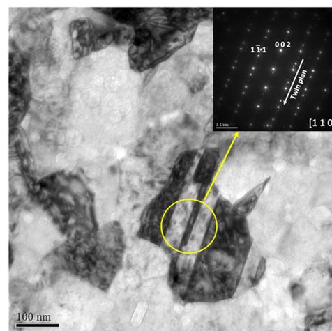
**Figure 9.** TEM investigation of the twinned structure in FCC phase.
