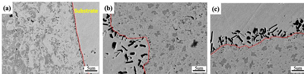
**Figure 6.** SEM images of the AlCoCrFeNi<sub>2.1</sub> with 2 wt.% of Y<sub>2</sub>O<sub>3</sub> coatings after annealing treatment for (a) 4 h, (b) 8 h, and (c) 16 h of milling.
