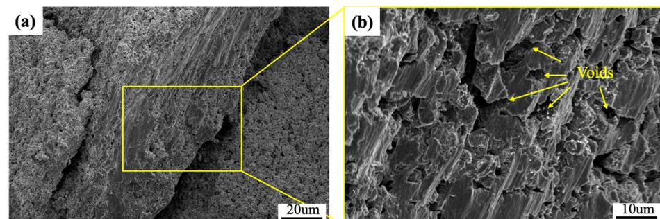
Figure 14. Fracture surfaces of the bulk AlCoCrFeNi<sub>2.1</sub> + 2 wt.% Y<sub>2</sub>O<sub>3</sub>.
