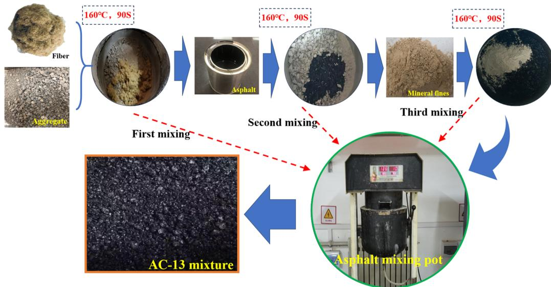
Figure 4. The fiber asphalt mixture mixing process.
