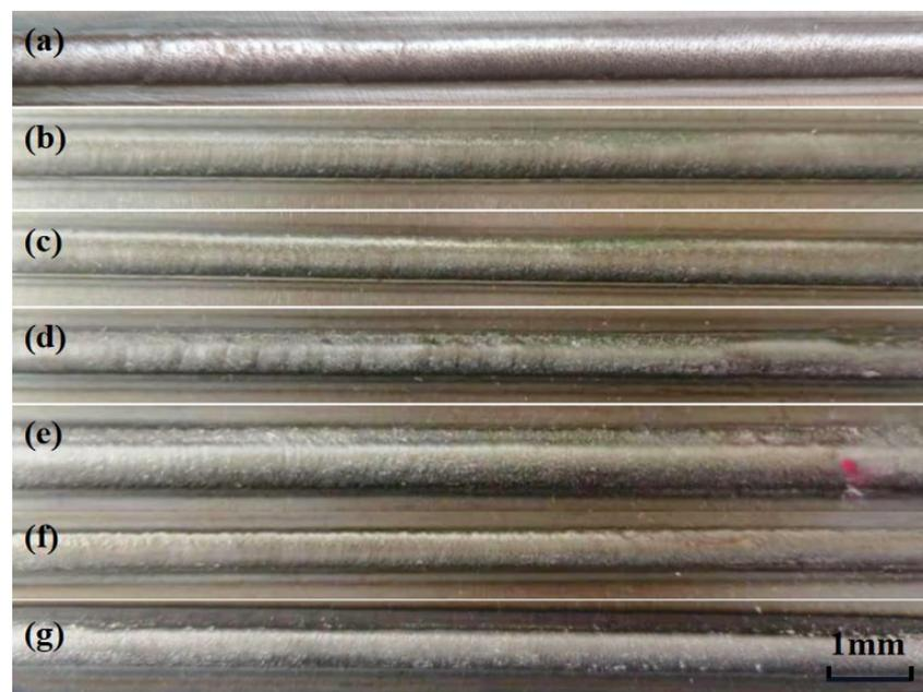
**Figure 2.** Macromorphology of the cladding layers after forming with different processes. (a) The optimal forming process; (b) a scanning speed of 0.003 m/s; (c) a scanning speed of 0.004 m/s; (d) a laser power of 1.8 kW; (e) a laser power of 2.6 kW; (f) a powder feed rate of 0.429 kg/h; and (g) a powder feed rate of 0.966 kg/h.
