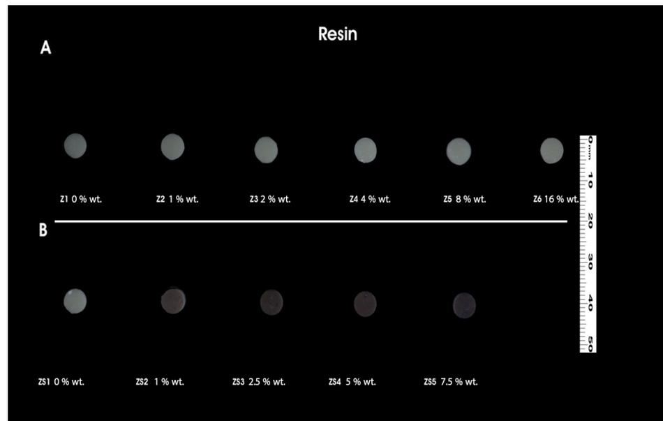
**Figure 3.** 3D-printed samples for Vickers microhardness. (A) Unmodified 3D-printed resin (Z1); ZrO<sub>2</sub> 1 %wt. (Z2); ZrO<sub>2</sub> 2 %wt. (Z3); ZrO<sub>2</sub> 4 %wt. (Z4); ZrO<sub>2</sub> 8 %wt. (Z5); ZrO<sub>2</sub> 16 %wt. (Z6); (B) HNC/Ag 0 %wt. (ZS1); HNC/Ag 1 %wt. (ZS2); HNC/Ag 2.5 %wt. (ZS3); HNC/Ag 5 %wt. (ZS4); HNC/Ag 7.5 %wt. (ZS5).
