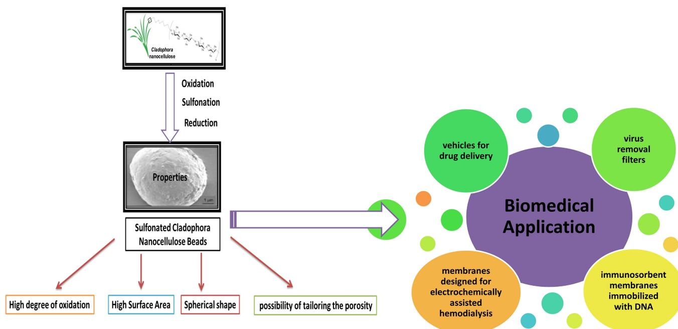
**Figure 7.** Properties of sulfonated Cladophora nano-cellulose beads [59].
