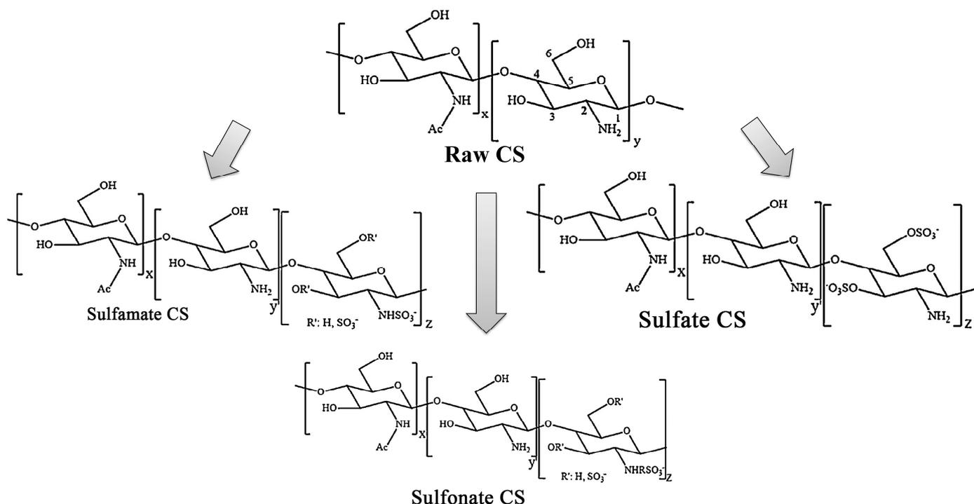
**Figure 4.** Chemical structure scheme of chitosan and its sulfonated derivatives [23].
