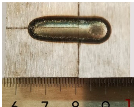
Figure 2. Cladding test block.
