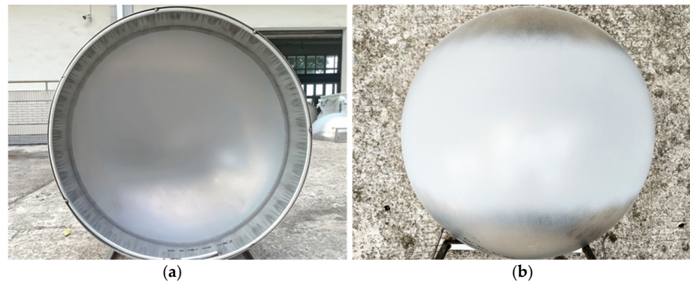
Figure 22. Film formation experiments of spraying on spherical surfaces. (a) Inner surface; (b) outer surface.
