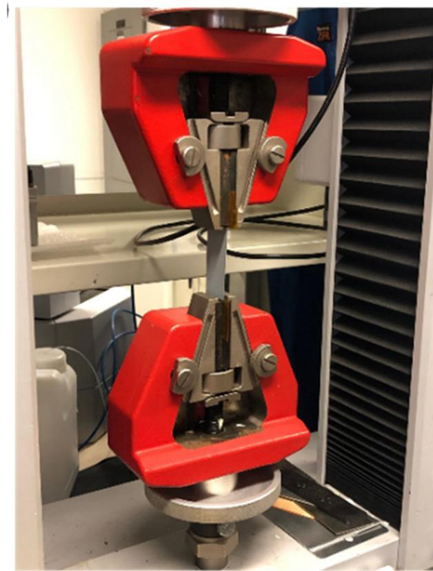
**Figure 3.** Test configuration for measuring the elastic properties of the different coating samples.
