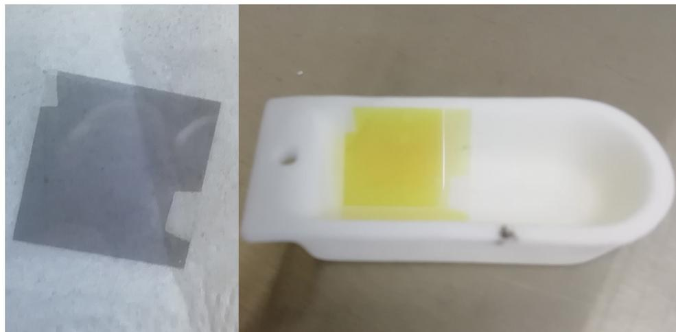
**Figure 2.** Continuous Ag film (Ag #3–12 nm) (left) before and (right) after annealing at 440 °C for 30 min.
