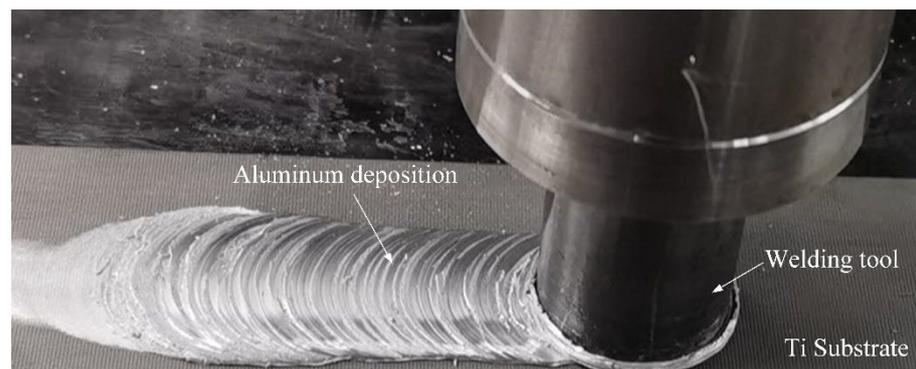
**Figure 4.** Verification of Ti/Al deposition by SRFD equipment.
