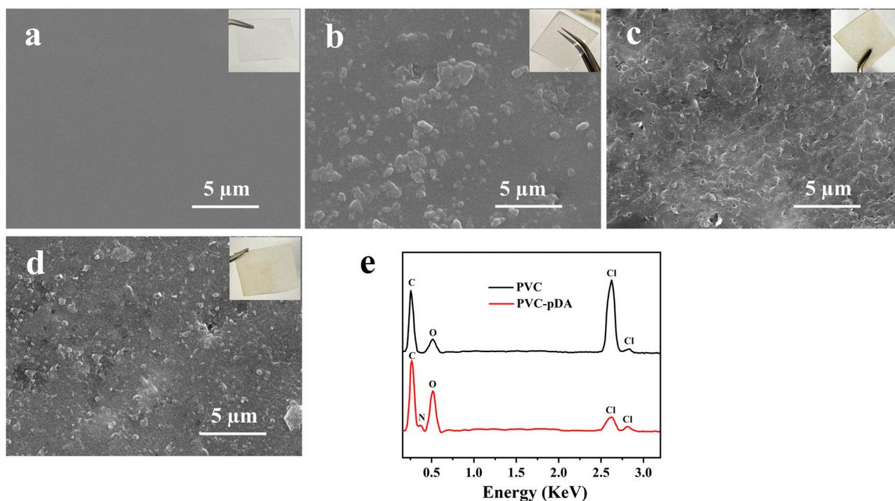
**Figure 2.** SEM images (insets are the corresponding photographs) of (a) PVC, (b) PVC-pDA, (c) PVC-pDA/HBPL, (d) PVC-pDA-HBPL; and (e) EDS spectrum of pristine PVC and PVC-pDA.
