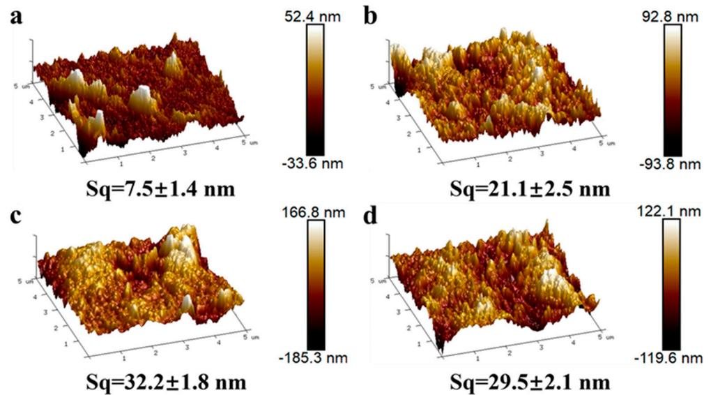
**Figure 3.** Three-dimensional maps characterizing the AFM results for (a) PVC, (b) PVC-pDA, (c) PVC-pDA/HBPL, and (d) PVC-pDA-HBPL. The variable  $S_q$  denotes the root mean square of surface roughness in the given area.
