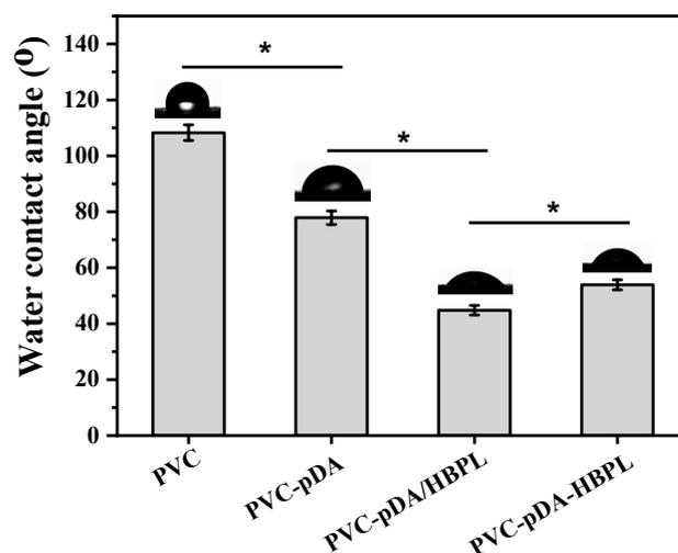
**Figure 5.** Water contact angles of unmodified and modified PVC substrates. \* indicates significant difference at  $p < 0.05$  level.
