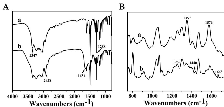
**Figure 9.** (A) FTIR and (B) Raman spectra of (a) pDA and (b) pDA/HBPL acquired from a solution-based reaction in the absence of PVC film.
