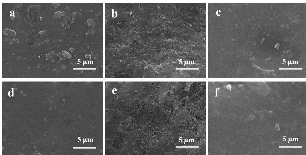
**Figure 6.** SEM images of (a,d) PVC-pDA, (b,e) PVC-pDA/HBPL, and (c,f) PVC-pDA-HBPL eluted with 1.0 M HCl (a–c) or 1.0 M NaOH solution (d–f) for 24 h.
