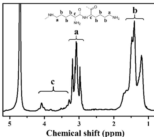
**Figure 1.**  $^1\text{H}$  NMR spectrum of HBPL (a, b, and c denote the chemical shifts corresponding to distinct hydrogen species in HBPL).
