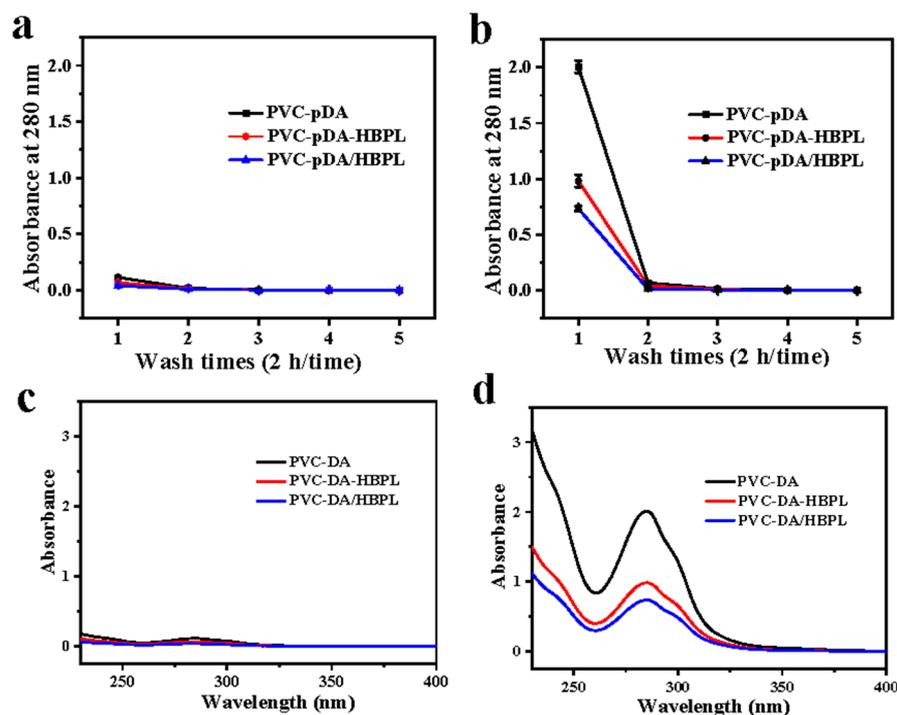
**Figure 7.** (a,b) Absorbance at 280 nm of eluent from modified samples during repeated elution (2 h/time) with (a) 1.0 M HCl or (b) 1.0 M NaOH solution ( $n = 4$ ). (c,d) UV-vis spectra of the eluent of modified materials immersed in (c) 1.0 M HCl or (d) 1.0 M NaOH solution for 2 h.
