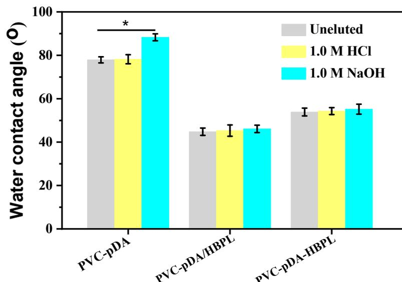
**Figure 8.** Water contact angles of PVC-pDA, PVC-pDA/HBPL, and PVC-pDA-HBPL after elution with 1.0 M HCl or 1.0 M NaOH solution for 2 h. \* indicates significant difference at  $p < 0.05$  level.
