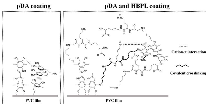
**Figure 10.** Schematic representation of interactions on PVC films with pDA and pDA/HBPL coatings.
