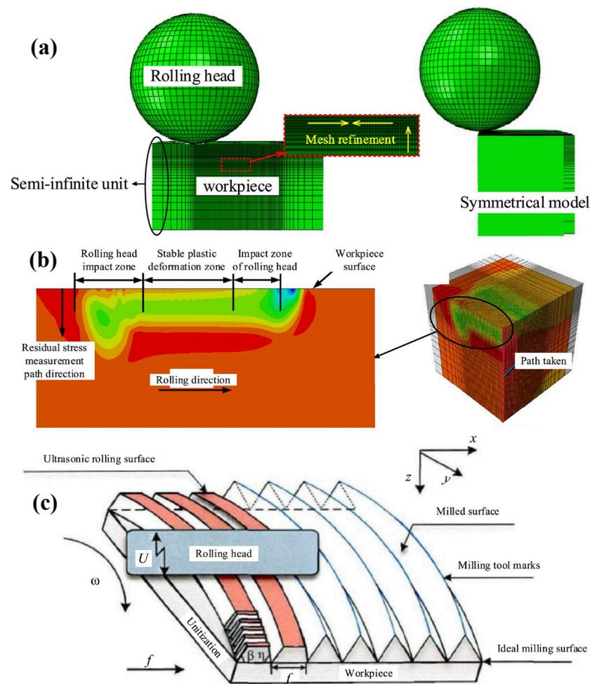
**Figure 12.** (a) Mesh division of a 3D finite element model; (b) residual stress distribution (left) and junction path (right) after ultrasonic rolling; the green area indicates the stable residual compressive stress layer near the surface of the processed workpiece; (c) schematic diagram of ultrasonic rolling [72]. (Reused with permission from ref. [72]. Copyright 2022, Elsevier).
