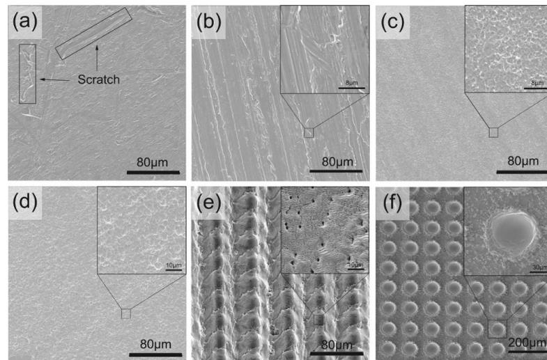
**Figure 10.** Surface microstructure after treatment. (a) Metallographic grinding; (b) parallel grinding; (c) diamond blasting and acid etching; (d)  $\text{Al}_2\text{O}_3$  blasting and acid etching; (e) laser groove array; (f) laser pore array [64]. (Reused with permission from ref. [64]. Copyright 2020, Elsevier).
