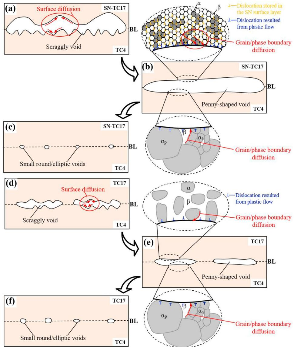
**Figure 13.** Evolution mechanism of voids in the bonding interface of SN-TC17/TC4 and TC17/TC4 bond: (a,d) are scraggly voids, (b,e) are penny-shaped voids, and (c,f) are round/elliptic voids [78]. (Reused with permission from ref. [78]. Copyright 2022, Elsevier).
