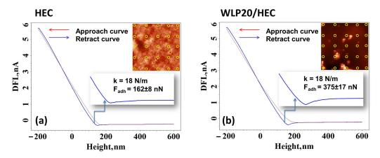
**Figure 8.** Typical DFL-height curves (red, approach curve; blue retract, curve) registered for the HEC matrix (a) and WLP20/HEC system (b). The place where each curve was collected is indicated on the AFM images inserted in the upper right corner.
