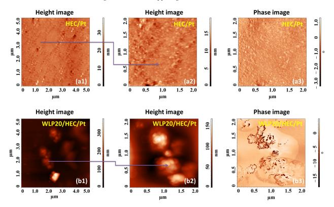
Figure 9. Height and phase AFM images recorded for the HEC/Pt and WLP20/HEC/Pt systems.
