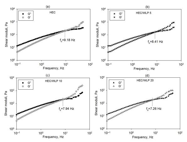
**Figure 2.** The shear moduli variation with frequency for the (a) HEC, (b) WLP5/HEC, (c) WLP10/HEC, and (d) WLP20/HEC systems.
