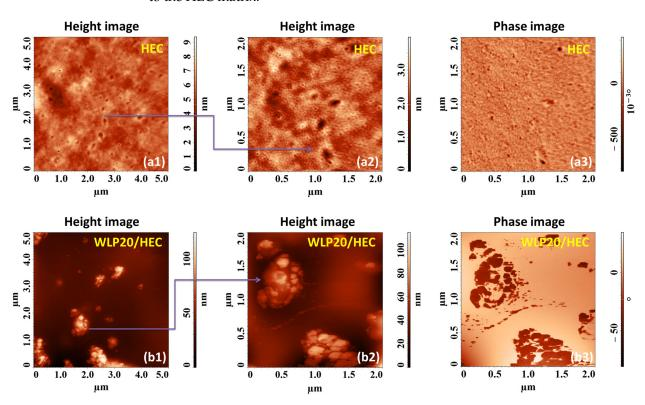
Figure 7. Height and phase AFM images recorded for the HEC and WLP20/HEC systems.
