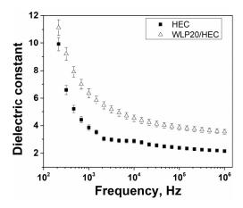
Figure 10. The dielectric spectra of HEC and WLP20/HEC samples at ambient temperature.
