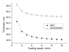
Figure 5. The thickness variation with casting speed for the HEC and WLP20/HEC systems.
