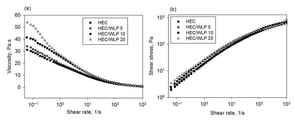
**Figure 1.** The viscosity (a) and shear stress (b) dependencies on the imposed shear rate for the HEC and WLP/HEC systems.
