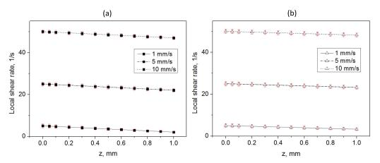
Figure 4. Local shear rate distributions below the blade for the (a) HEC and (b) WLP20/HEC systems.
