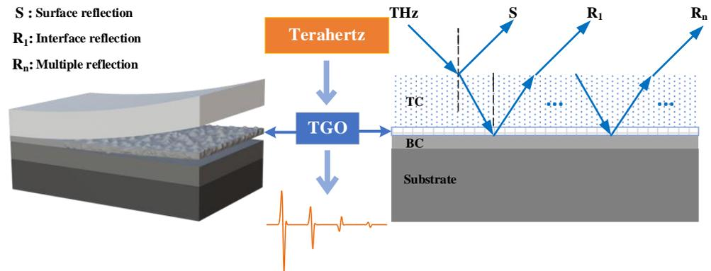
Figure 1. Schematic diagram of terahertz non-destructive testing of TBCs.
