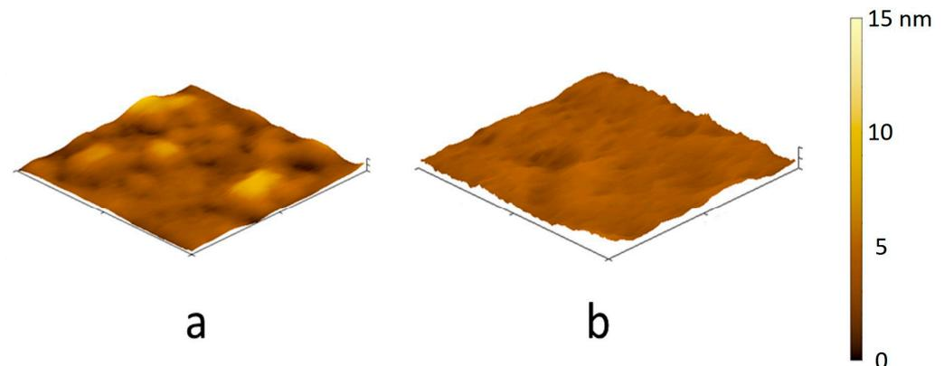
**Figure 6.** AFM images of four polycationic coatings from PEI-750 (a) and PDADMAC-500 (b) on a glass surface. Scanning area 500 nm × 500 nm.
