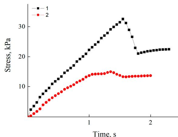
**Figure 5.** Typical stress versus time curves for PEI-70 (1) and PDADMAC-300 (2). Traverse rate 5 mm/min. Relative humidity  $18 \pm 2\%$ .
