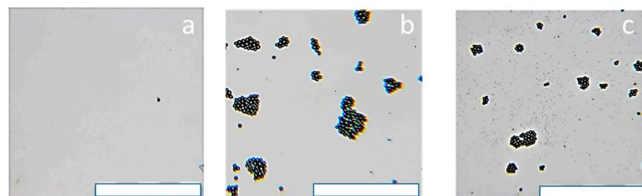
**Figure 7.** Optical microscope images of glass surface (a); glass covered with PEI-750 (b) and glass covered with PDADMAC-500 (c) after contact with latex. White scale-bar 50 μm.
