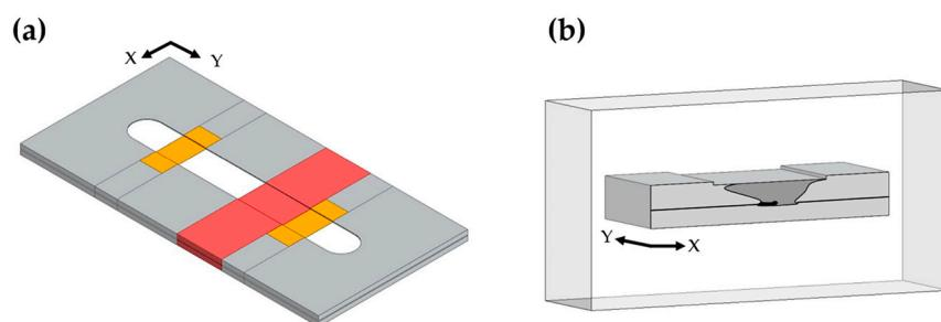
**Figure 4.** Schematic of samples prepared for characterization techniques: (a) analyzed sections; (b) section embedded in resin for macroscopic and microscopic characterization.
