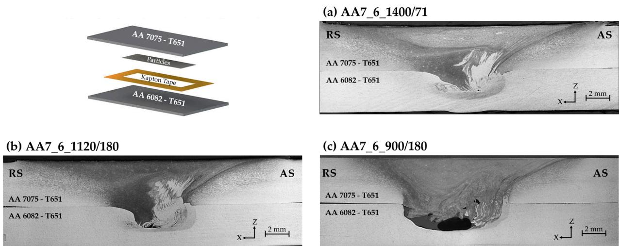
**Figure 5.** Macrography of aluminium-based dissimilar alloys composites produced by UFSP with a lower plate of AA 6082-T651 and an upper plate of AA 7075-T651: (a) AA7\_6\_1400/71; (b) AA7\_6\_1120/180; (c) AA7\_6\_900/180.
