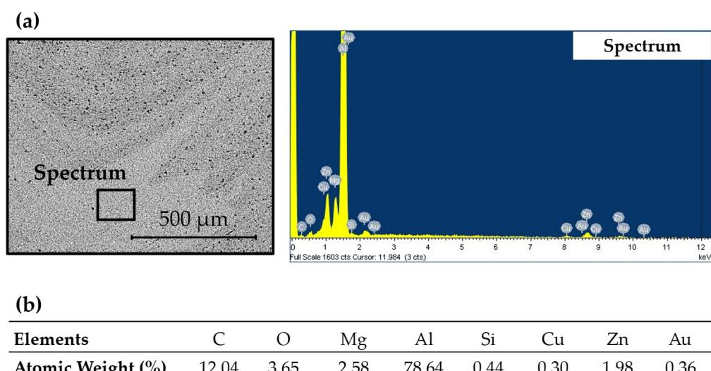
**Figure 17.** Energy dispersive X-ray spectroscopy (EDS) analysis of the “flow arms” in the advancing side of sample AA7\_6\_900/180\_P: (a) spectrum image; (b) atomic weights of the elements within the sample.
