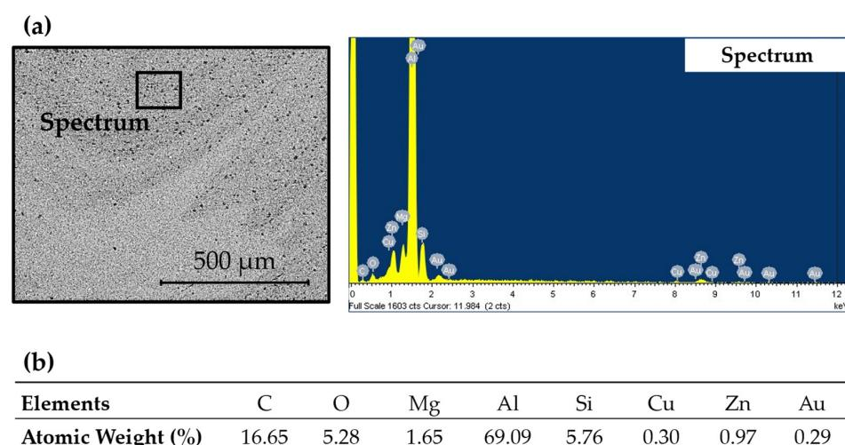
**Figure 16.** Energy dispersive X-ray spectroscopy (EDS) analysis of upper plate in the advancing side of sample AA7\_6\_900/180\_P: (a) spectrum image; (b) atomic weights of the elements within the sample.
