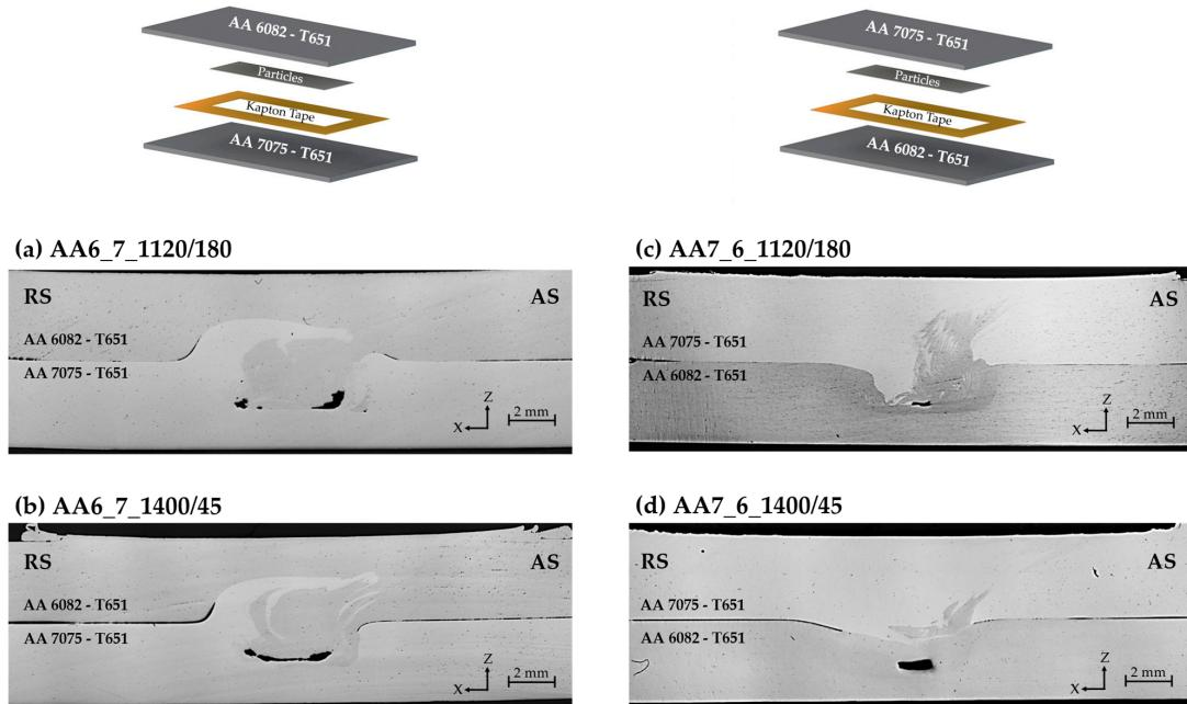
**Figure 7.** Macrography of aluminium-based dissimilar alloys composites produced by UFSP with a lower plate of AA 7075-T651 and an upper plate of AA 6082-T651: (a) AA6\_7\_1120/180; (b) AA6\_7\_1400/45 and dissimilar alloys composites produced with a lower plate of AA 6082-T651 and an upper plate of AA 7075-T651; (c) AA7\_6\_1120/180; (d) AA7\_6\_1400/45.
