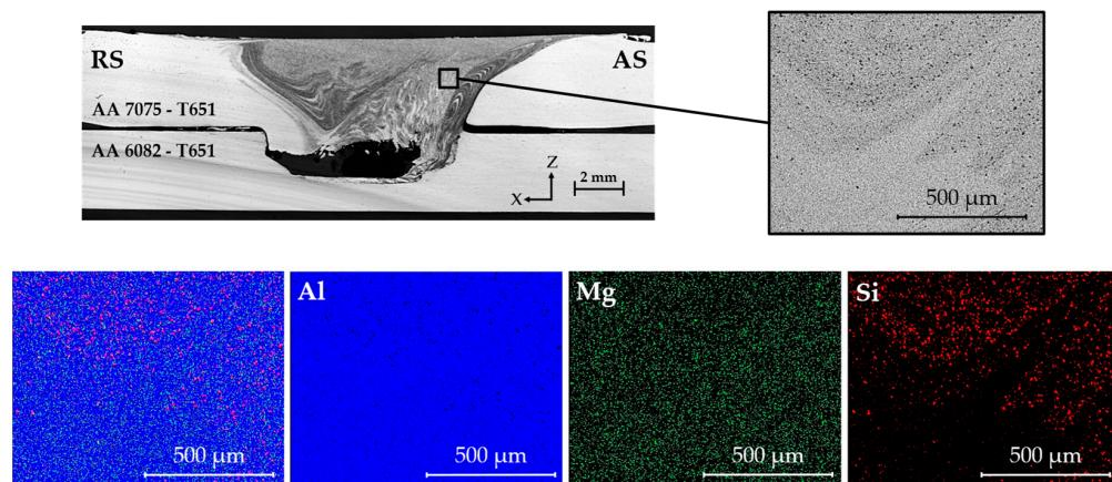
**Figure 15.** Energy dispersive X-ray spectroscopy (EDS) mapping images of sample AA7\_6\_900/180\_P in advancing side.
