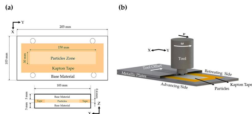
**Figure 2.** Experimental setup of surface composites production by UFSP: (a) top view and transversal view; (b) 3D schematic.
