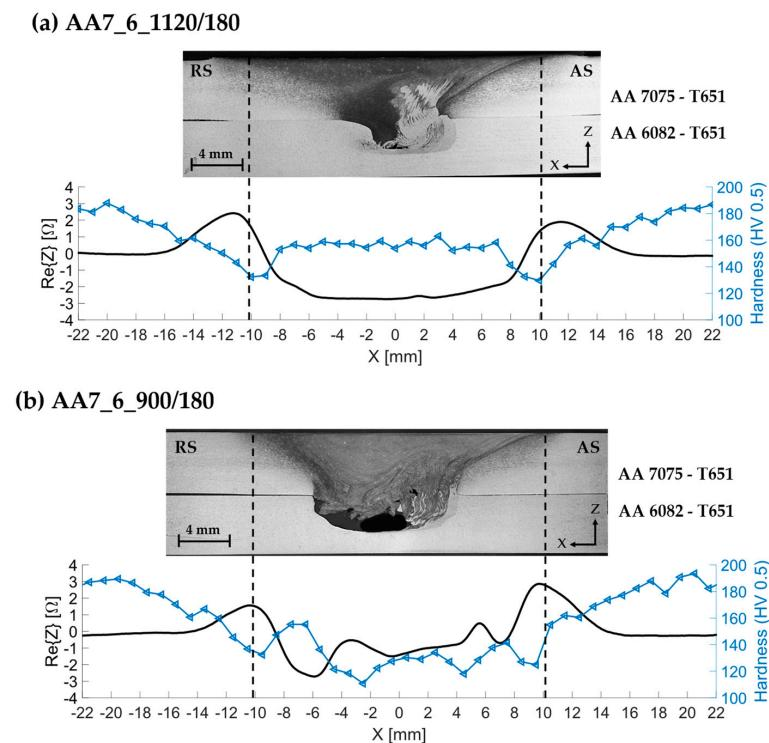
**Figure 8.** Eddy currents and microhardness profiles along the X direction of the plates: (a) AA7\_6\_1120/180 and (b) AA7\_6\_900/180.
