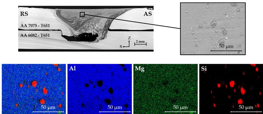
**Figure 13.** Energy dispersive X-ray spectroscopy (EDS) mapping images of sample AA7\_6\_900/180\_P.
