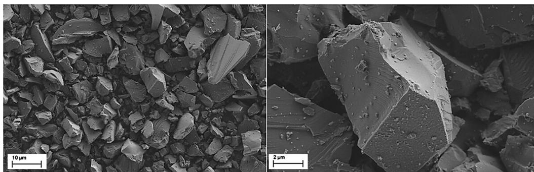
**Figure 1.** Scanning electron microscopy images of SiC particles' morphology and dimensions (adapted from [42]).
