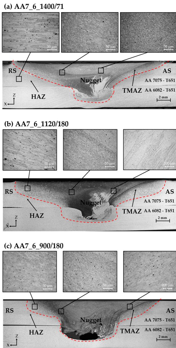
**Figure 6.** Micrography of aluminium-based dissimilar alloys composites produced by UFSP with a lower plate of AA 6082-T651 and an upper plate of AA 7075-T651: (a) AA7\_6\_1400/71; (b) AA7\_6\_1120/180; (c) AA7\_6\_900/180.
