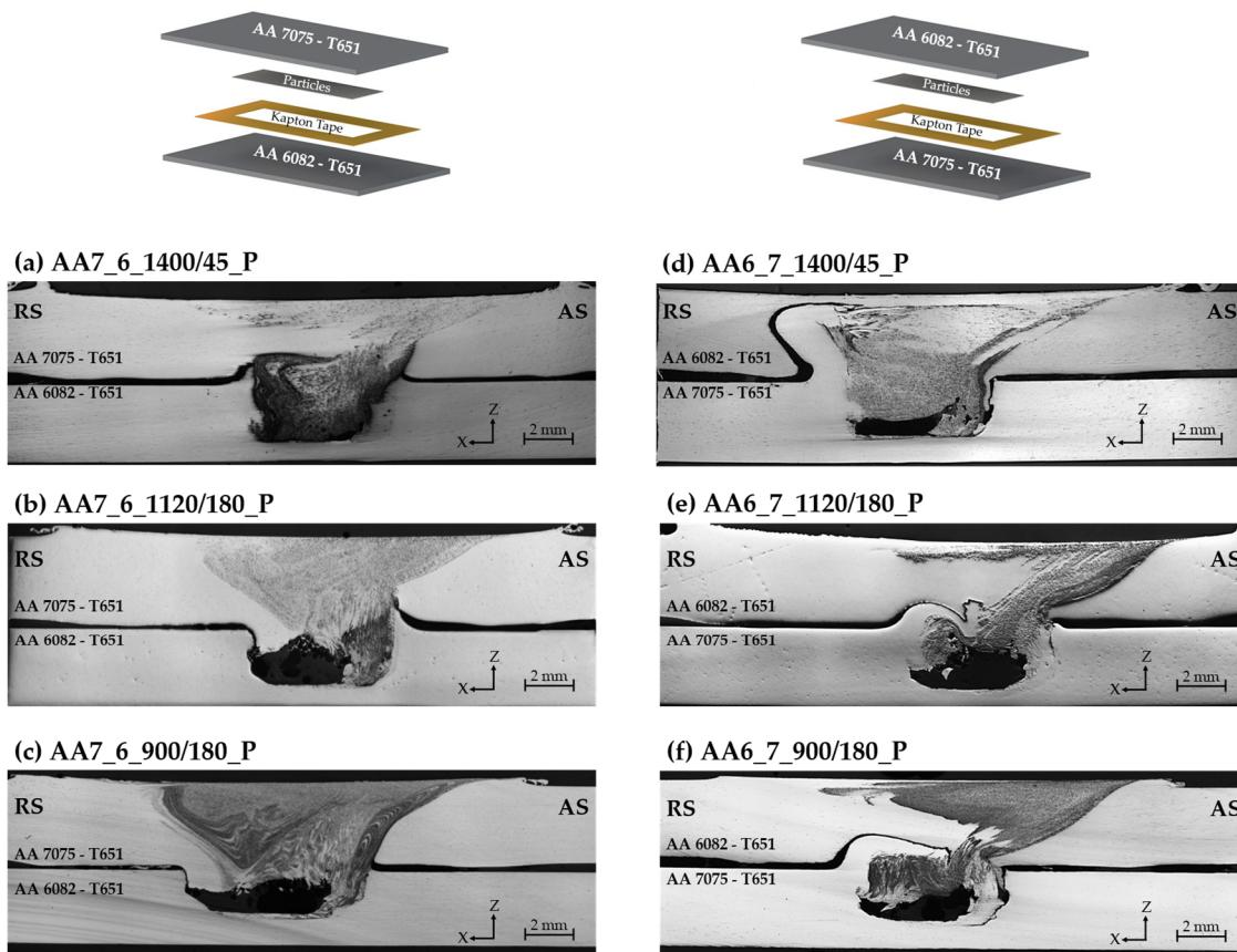
**Figure 9.** Macrography of aluminium-based dissimilar alloys composites reinforced with SiC particles produced by UFSP with a lower plate of AA 6082-T651 and an upper plate of AA 7075-T651: (a) AA7\_6\_1400/45\_P; (b) AA7\_6\_1120/180\_P; (c) AA7\_6\_900/180\_P and composites produced with a lower plate of AA 7075-T651 and an upper plate of AA 6082-T651; (d) AA7\_6\_1400/45\_P; (e) AA7\_6\_1120/180\_P; (f) AA7\_6\_900/180\_P.
