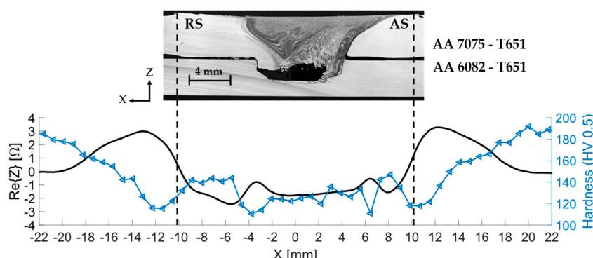
**Figure 11.** Eddy currents and microhardness profiles along the X direction of the plates reinforced with SiC particles: (a) AA7\_6\_1120/180\_P and (b) AA7\_6\_900\_180\_P.
