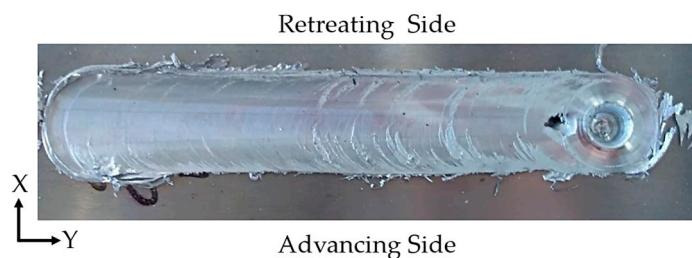
**Figure 12.** Surface composite AA7\_6\_900/180\_P produced by UFSP with a lower plate of AA 6082-T651 and an upper plate of AA 7075-T651.
