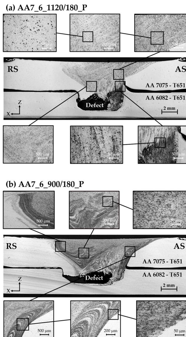
**Figure 10.** Micrography of aluminium-based dissimilar alloys composites reinforced with SiC particles produced by UFSP with a lower plate of AA 6082-T651 and an upper plate of AA 7075-T651: (a) AA7\_6\_1120/180\_P; (b) AA7\_6\_900/180\_P.
