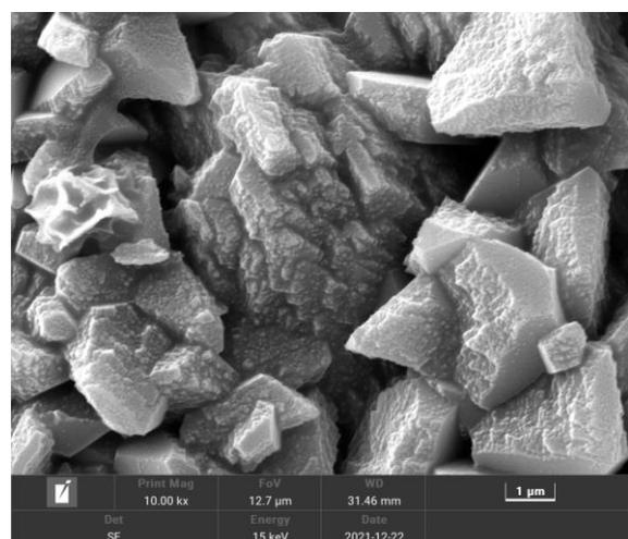
(f) Lime saturated H<sub>2</sub>O at 60 °C for 3 days
