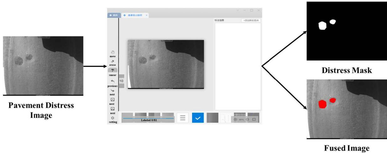
Figure 3. Pothole images labelling procedure.
