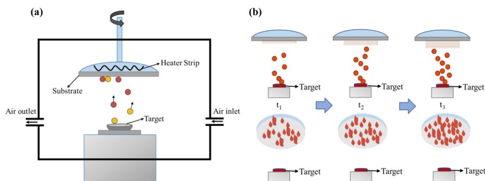
**Figure 1.** The diagram of preparing mineral anti-fog film materials. (a) Device diagram of vacuum evaporation coating machine; (b) growth of films with different thicknesses.
