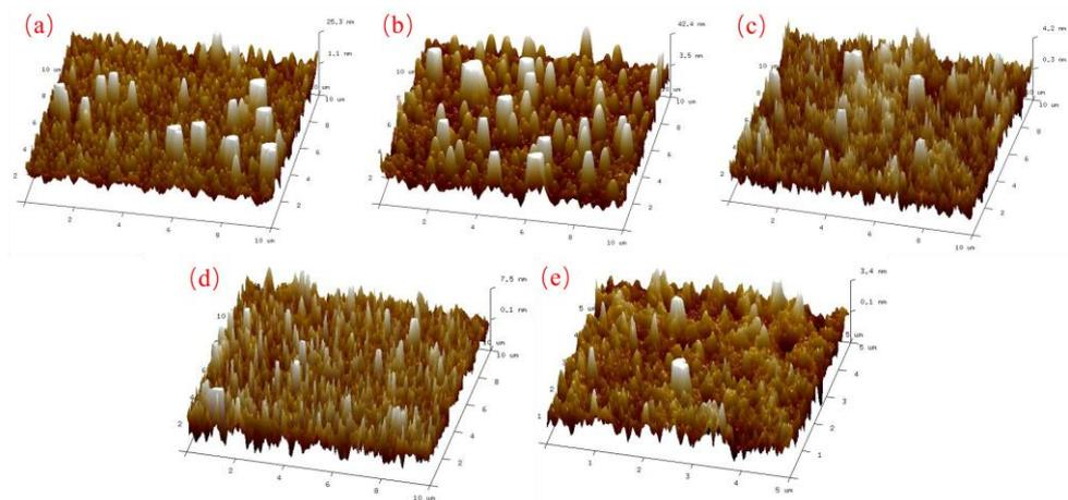
**Figure 5.** AFM images of thin film samples with different film thicknesses: (a) 100 nm; (b) 200 nm; (c) 400 nm; (d) 800 nm; (e) 1000 nm.
