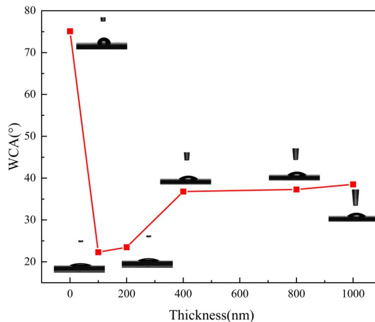
**Figure 4.** Surface contact angles of film samples with different film thicknesses.
