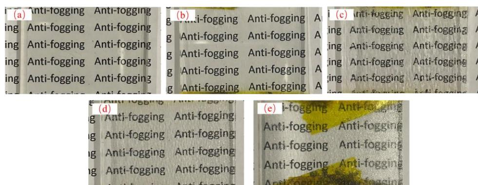
**Figure 3.** Anti-fog effect of film samples with different film thicknesses: (a) 100 nm; (b) 200 nm; (c) 400 nm; (d) 800 nm; (e) 1000 nm.
