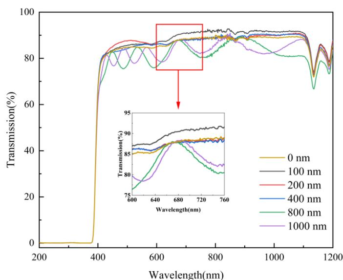
**Figure 7.** Transmittance of film samples with different film thicknesses.
