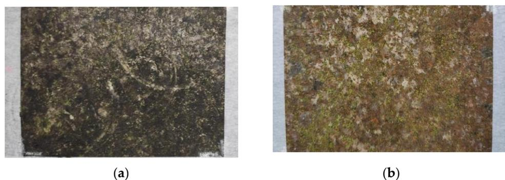
**Figure 1.** Experimental surfaces (details). In the pictures, the two surfaces are compared. In (a) the dark green biopatina is shown (Surface a), and in (b) the green-orange biopatina is shown (Surface b).
