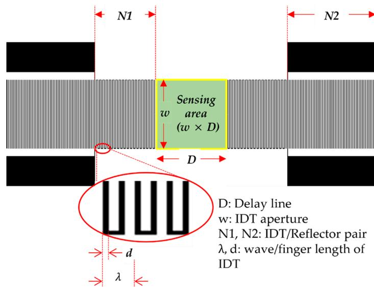
Figure 2. SAW sensor design and parameters.
