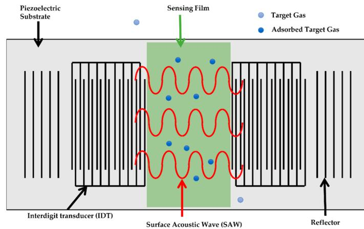
Figure 1. Surface acoustic wave chemical sensor.
