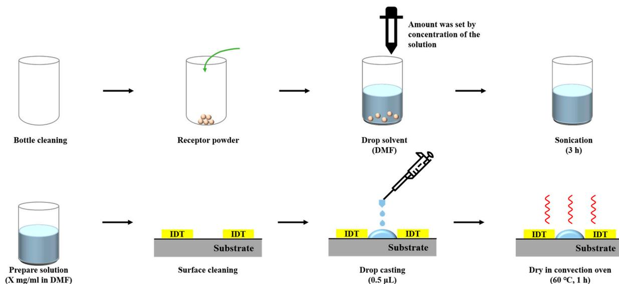
Figure 5. The solution manufacturing process and drop casting process.
