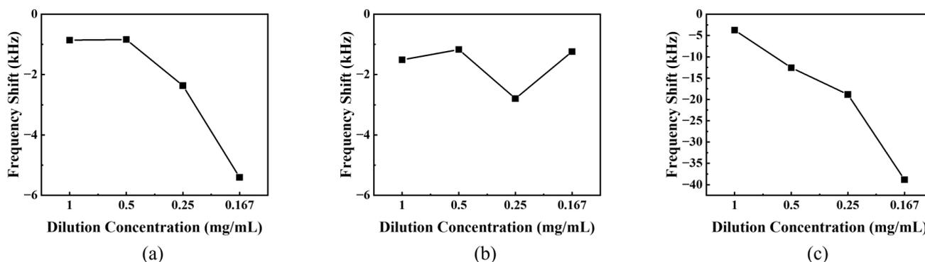
**Figure 7.** Maximum frequency shift according to DMMP response from SAW sensor according to coating concentration of sensing material: (a) PSS-TU1, (b) PSS-TU2, (c) PSS-TU3.
