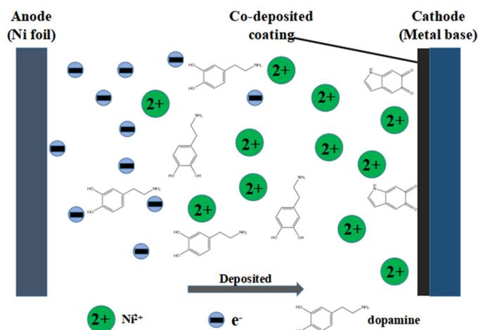
**Figure 1.** Schematic diagram for fabrication of PDA coating by one-step electrodeposition.
