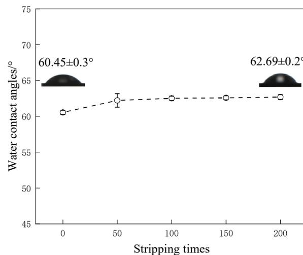
**Figure 5.** Evolution of water contact angle of PDA coating vs. stripping times.
