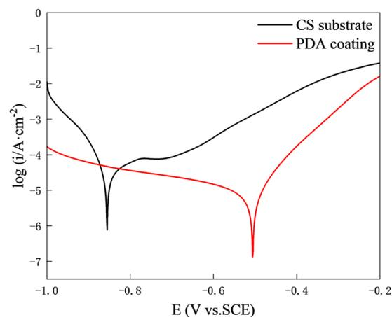
**Figure 6.** Potentiodynamic polarization curves of carbon steel (CS) and PDA coating in 3.5 wt.% NaCl solution.
