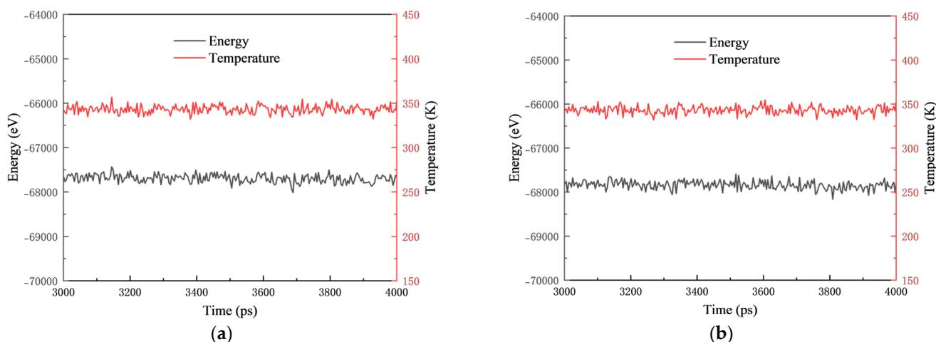
**Figure 3.** Evolution of system temperature and energy for (a) Fe plate and (b) PDA coating.
