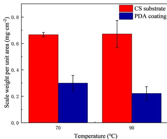
**Figure 7.** Comparison of  $\text{CaCO}_3$  scale deposition on carbon steel (CS) and PDA coating surface.
