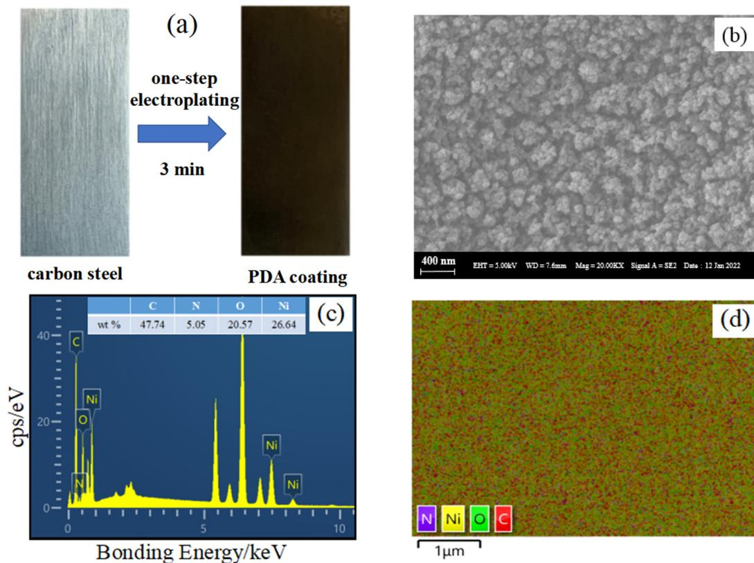
**Figure 4.** (a) Image of carbon steel and PDA-Ni coating, and (b) SEM-, (c) EDS-, and (d) EDS-layered image for PDA coating.
