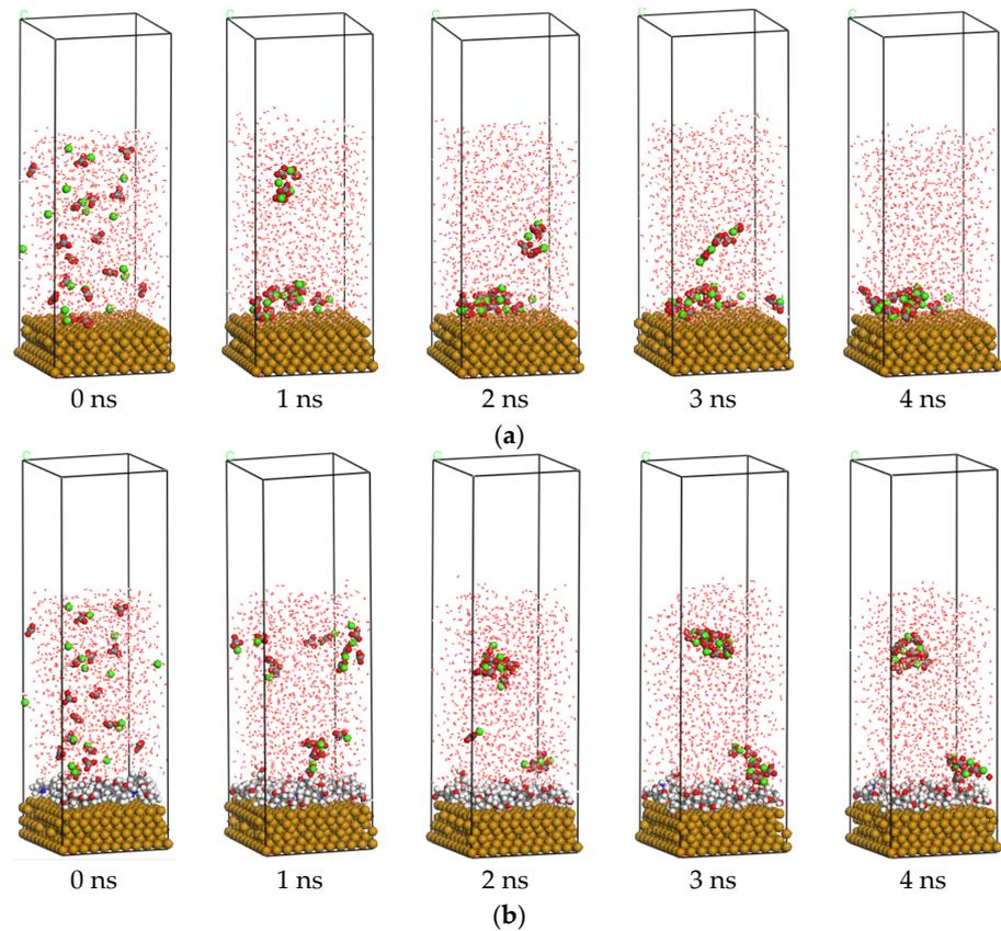
**Figure 8.** Adsorption configurations of  $\text{CaCO}_3$  on (a) Fe plate and (b) PDA coating.
