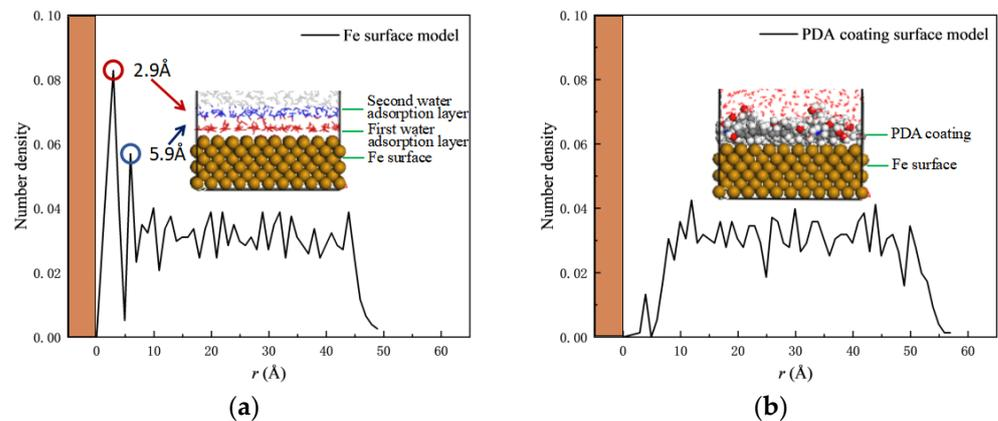
**Figure 9.** Number density distribution of water molecules oriented perpendicular to the surface. (a) Fe plate and (b) PDA coating, brown area is Fe plate.
