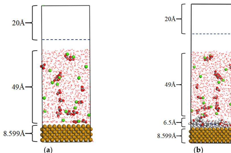
**Figure 2.** Initial simulation system: (a) Fe plate and (b) Fe plate with PDA coating.
