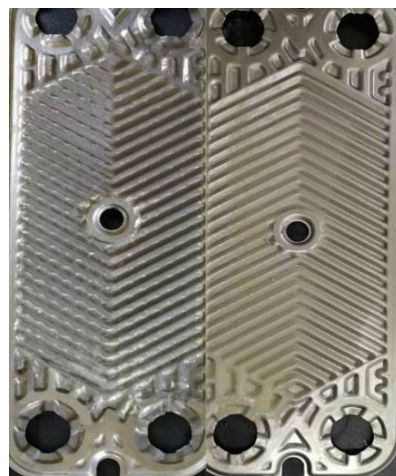
Figure 11. Macroscopic topography of the Ni-P-TiO 2 composite coating (left) and 316 stainless steel (right) at the MgO solution concentration is 400 mg/L.
