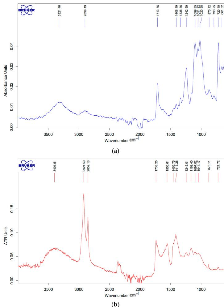
**Figure 7.** ATR FTIR spectra of the detached fragments showing the different organic and inorganic constituents materials identified in (a) sample 1 and (b) sample 2.
