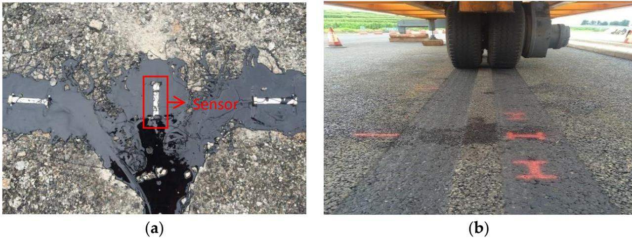
**Figure 6.** Sensor mounting position. (a) Field layout of sensors on the field test road. (b) Location and wiring of the strain gauge.
