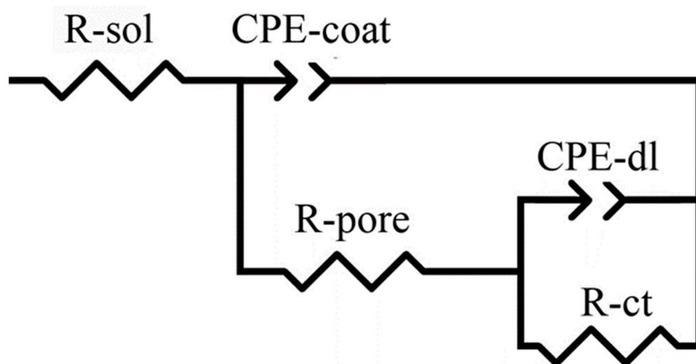
**Figure 3.** Equivalent circuit used for EIS fitting.
