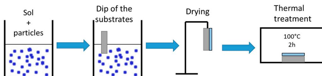
**Figure 1.** Schematic diagram of the coating preparation.
