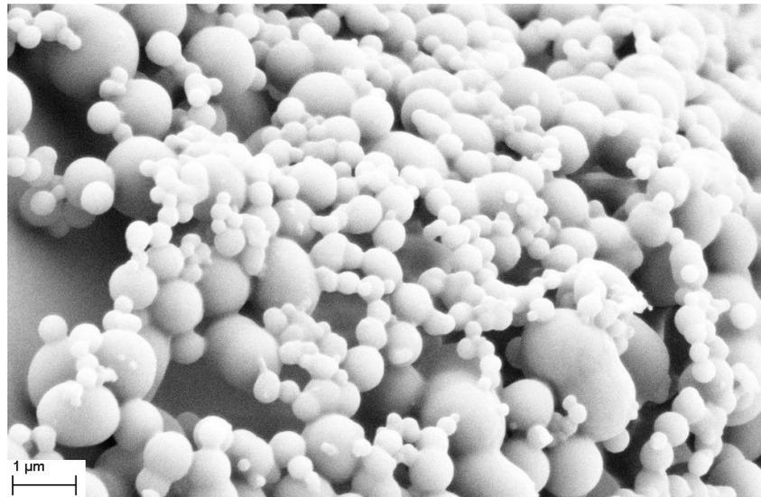
**Figure 4.** SEM micrograph (at 30 kx) of PVA microspheres.
