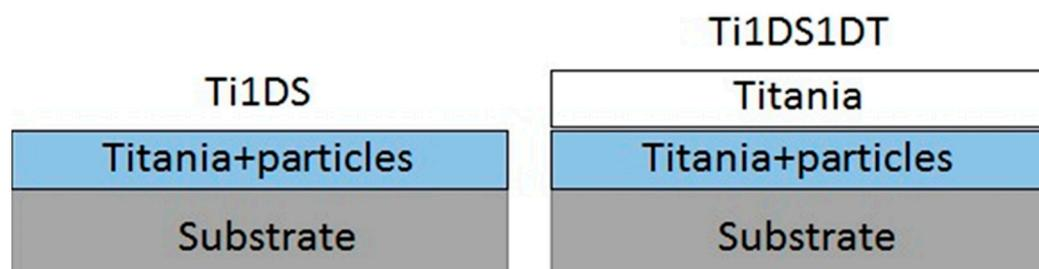
**Figure 2.** The figure shows a schematic diagram of the samples prepared.
