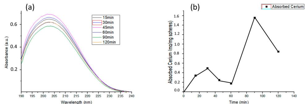
**Figure 7.** The figures show the behaviour of the Ce solution with spheres at different times. (a) Shows the UV spectra for the different immersion times; (b) shows instead the average absorption of molecules for each time.
