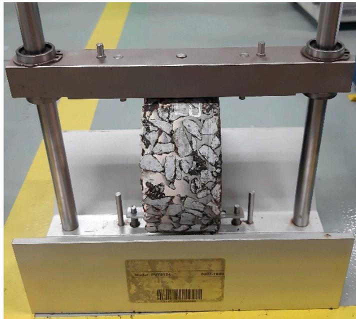
**Figure 3.** Positioning rig for positioning and gluing the deformation strips on the specimen.
