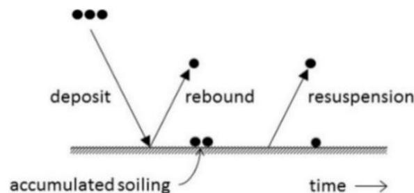
**Figure 3.** The behaviors of dust particles on PV modules [28].
