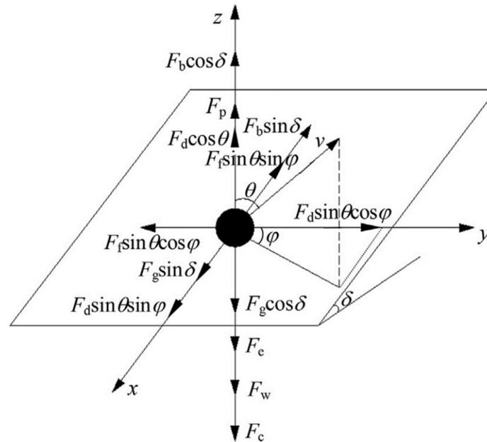
Figure 4. Schematic diagram of particle forces acting on an inclined plate [32].
