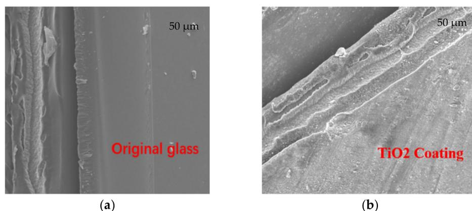
**Figure 9.** SEM images of super-hydrophilic  $TiO_2$  coating [81]. (a) Original solar glass; (b) Solar glass with  $TiO_2$  coating.
