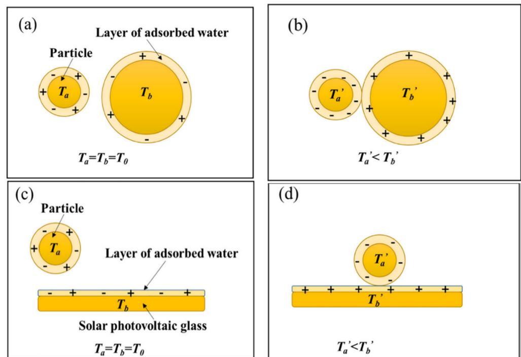
**Figure 8.** Schematic diagram of solar panels and charged particles [65]. (a,b) The temperature change process of particle to particle collision; (c,d) The temperature change process after a particle collides with a rough glass panel.
