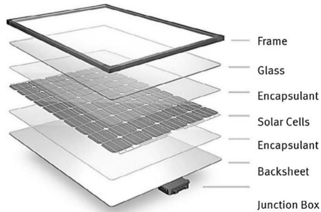
**Figure 1.** The components of a solar panel [16].
