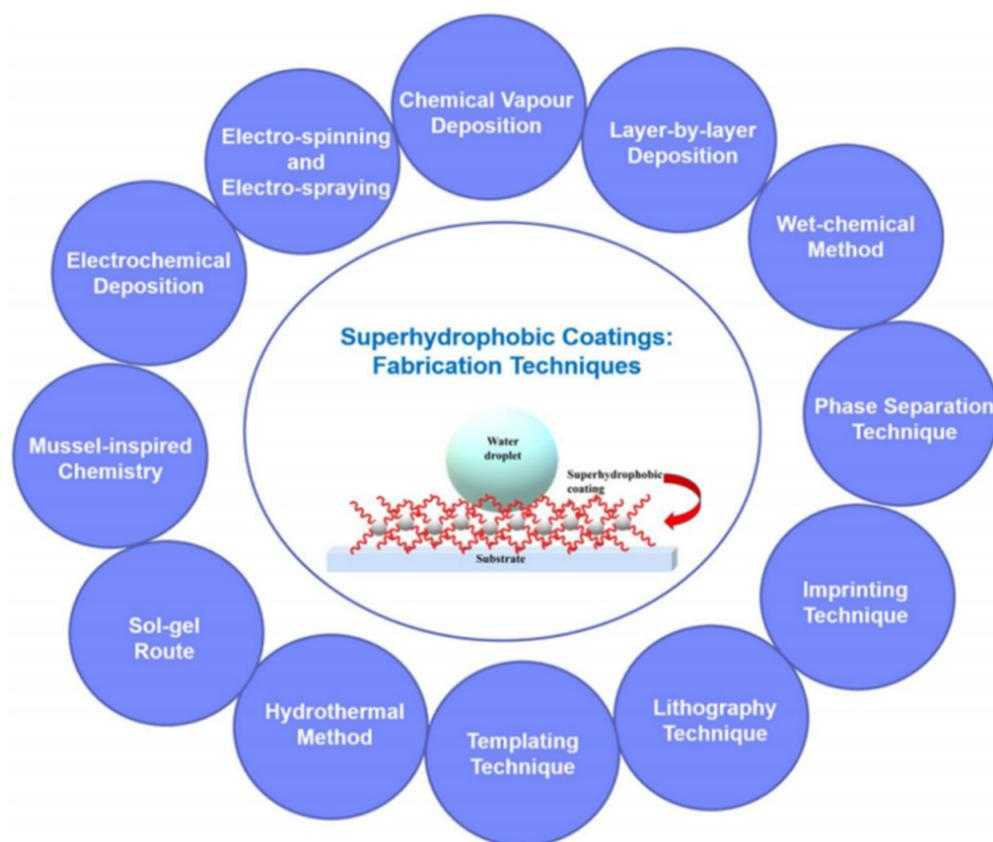
**Figure 11.** The schematic diagram of multiple superhydrophobic coating manufacturing methods [103].
