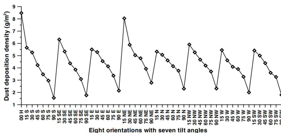
**Figure 7.** Exposure of glass samples to seven tilted angles and eight different orientations of the experimental setup [10].
