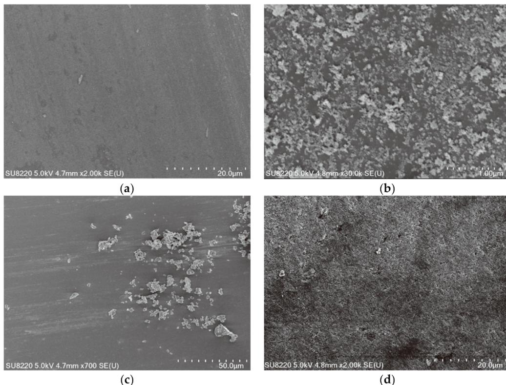
**Figure 10.** SEM images of the glass surfaces without/with super-hydrophobic coating before/after dust deposition [100]. (a) Glass without super-hydrophobic coating before dust deposition; (b) Glass with super-hydrophobic coating before dust deposition; (c) Glass without super-hydrophobic coating after dust deposition; (d) Glass with super-hydrophobic coating after dust deposition.
