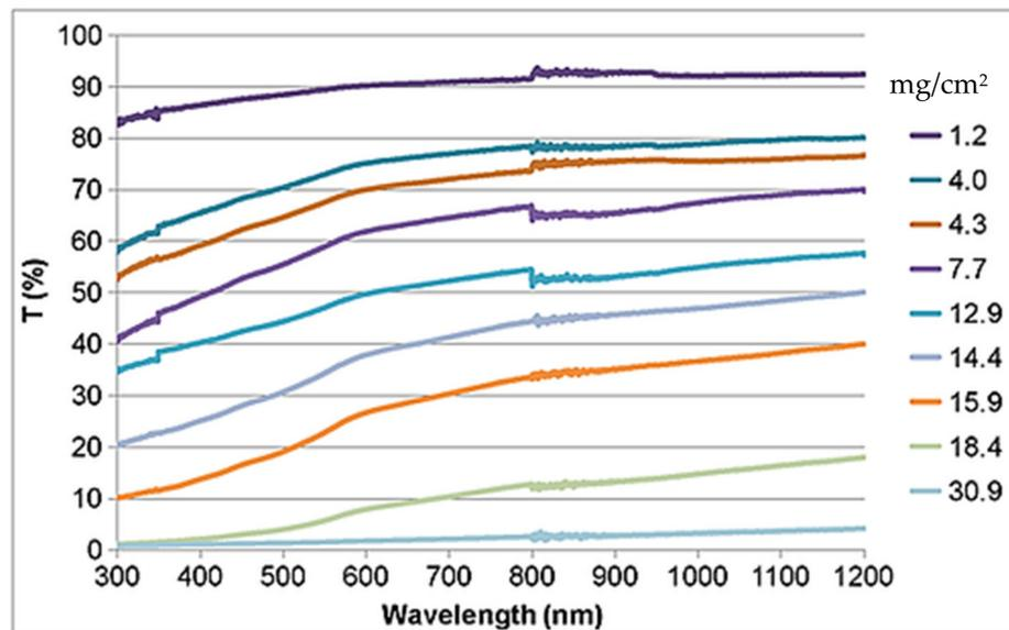
Figure 6. Influence of deposition density on transmittance [54].
