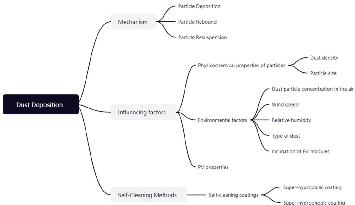
**Figure 12.** A flow chart that explains the dust deposition mechanism, influencing factors, and self-cleaning methods.
