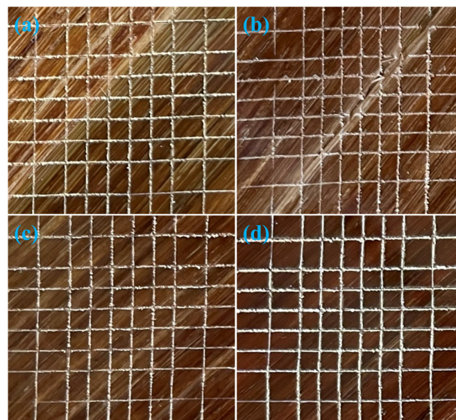
Figure 8. WBV-coated surfaces of bamboo scrimbers with different resin contents: (a) 9%, (b) 11%, (c) 13% and (d) 15%.
