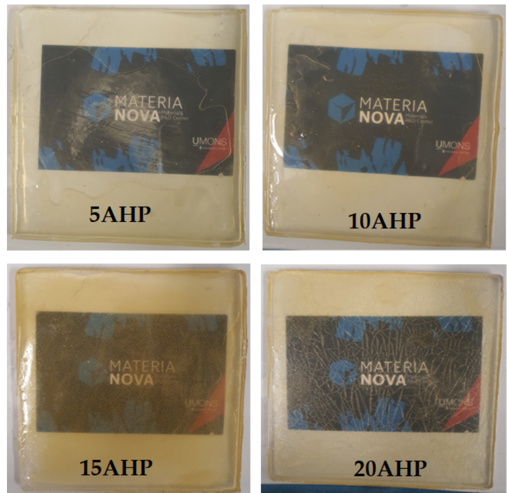
Figure 6. PLA plates surface coated with epoxy/AHP nanocomposite films containing 5, 10, 15 and 20 wt.% AHP nanoparticles.
