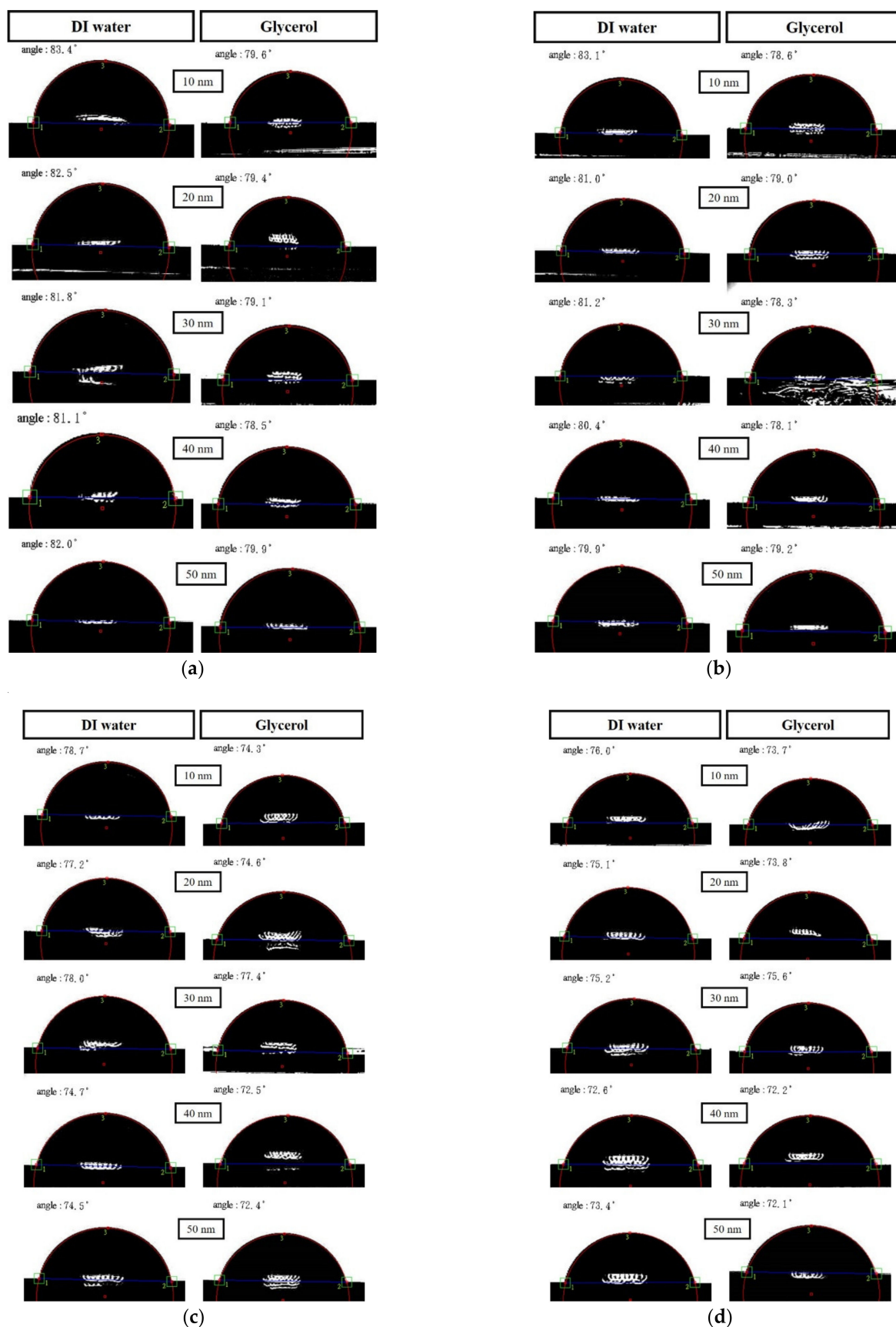
Figure 6. Contact angles of the CoFeY following four situations: (a) RT, (b) after annealing at 100 °C, (c) after annealing at 200 °C, and (d) after annealing at 300 °C.
