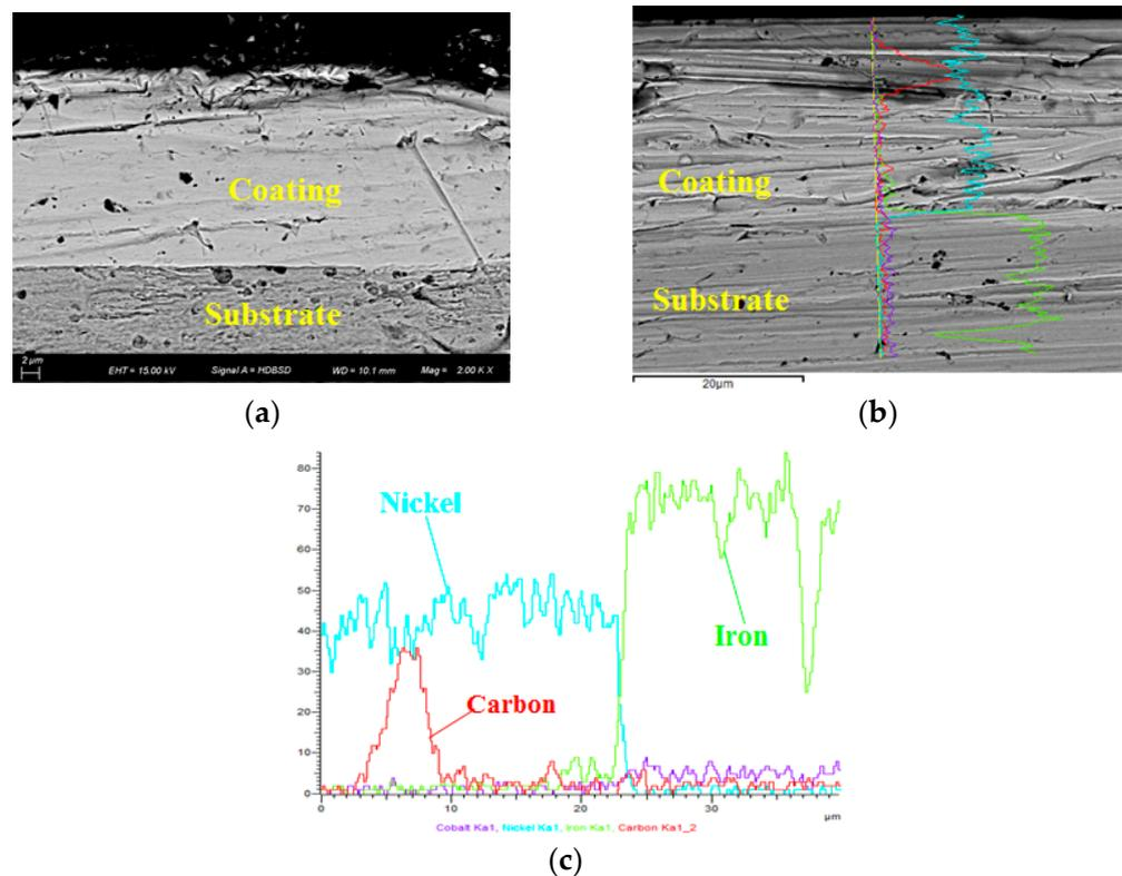
**Figure 2.** Cross-sectional image of the plating: (a) chemically etched cross section, (b) cross section before chemical etching and (c) analysis of cross-sectional elements at different depths.
