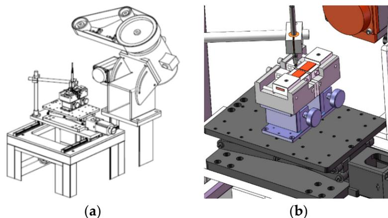
**Figure 6.** Schematic diagram of the friction tester measuring wear in situ: (a) schematic diagram of the complete appearance of the friction tester; (b) local enlargement of in situ measurement.
