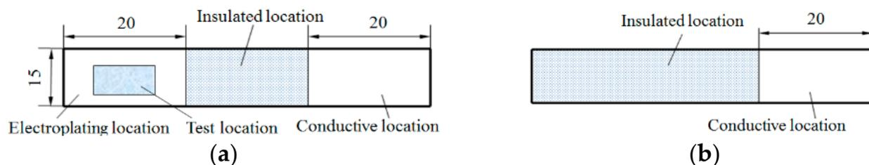
**Figure 1.** Schematic diagram of the matrix size of the substrate and the sealing, plating and conductive locations: (a) front view and (b) back-face view.
