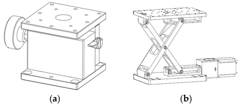
**Figure 9.** Height lift adjustment mechanism: (a) manual operation and (b) electric controls.
