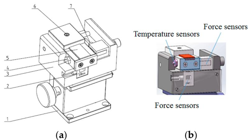
**Figure 8.** Adjustable precision measuring stage and sample-loading mechanism: (a) overall view and (b) partial enlargement. 1—manual fine adjustment of the lift; 2,7—force sensors; 3—sample-loading mechanism; 4—temperature sensors; 5—samples tested; 6—fastening screws.
