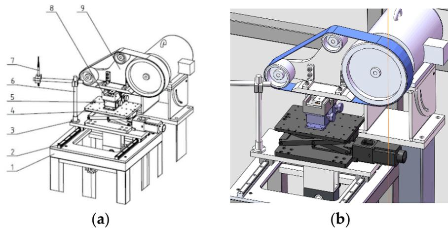
**Figure 5.** Schematic diagram of the friction test process of the test machine: (a) diagram of the complete friction-testing machine; (b) partial enlargement of the friction tester. 1—base; 2—guideway; 3—precision bearing; 4—table for the sample to be tested; 5—lifting mechanism; 6—spindle; 7—probe; 8—clamping mechanism; 9—belt grinding mechanism.
