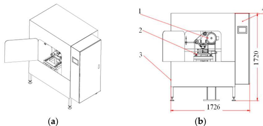
**Figure 4.** Schematic diagram of the appearance of the frictional wear test equipment: (a) axonometric projection view of the appearance of the friction tester; (b) a front-view projection of the appearance of the friction tester. 1—grinding mechanism; 2—table for the sample to be tested; 3—outer cover of the tester; 4—control systems for equipment.
