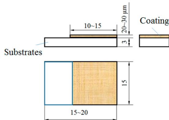
**Figure 7.** Specification of the sample under test and the dimensions of the surface film.
