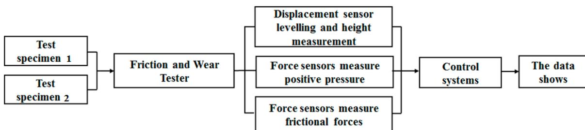
**Figure 12.** Experimental flow diagram of the new friction and wear tester.
