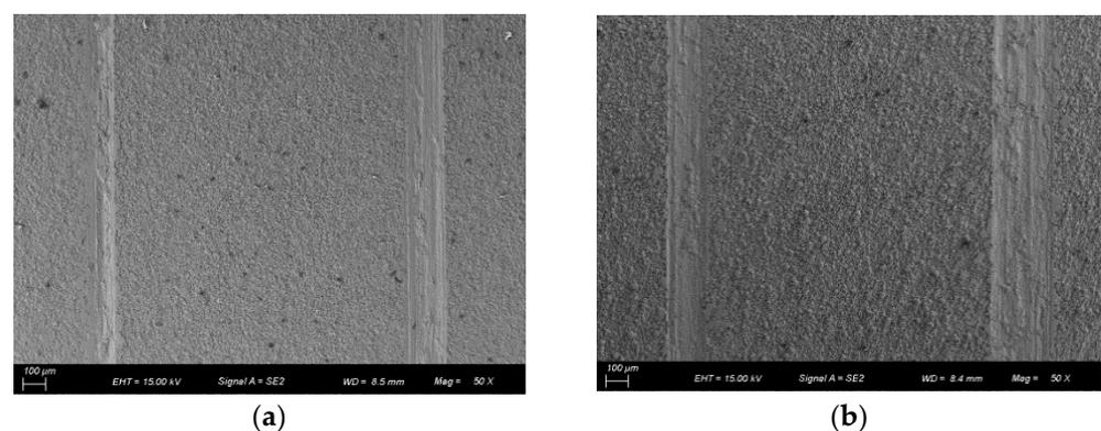
**Figure 3.** Frictional morphology of the composite coating prepared under two different electrodeposition conditions: (a) Sample 1 and (b) Sample 2.
