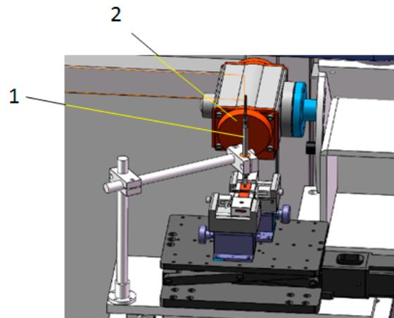
**Figure 11.** Schematic diagram of the height measurement of the sample under test. 1—displacement sensors; 2—data-acquisition equipment.
