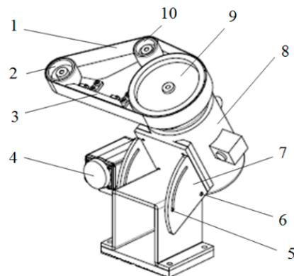
**Figure 10.** Axonometric view of the belt grinding mechanism. 1—sanding belts; 2,9,10—sanding belt support wheels; 3—sanding belt support frame; 4—electric motors; 5—guide pins; 6—spindle; 7—support frame for electric motor actuators; 8—electric motor actuators.
