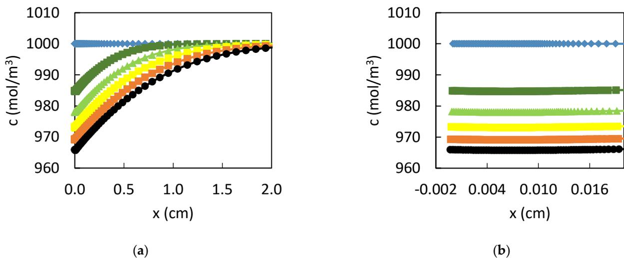
**Figure 14.** Evolution of the chloride ion concentration in an electrolyte of  $1000 \text{ mol/m}^3$  HCl and of size  $L = 10 \text{ cm}$  with an initial CPL of  $100 \text{ }\mu\text{m}$  and a variable porosity (a) the first 2 cm and (b) the first 200  $\mu\text{m}$  of the electrolyte are presented for different times  $t = 0$  (light blue), 3600 (dark green) 7200 s (green), 10,800 s (yellow), 14,400 s (orange), and 18,000 s (black).
