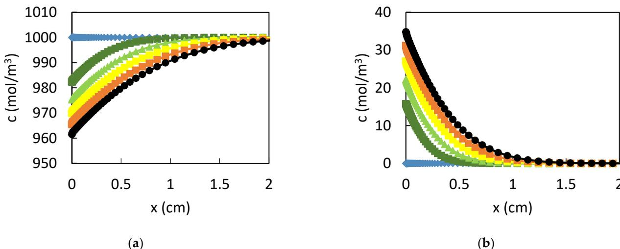
**Figure 10.** Evolution of (a) the protons and (b) H<sub>2</sub> concentration in an electrolyte of 1000 mol/m<sup>3</sup> HCl and of size L = 10 cm with an initial CPL of 100 μm and a fixed porosity of 0.9. The first 2 cm of the electrolyte are presented for different times t = 0 s (light blue), 3600 s (dark green) 7200 s (green), 10,800 s (yellow), 14,400 s (orange), and 18,000 s (black).
