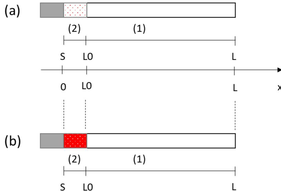
**Figure 4.** Schematic representation of the evolution of the CPL by variation of the porosity over time. The points S, L0 and L are fixed. (a)  $\varepsilon$  at  $t_0$  and (b)  $\varepsilon$  at  $t$ .
