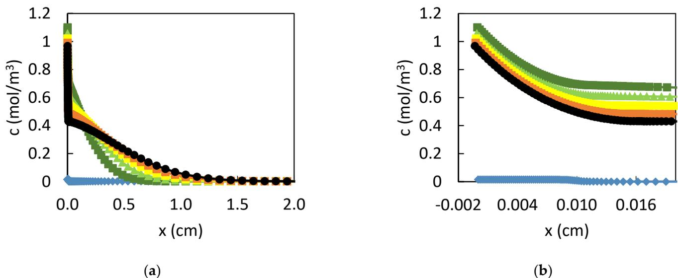
**Figure 8.** Evolution of the lead ion concentration in an electrolyte of  $1000 \text{ mol/m}^3$   $\text{HCl}$  and of size  $L = 10 \text{ cm}$  with an initial CPL of  $100 \text{ }\mu\text{m}$  and a fixed porosity of 0.9 (a) The first 2 cm and (b) the first  $200 \text{ }\mu\text{m}$  of the electrolyte are presented for different times  $t = 0$  (light blue), 3600 (dark green) 7200s (green), 10,800 s (yellow), 14,400 s (orange), and 18,000 s (black).
