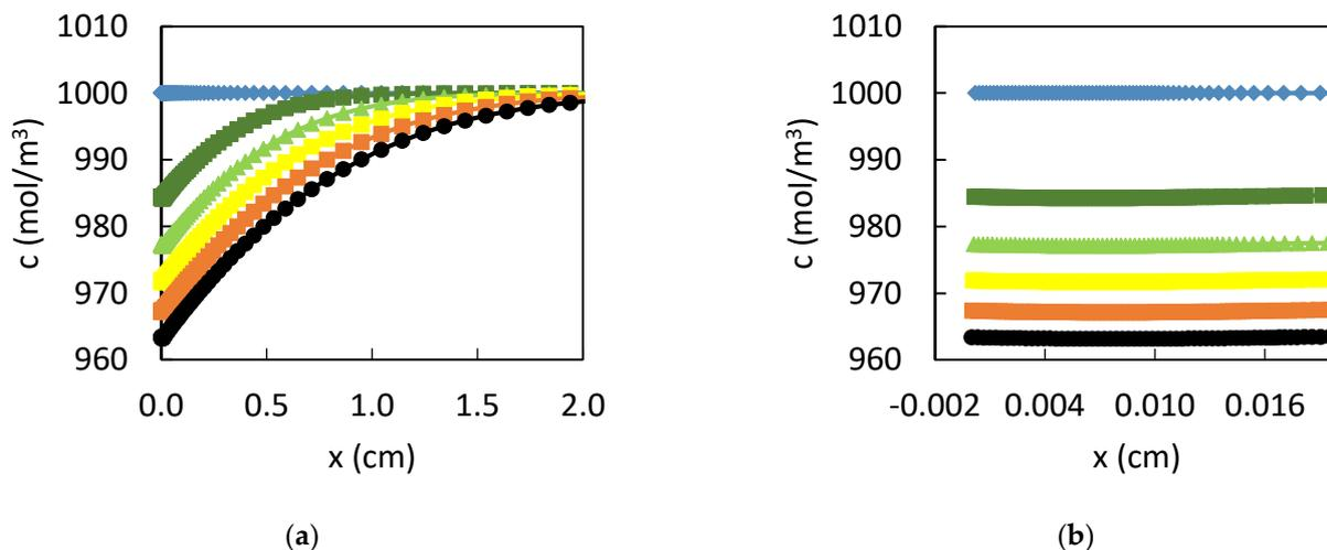
**Figure 9.** Evolution of the chloride ion concentration in an electrolyte of 1000 mol/m<sup>3</sup> HCl and of size L = 10 cm with an initial CPL of 100 μm and a fixed porosity of 0.9 (a) the first 2 cm and (b) the first 200 μm of the electrolyte are presented for different times t = 0 s (light blue), 3600 s (dark green) 7200 s (green), 10,800 s (yellow), 14,400 s (orange), and 18,000 s (black).
