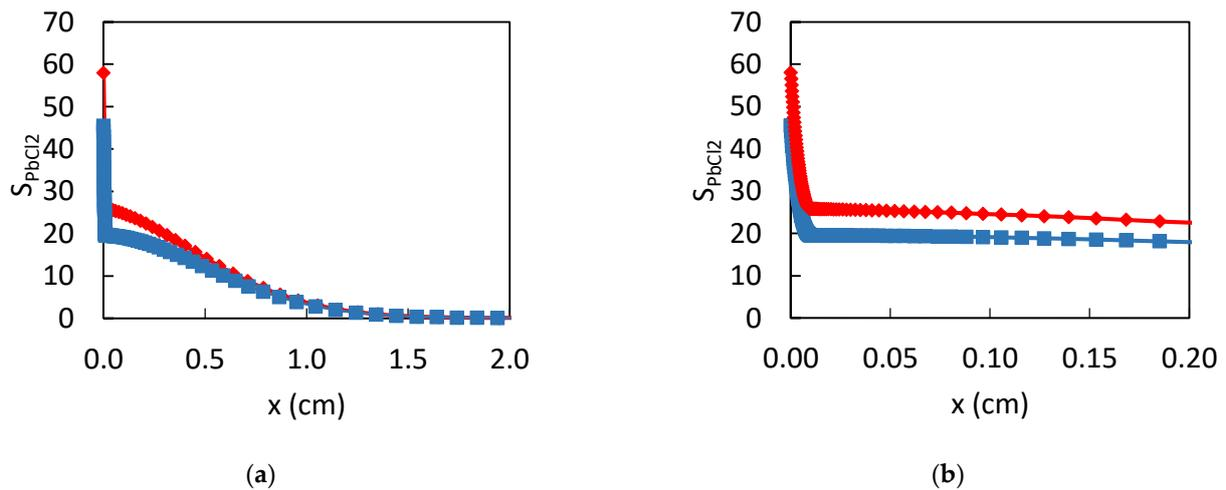
**Figure 16.** Evolution of  $S_{PbCl_2}$  (a) on the first 2 cm and (b) on the first 200  $\mu\text{m}$  of the electrolyte, for (blue) the fixed porosity case and (red) the variable porosity case.
