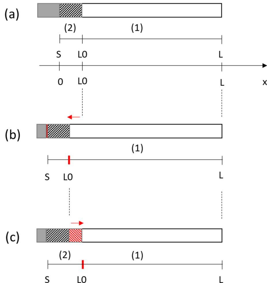
**Figure 3.** Schematic representation of the movement of the CPL corrosion product layer (domain (2)) of size  $x = L_0$ . (a) At  $t_0$ , (b) evolution during dissolution of the lead electrode and (c) precipitation of  $PbCl_2$ .
