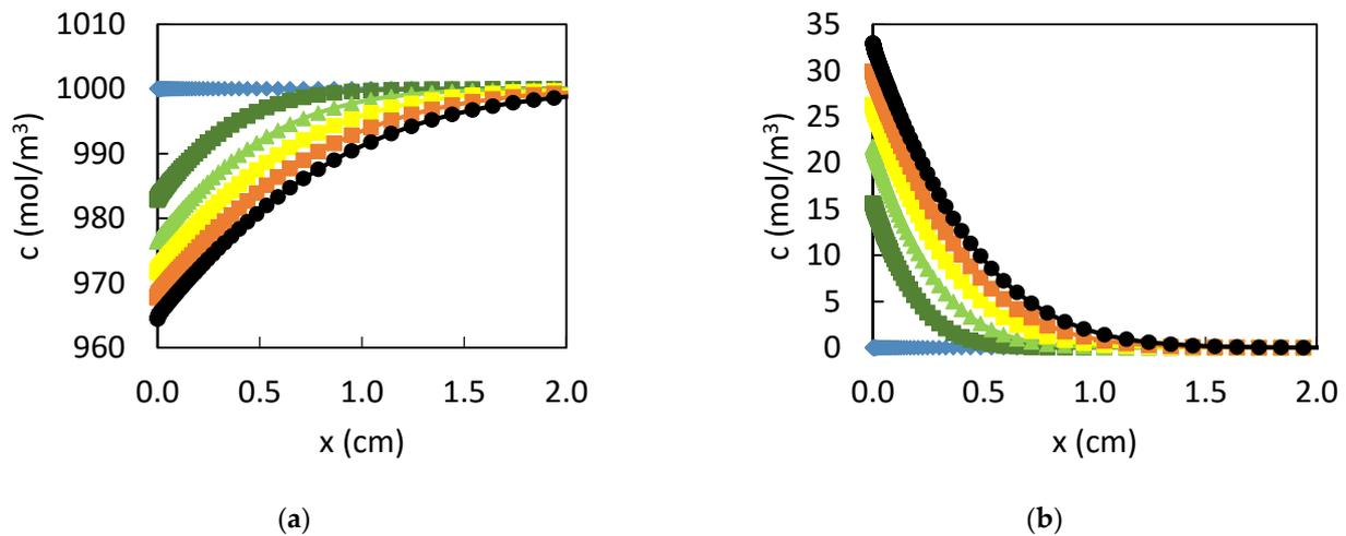
**Figure 15.** Evolution of (a) the protons and (b)  $H_2$  concentration in an electrolyte of  $1000 \text{ mol/m}^3$  HCl and of size  $L = 10 \text{ cm}$  with an initial CPL of  $100 \mu\text{m}$  and a fixed porosity of 0.9. The first 2 cm of the electrolyte are presented for different times  $t = 0 \text{ s}$  (light blue), 3600 s (dark green) 7200 s (green), 10,800 s (yellow), 14,400 s (orange), and 18,000 s (black).
