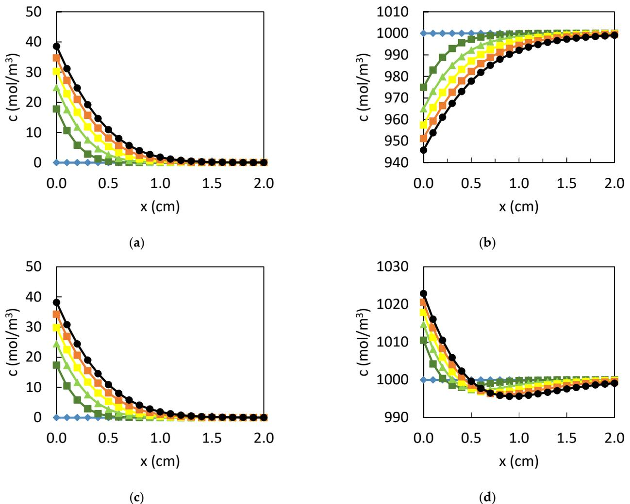
**Figure 6.** Evolution of the ion concentration in an electrolyte of  $1000 \text{ mol/m}^3$  HCl and of size  $L = 10$  cm with only the first 2 cm are presented for six times  $t = 0$  s (light blue), 3600 s (dark green) 7200 s (green), 10,800 s (yellow), 14,400 s (orange), and 18,000 s (black). (a)  $\text{Pb}^{2+}$  ions, (b)  $\text{H}^+$  ions, (c)  $\text{H}_2$  and (d)  $\text{Cl}^-$  ions.
