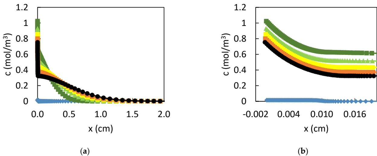
**Figure 13.** Evolution of the lead ion concentration in an electrolyte of  $1000 \text{ mol/m}^3$  HCl and of size  $L = 10 \text{ cm}$  with an initial CPL of  $100 \text{ }\mu\text{m}$  and a variable porosity (a) the first 2 cm and (b) the first 200  $\mu\text{m}$  of the electrolyte are presented for different times  $t = 0$  (light blue), 3600 (dark green) 7200s (green), 10,800 s (yellow), 14,400 s (orange), and 18,000 s (black).
