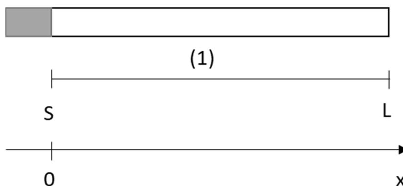
**Figure 1.** Schematic representation of a lead electrode exposed to a deaerated HCl electrolyte. Initially, the thickness of the electrolyte is  $L$  and the surface  $S$  of lead is at  $x = 0$ .
