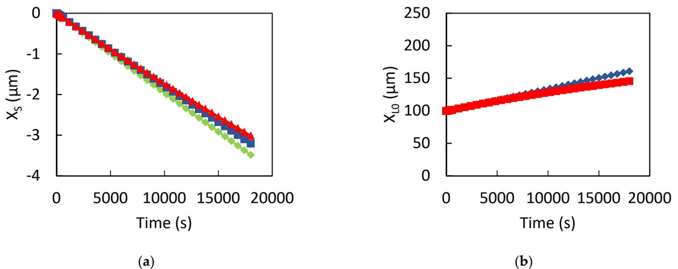
**Figure 7.** Evolution of (a) the position of the electrode surface  $x_s$  ( $\mu\text{m}$ ) and (b) position of CPL electrolyte interface  $x_{L0}$  ( $\mu\text{m}$ ). Simulation with only dissolution (green), a fixed porosity (blue), and a variable porosity (red).
