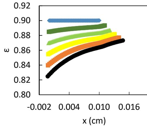
**Figure 11.** Evolution of the porosity of the CPL in an electrolyte of 1000 mol/m<sup>3</sup> HCl of a size L = 10 cm with an initial CPL of 100 μm as a function of time (s) presented for different times t = 0 s (light blue), 3600 s (dark green) 7200 s (green), 10,800 s (yellow), 14,400 s (orange), and 18,000 s (black).
