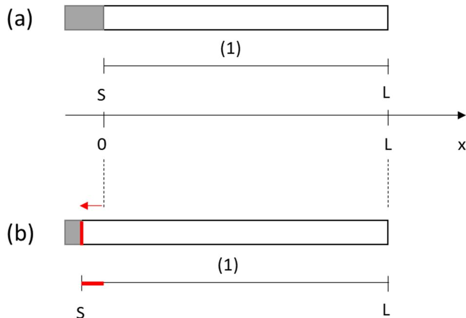
**Figure 2.** Schematic representation of the dissolution of the lead test tube immersed in a deaerated HCl solution. (a) at  $t_0$  and (b) at  $t$ .
