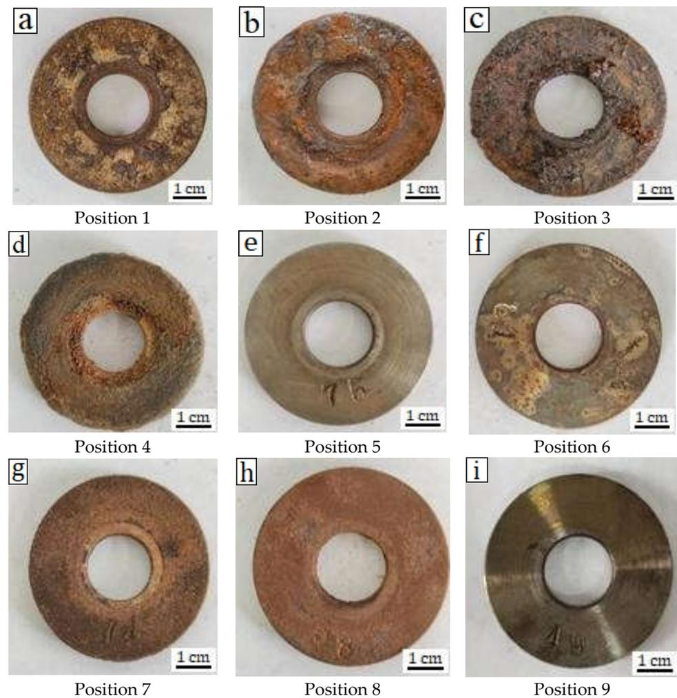
**Figure 2.** Macro-morphology of corrosion hanging ring at each site.
