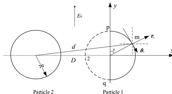
Figure 3. The calculation model for the two-particle system in the longitudinal external electric field.
