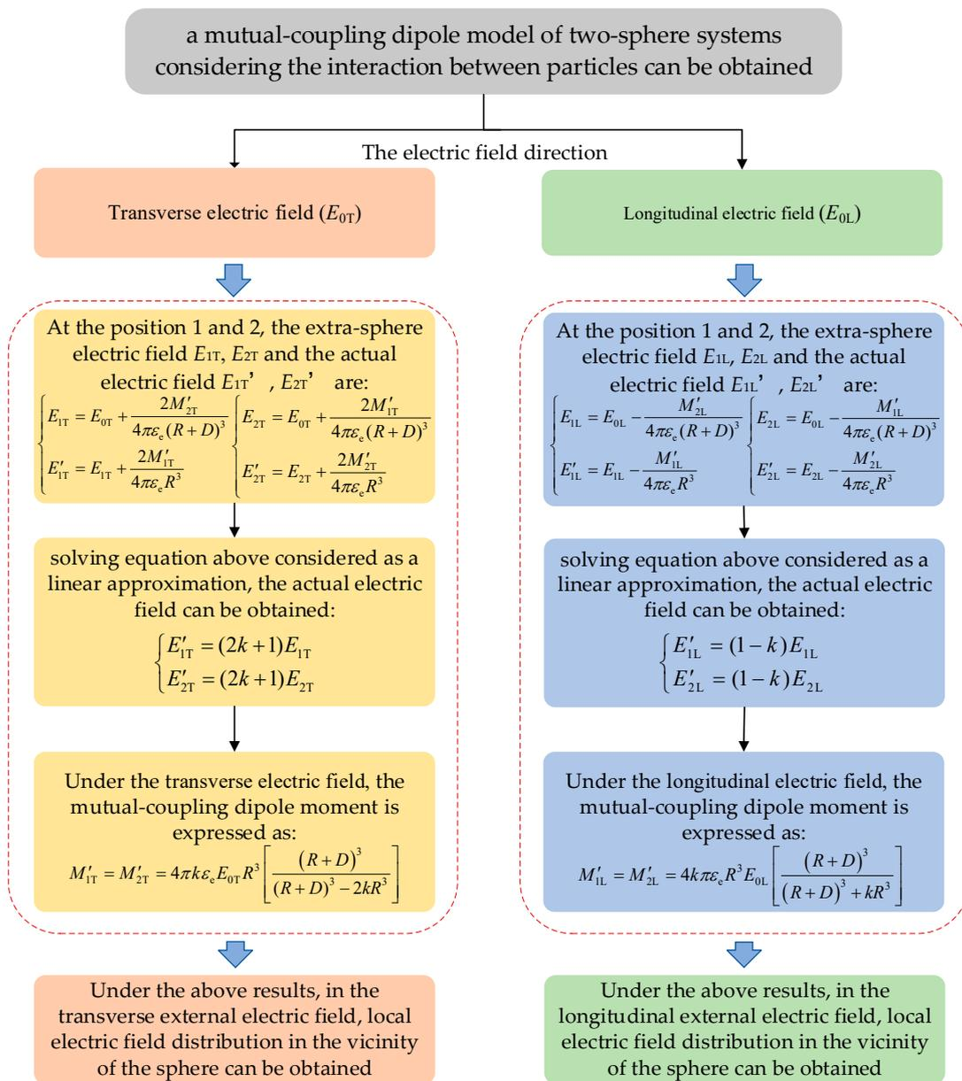
**Figure 4.** The mutual-coupling dipole model for calculating the equations under different scenarios.
