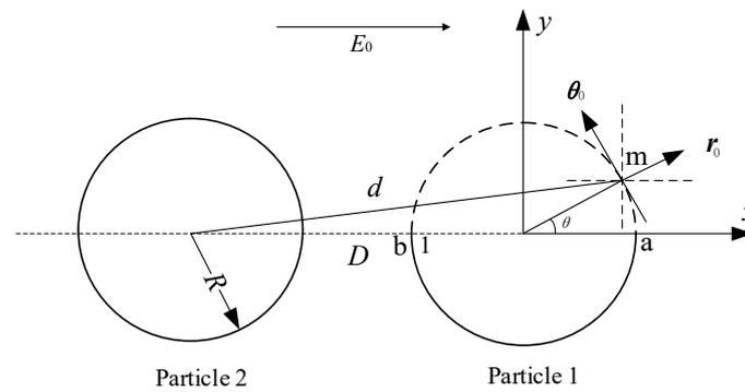
**Figure 2.** The calculation model for the two-particle system in the transverse external electric field.
