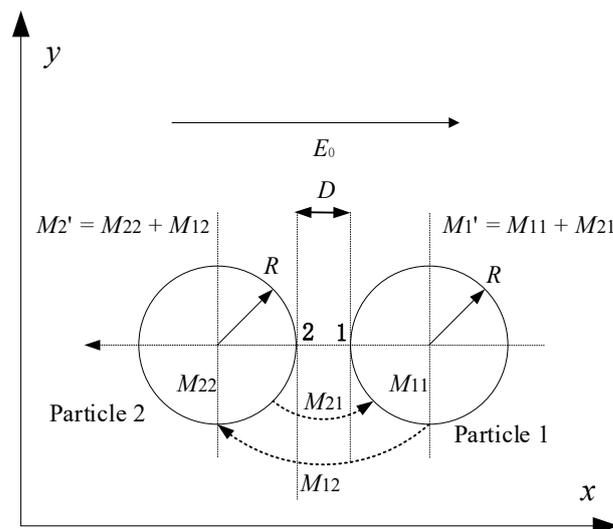
**Figure 1.** A mutual-coupling dipole model in a two-particle system.
