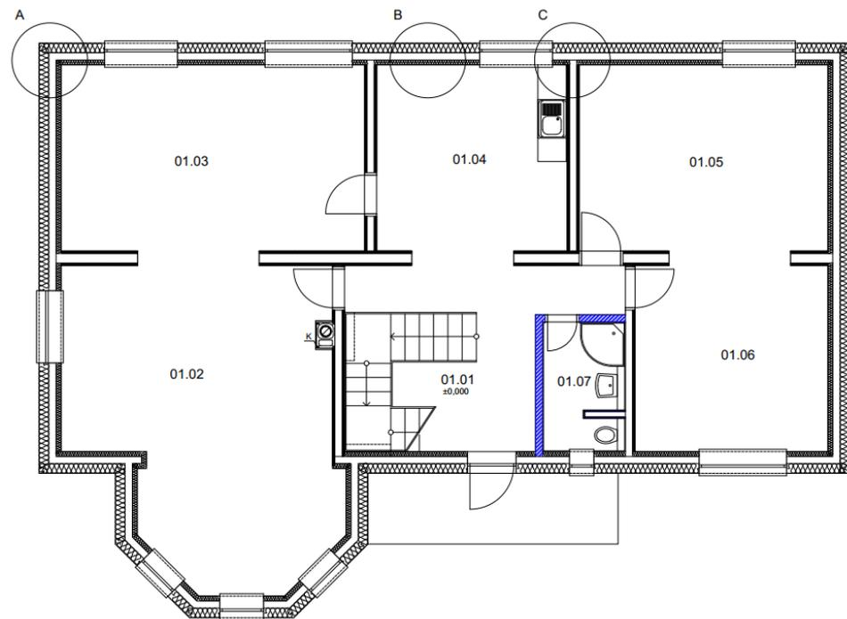
**Figure 9.** First floor plan showing the location of details A, B, and C; K—chimney for fireplace; the digit +0.000 indicates the ground floor elevation.
