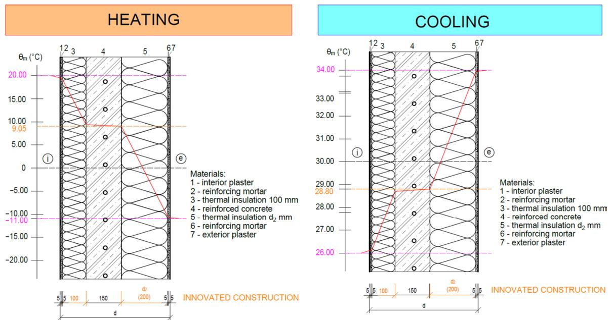
**Figure 8.** Temperatures in individual layers of the upgraded panel, i—interior, e—exterior.
