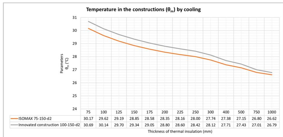
Figure 24. Dependence of the average temperature  $\theta_m$  in the thermal barrier layer of the ISOMAX panel and the innovative panel during the cooling period on the thickness of the external thermal insulation.
