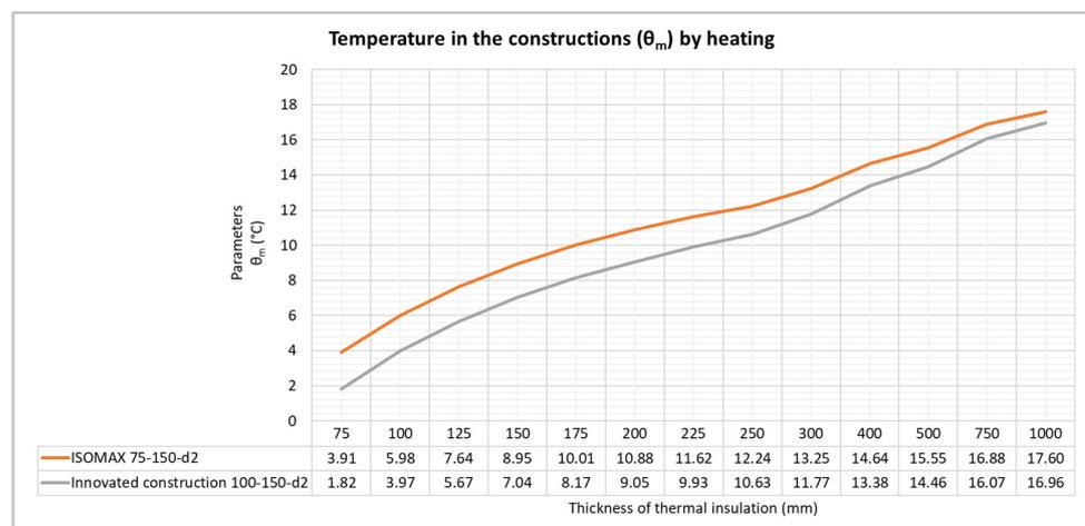
Figure 23. Dependence of the average temperature  $\theta_m$  in the thermal barrier layer of the ISOMAX panel and the innovative panel in the heating period on the thickness of the external thermal insulation.
