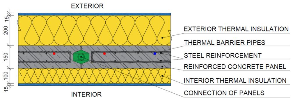
**Figure 12.** “Detail B”, the through joint of two perimeter panels. The colored points (red and blue) in the picture are thermal barrier pipes.
