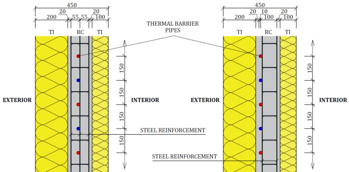
**Figure 19.** Principle of thermal barrier application in innovative panels (left—thermal barrier pipes are installed on the auxiliary reinforcement in the center of the panel structure; right—thermal barrier pipes are installed on the outer reinforcement of the panel structure). The colored points (red and blue) in the picture are thermal barrier pipes [1].
