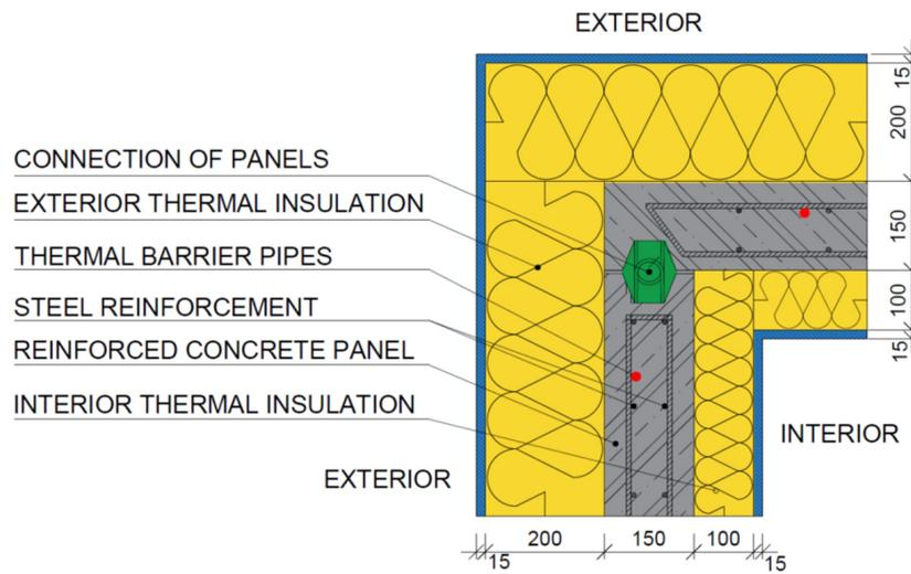
**Figure 11.** “Detail A”, the corner joint of two perimeter panels. The colored points (red) in the picture are thermal barrier pipes.
