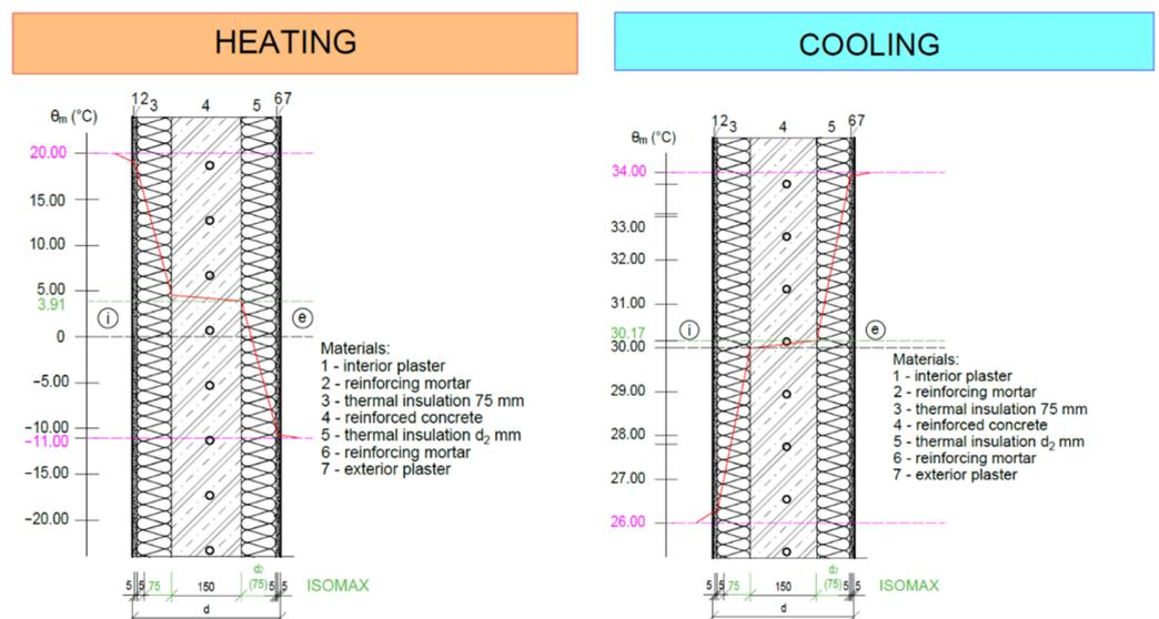
**Figure 5.** Temperatures in individual layers of the ISOMAX panel, i—interior, e—exterior.
