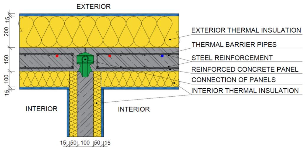
**Figure 13.** “Detail C”, a through joint of two perimeter panels with an internal load-bearing panel. The colored points (red and blue) in the picture are thermal barrier pipes.
