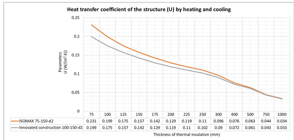
Figure 21. Dependence of the heat transfer coefficient  $U$  of the ISOMAX panel and the innovative panel on the thickness of the external thermal insulation.
