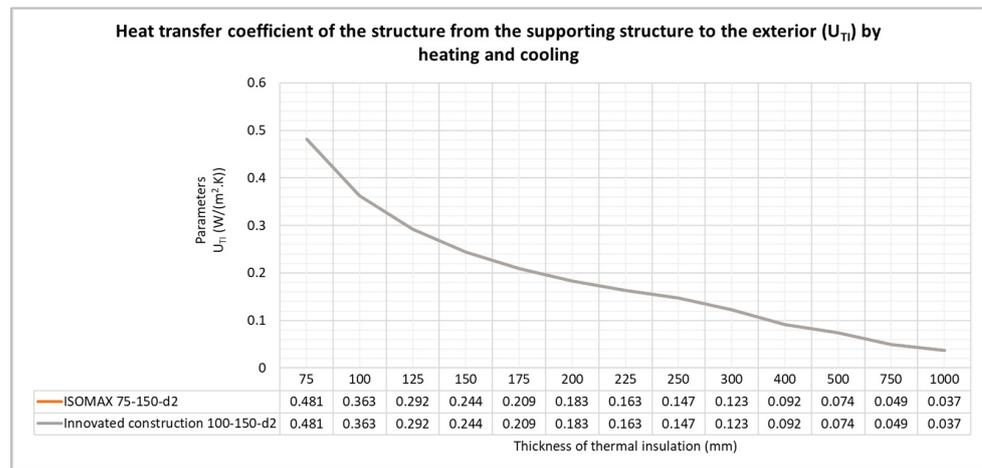
Figure 22. Dependence of the heat transfer coefficient  $U_{TI}$  of the exterior thermal insulation on the thickness.
