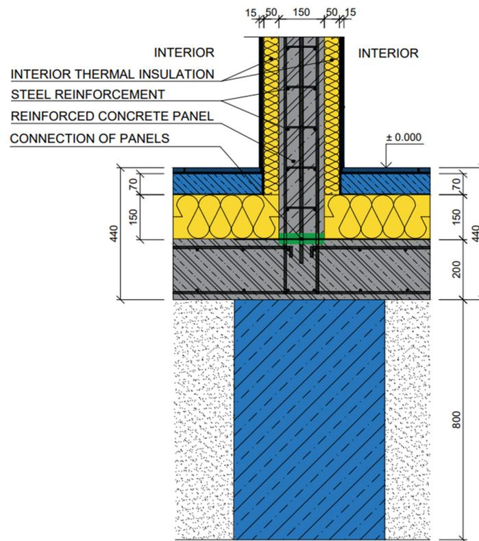
Figure 14. "Detail D", the connection of the inner load-bearing panel to the base plate.
