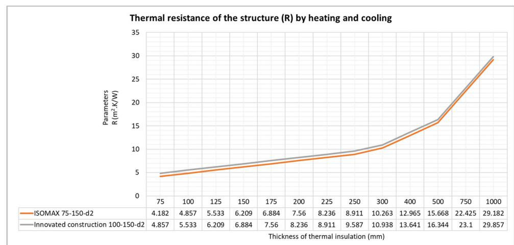
**Figure 20.** Dependence of the thermal resistance  $R$  of the ISOMAX panel and the innovative panel on the thickness of the exterior thermal insulation.
