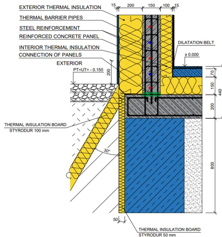
Figure 15. "Detail E", the joint of the perimeter panel with the base plate. The colored points (red and blue) in the picture are thermal barrier pipes.
