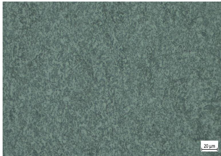
**Figure 1.** Microstructure of normalized GCr15 steel.
