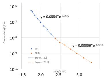
Figure 18. AC conductivity on temperature for the sample GBM 370 at frequency 20 Hz.
