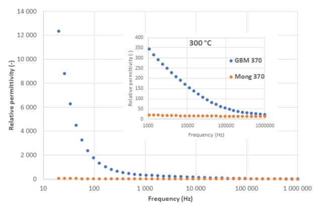
Figure 13. Relative permittivity dependence on frequency at 300 °C for coatings sprayed with SD 370.
