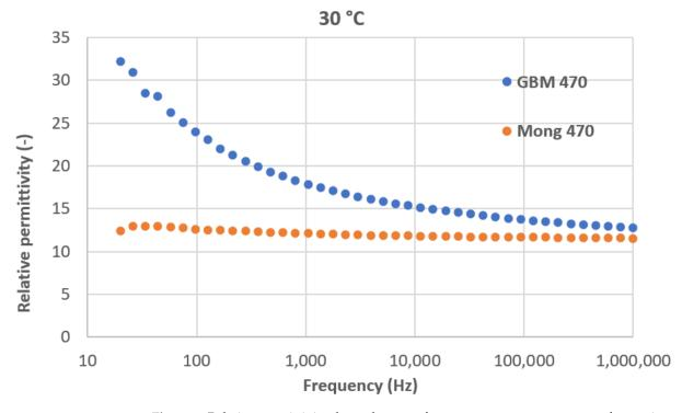
**Figure 9.** Relative permittivity dependence on frequency at room temperature for coatings sprayed with SD 470.
