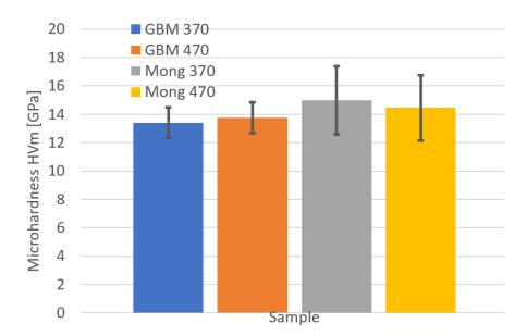
Figure 4. Microhardness of the coatings.
