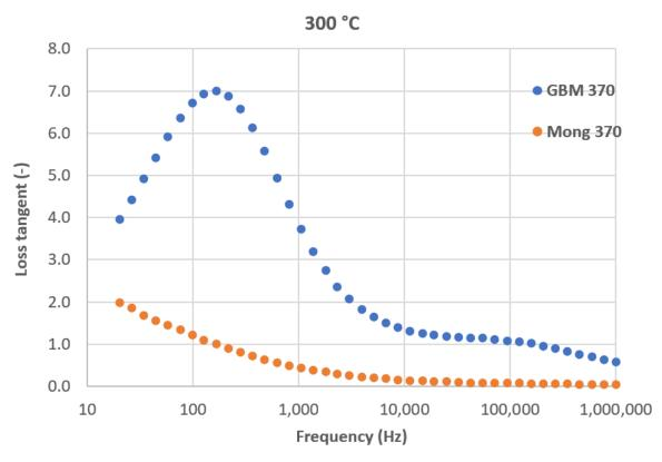
Figure 15. Loss tangent dependence on frequency at 300 °C for coatings sprayed with SD 370.
