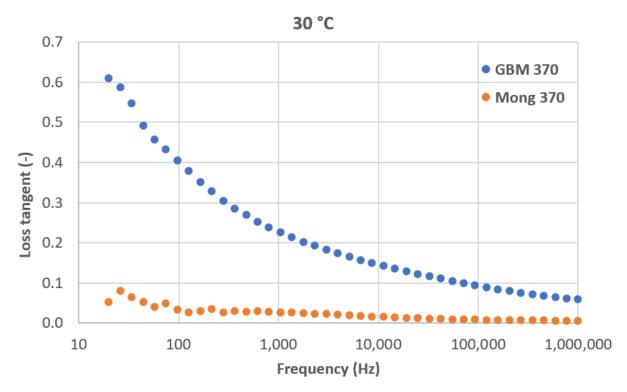
**Figure 10.** Loss tangent dependence on frequency at room temperature for coatings sprayed with SD 370.
