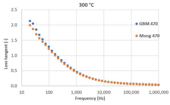
Figure 16. Loss tangent dependence on frequency at 300 °C for coatings sprayed with SD 470.
