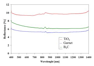
Figure 19. Optical reflectance of the plasma sprayed garnet.
