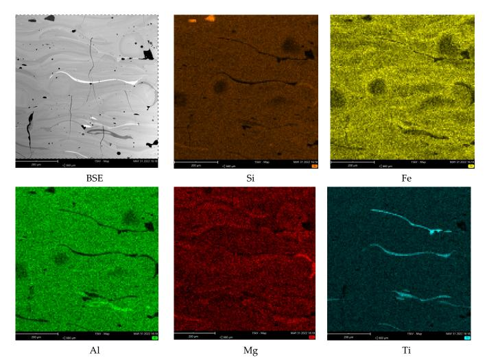
Figure 5. Element mapping of the sample GBM470, polished cross section.
