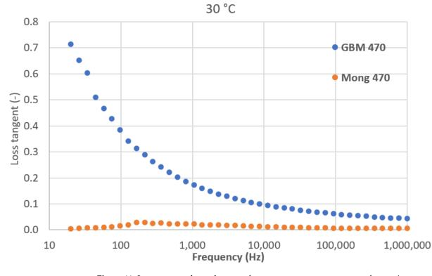
**Figure 11.** Loss tangent dependence on frequency at room temperature for coatings sprayed with SD 470.
