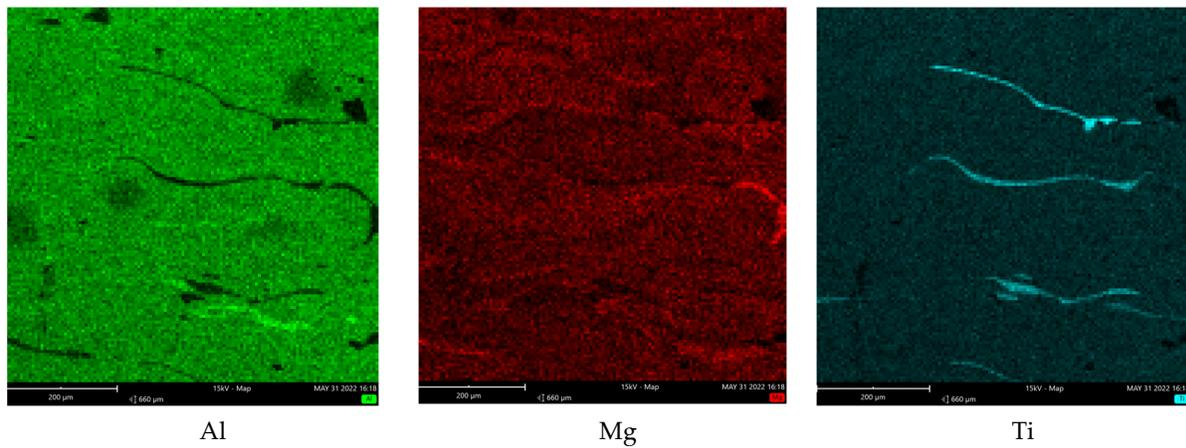
**Figure 5.** Element mapping of the sample GBM470, polished cross section.
