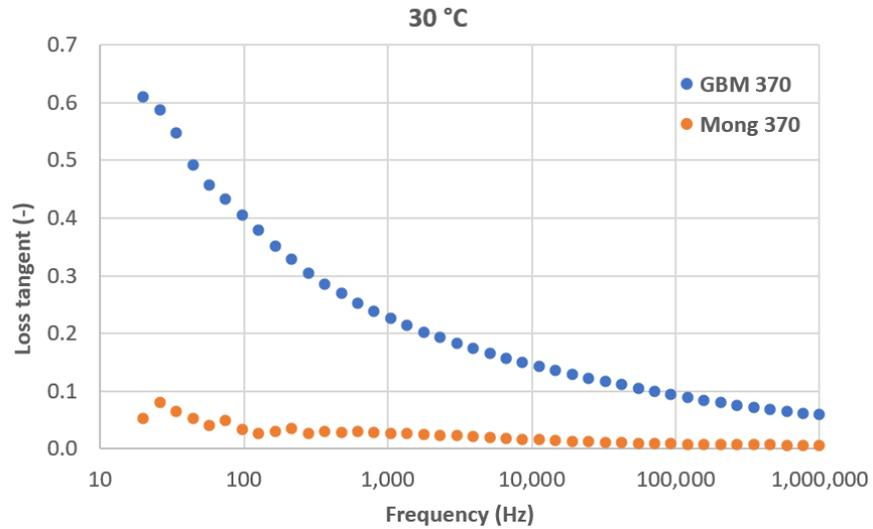
**Figure 10.** Loss tangent dependence on frequency at room temperature for coatings sprayed with SD 370.
