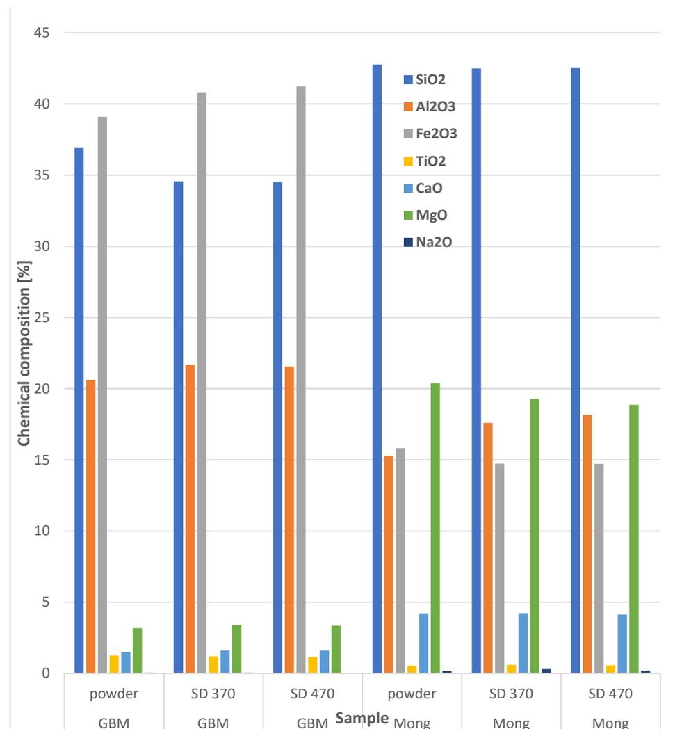
**Figure 12.** Content of individual simple oxides, recalculated from XRF results.
