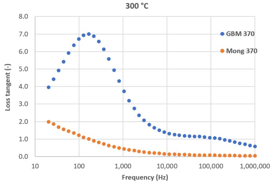
**Figure 15.** Loss tangent dependence on frequency at 300 °C for coatings sprayed with SD 370.
