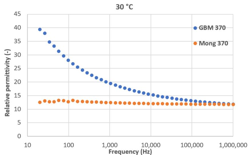
**Figure 8.** Relative permittivity dependence on frequency at room temperature for coatings sprayed with SD 370.
