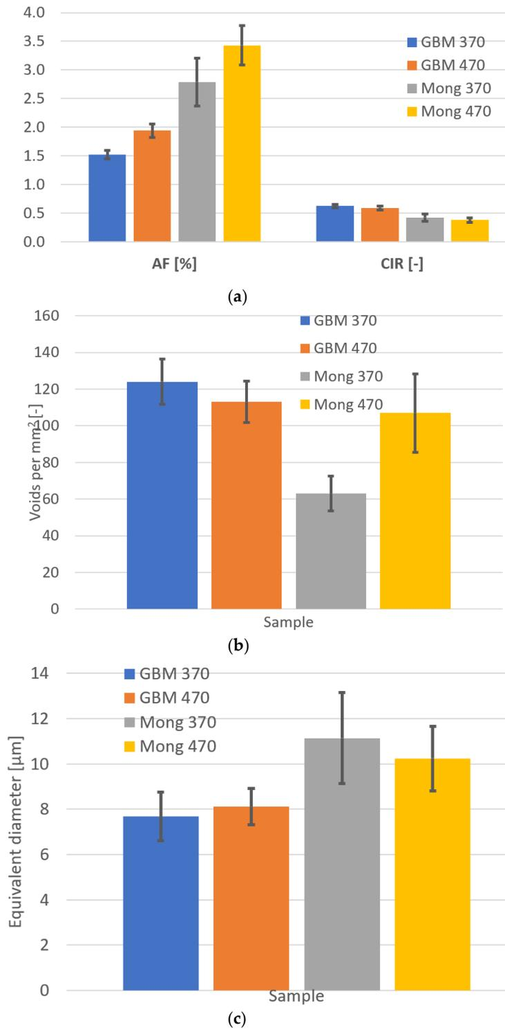
**Figure 3.** (a). Porosity expressed as area fraction AF and circularity of pores CIR. (b). Porosity parameter Voids per mm<sup>2</sup>. (c). Porosity parameter Equivalent diameter of a pore.
