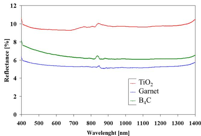
Figure 19. Optical reflectance of the plasma sprayed garnet.
