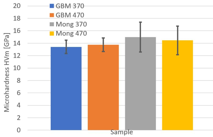
Figure 4. Microhardness of the coatings.
