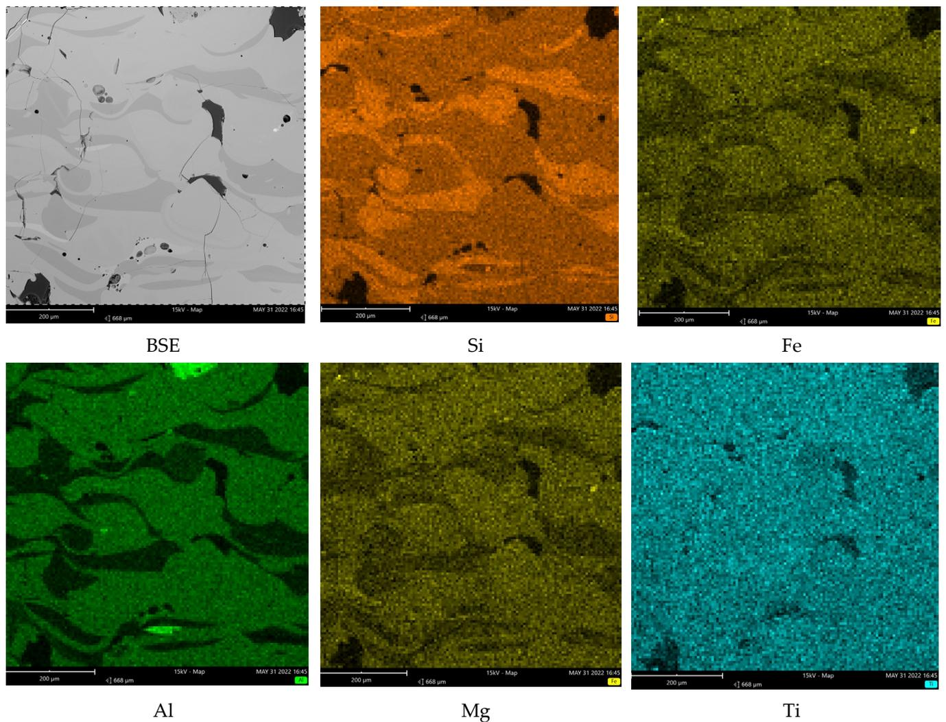
**Figure 6.** Element mapping of the sample Mong470, polished cross section.
