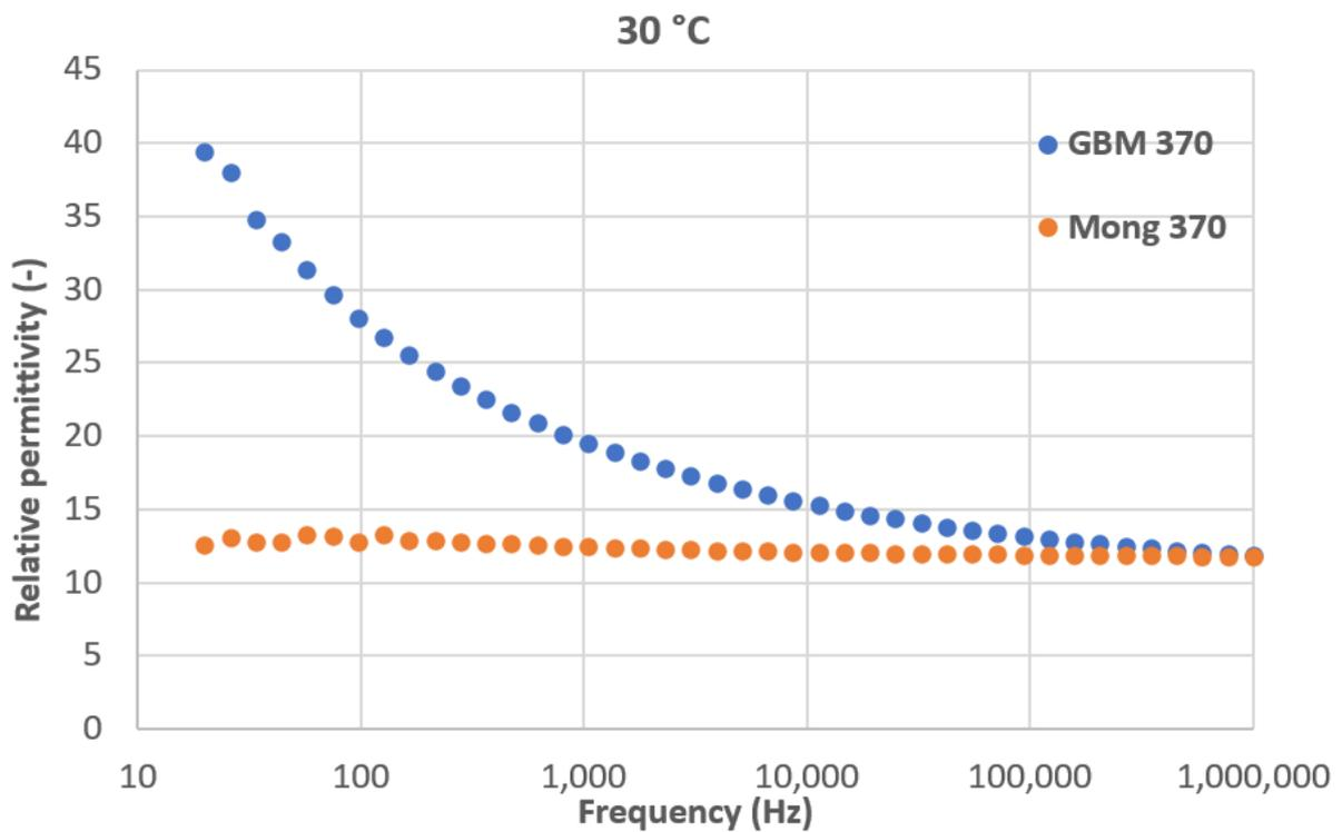
Figure 8. Relative permittivity dependence on frequency at room temperature for coatings sprayed with SD 370.
