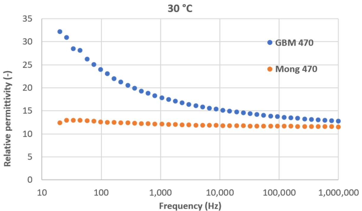
Figure 9. Relative permittivity dependence on frequency at room temperature for coatings sprayed with SD 470.
