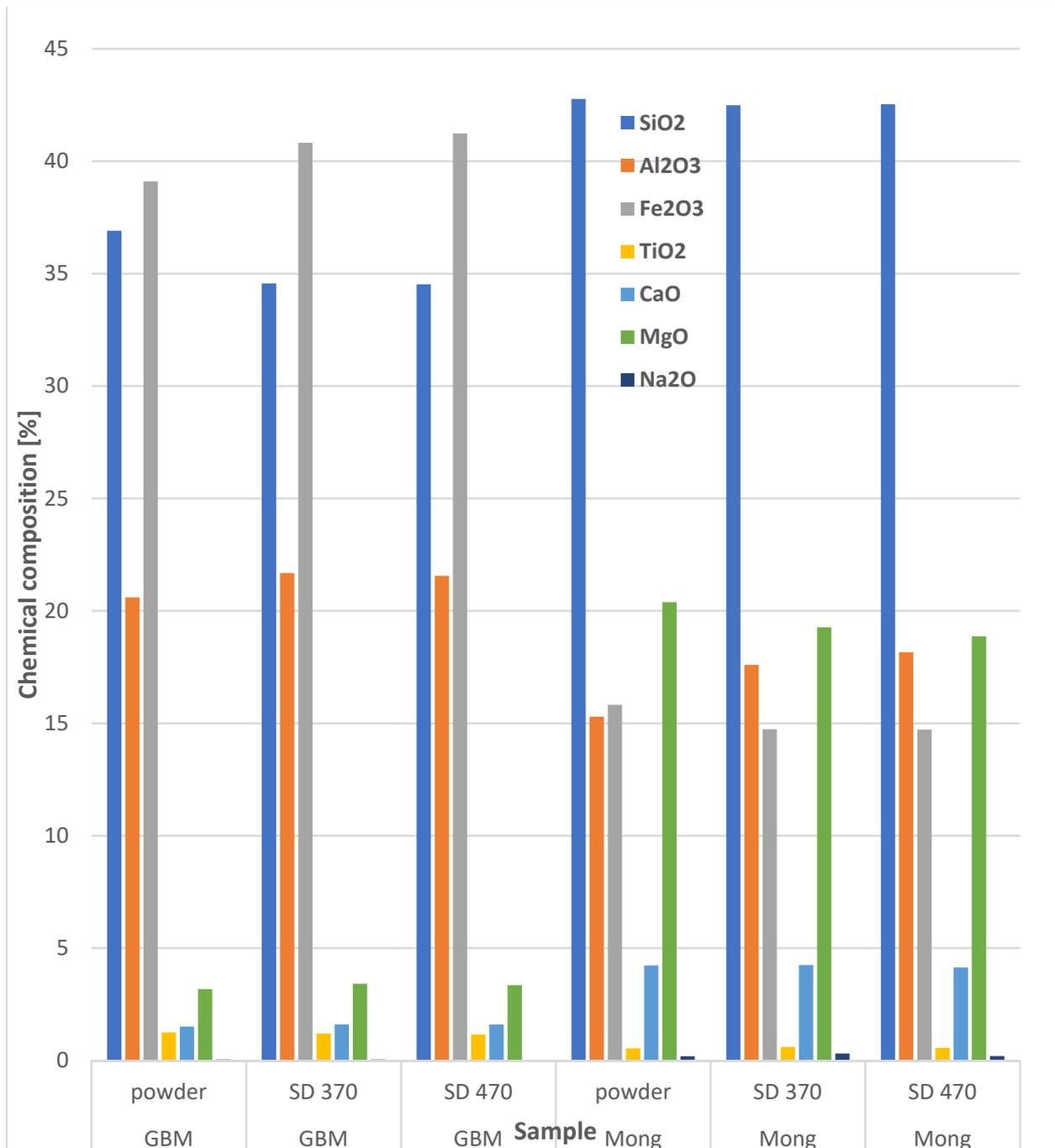
**Figure 12.** Content of individual simple oxides, recalculated from XRF results.
