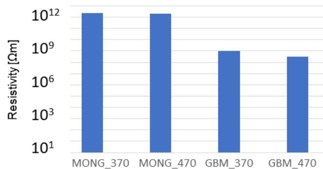
Figure 17. DC volume resistivity of the samples.
