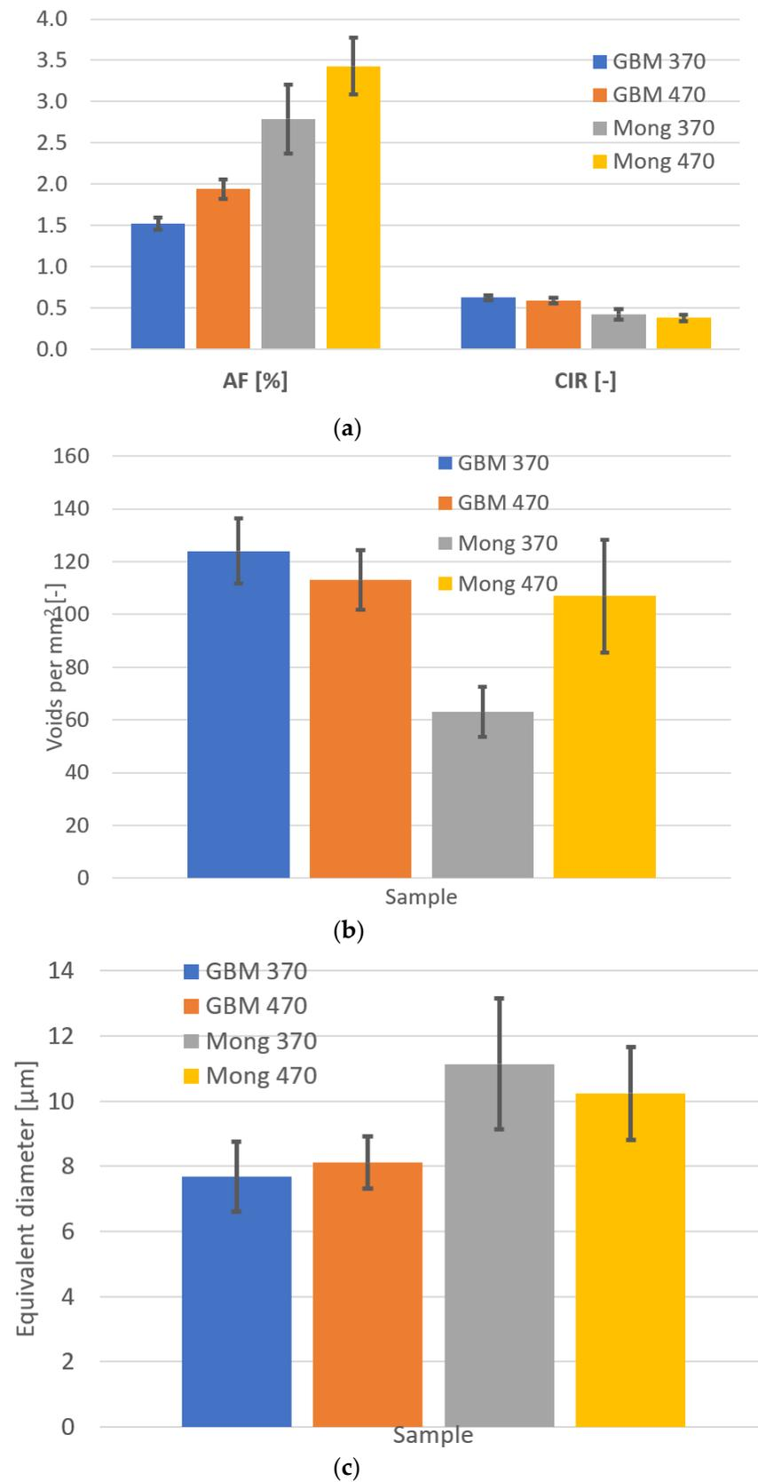
**Figure 3.** (a) Porosity expressed as area fraction AF and circularity of pores CIR. (b) Porosity parameter Voids per mm<sup>2</sup>. (c) Porosity parameter Equivalent diameter of a pore.
