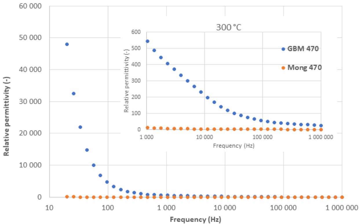
Figure 14. Relative permittivity dependence on frequency at 300 °C for coatings sprayed with SD 470.
