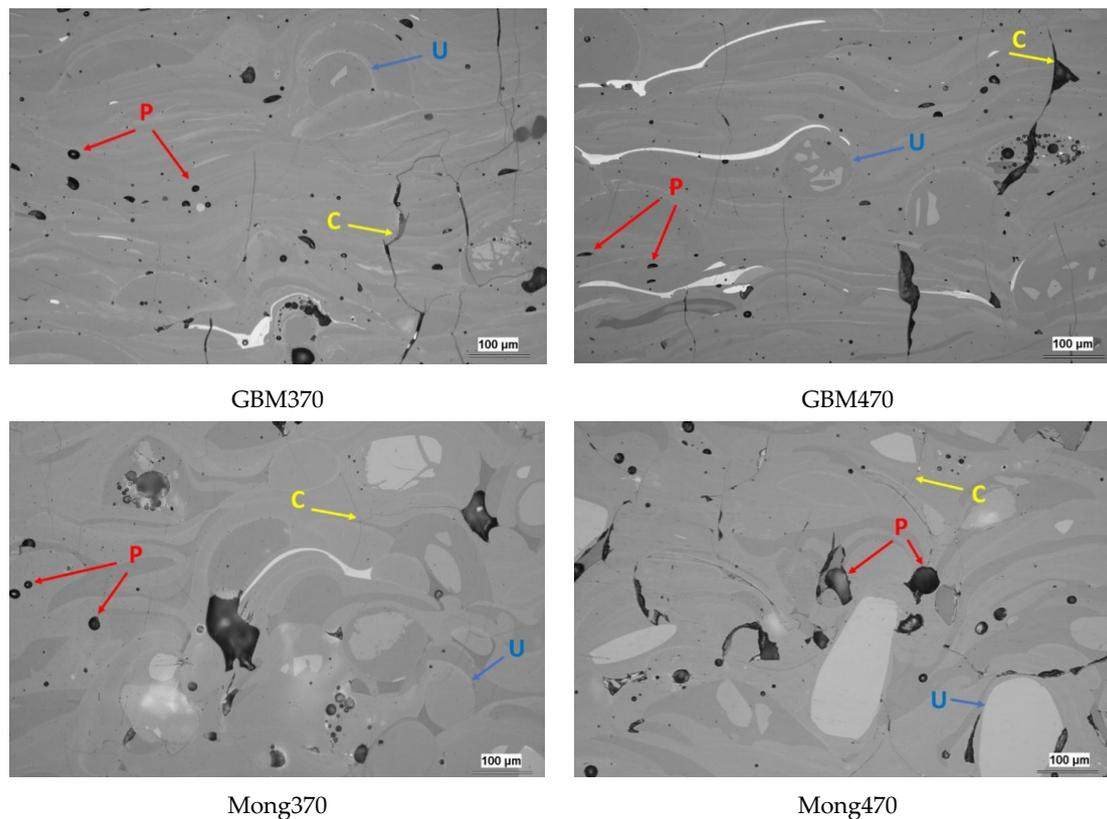
**Figure 2.** Light micrographs on cross sections of coatings. The powders for spraying came from different mines in Mongolia (label Mong) and in the Czech Republic (label GBM). The number indicates spray distance in mm.
