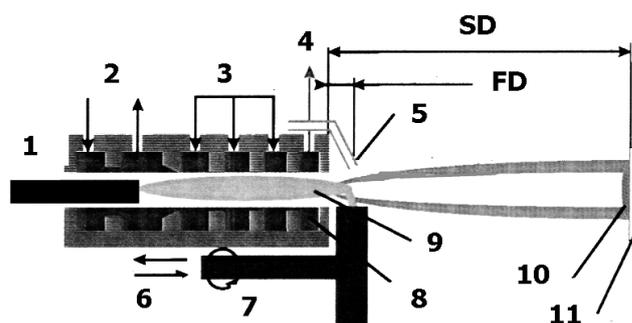
**Figure 1.** WSP plasma spraying. 1—cathode; 2—water in and out for cathode cooling; 3 and 4—water in and out for plasma stabilization; 5—powder feeding tube; 6—water in and out for anode cooling; 7—anode rotation; 8—water vortex; 9—electric arc; 10—coating; 11—substrate; SD—spray distance; FD—feeding distance.
