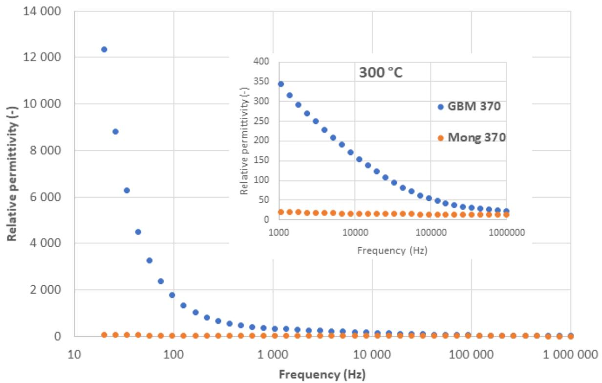
Figure 13. Relative permittivity dependence on frequency at 300 °C for coatings sprayed with SD 370.
