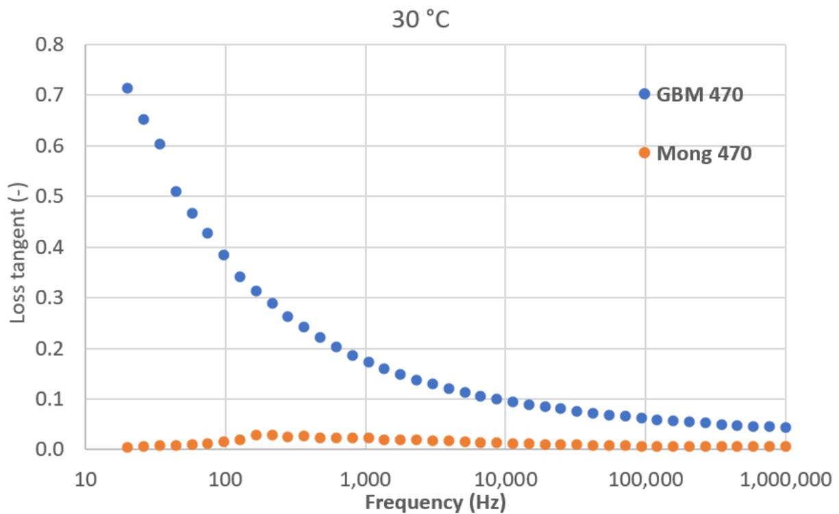
Figure 11. Loss tangent dependence on frequency at room temperature for coatings sprayed with SD 470.
