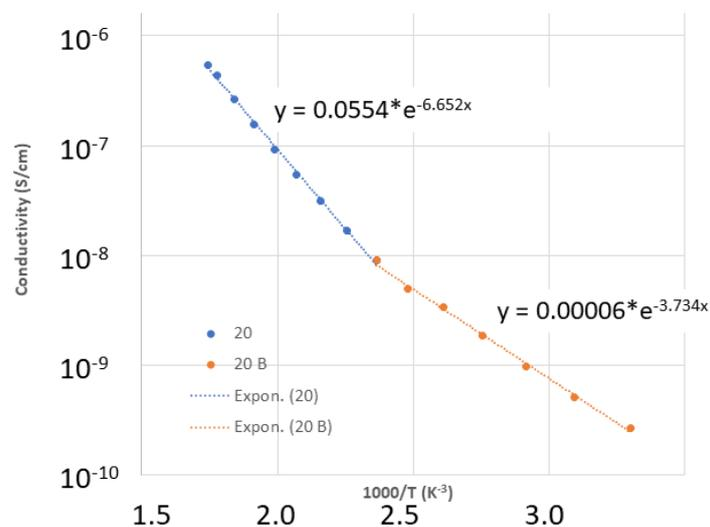
Figure 18. AC conductivity on temperature for the sample GBM 370 at frequency 20 Hz.
