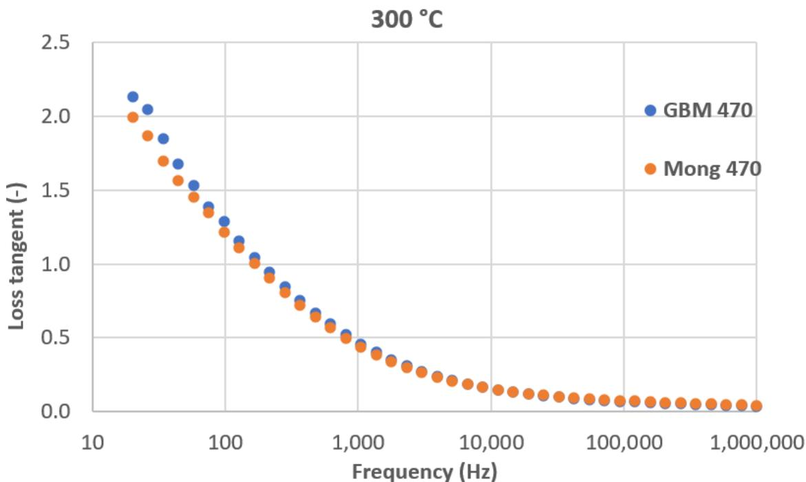
Figure 16. Loss tangent dependence on frequency at 300 °C for coatings sprayed with SD 470.
