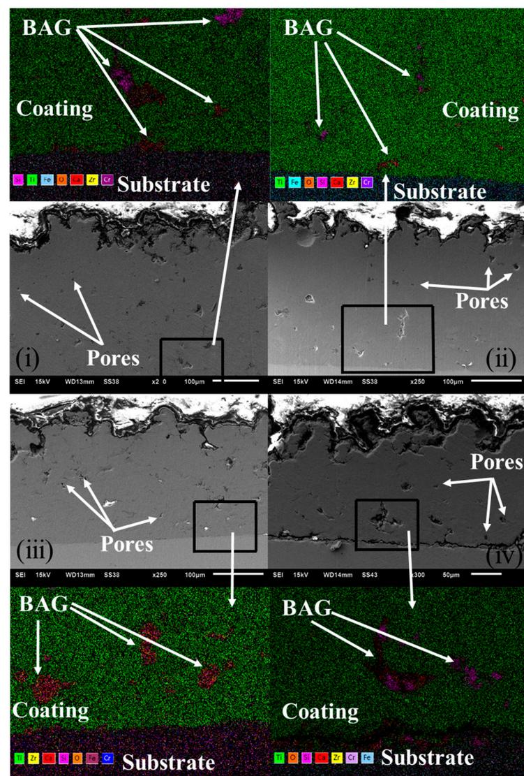
**Figure 2.** High-magnification SEM/EDS cross-sectional images of the laser-treated cold-sprayed deposits on austenitic 316L SS. (i) Ti/10BAG-L; (ii) Ti/15BAG-L; (iii) Ti/20BAG-L; (iv) Ti/25BAG-L.
