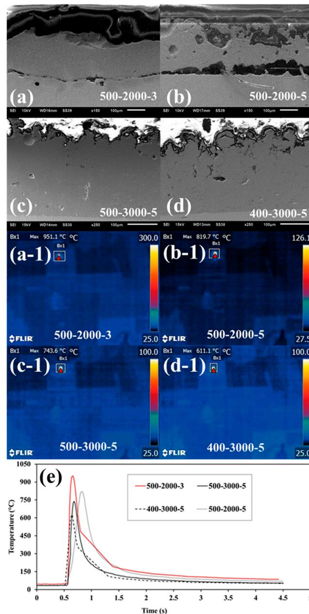
**Figure 1.** Experimentally measured maximum temperature results of laser-treated cold-sprayed Ti/15BAG composite coating along with SEM images at different laser parameters (a,a-1) 500-2000-3 (b,b-1) 500-2000-5 (c,c-1) 500-3000-5 (d,d-1) 400-3000-5 and (e) temperature distribution profile.
