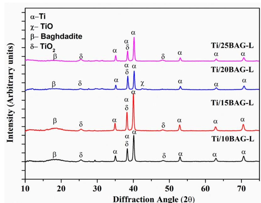
**Figure 4.** Phase assessment of the laser-treated cold-spray bio composite deposited on austenitic 316L SS.
