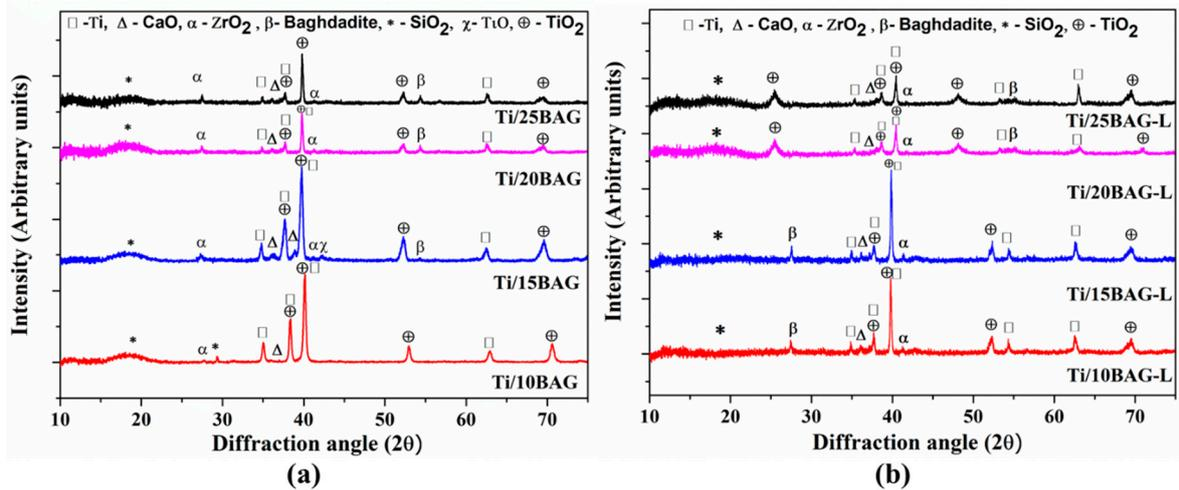
Figure 6. Phase identification of corroded cold-sprayed coatings (a) before laser treatment; (b) after laser treatment.
