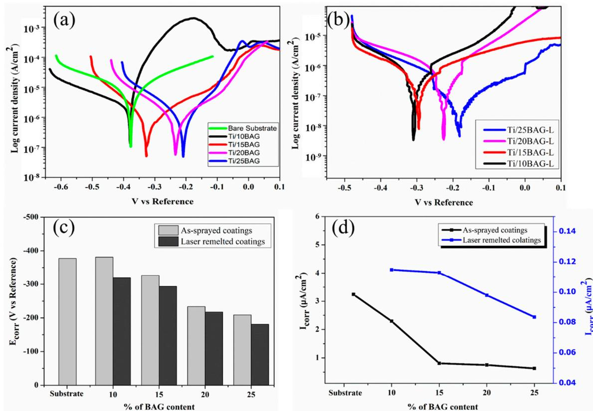
Figure 5. Potentiodynamic scans of (a) as-sprayed (b) laser-treated cold-spray deposits on biomedical steel in Ringer’s solution: (c)  $E_{corr}$  and (d)  $i_{corr}$ .
