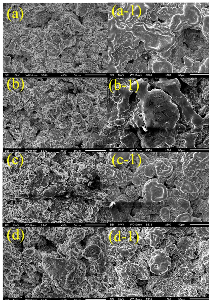
**Figure 3.** Surface SEM/EDS images of the cold-spray deposits on biomedical steel. (a) Ti/10BAG, (b) Ti/15BAG, (c) Ti/20BAG, (d) Ti/25BAG; and laser-treated coatings (a-1) Ti/10BAG-L, (b-1) Ti/15BAG-L, (c-1) Ti/20BAG-L, (d-1) Ti/25BAG-L.
